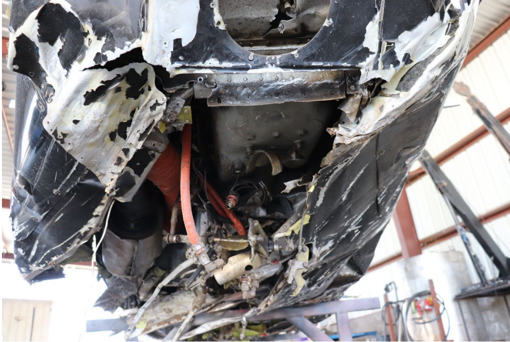
Figure 8: View of oil sump damage (photo courtesy of the NTSB)
