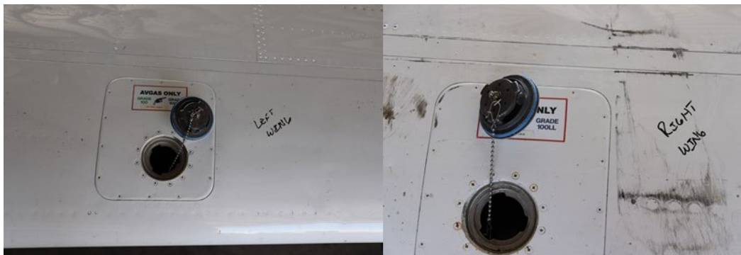
Figure 2: View of airplane left and right fuel caps (photo courtesy of the NTSB)
