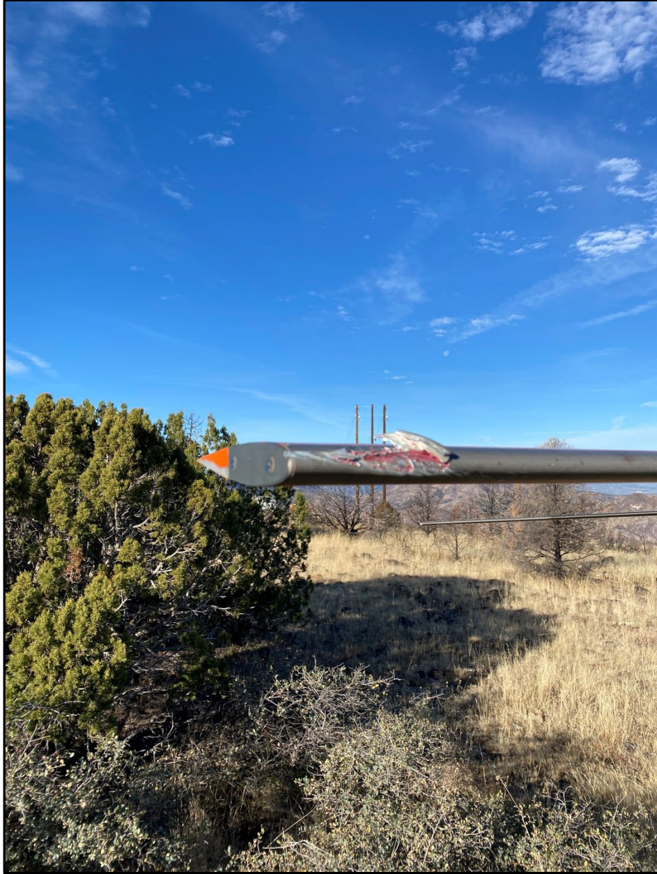
Figure 2: Helicopter main rotor blade damage as viewed from outboard leading edge.
