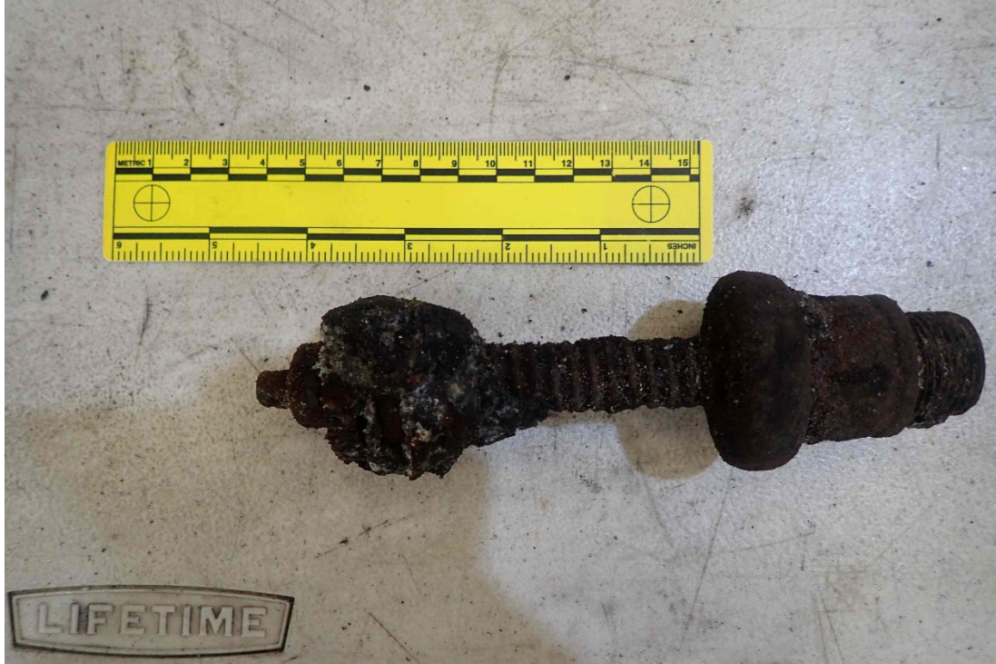
Figure 8 - Flap actuator jackscrew
