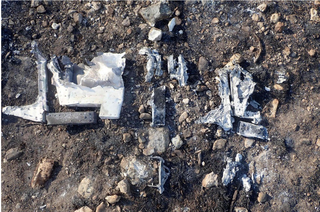
Figure 9 - Tail section balance weights and hinges
