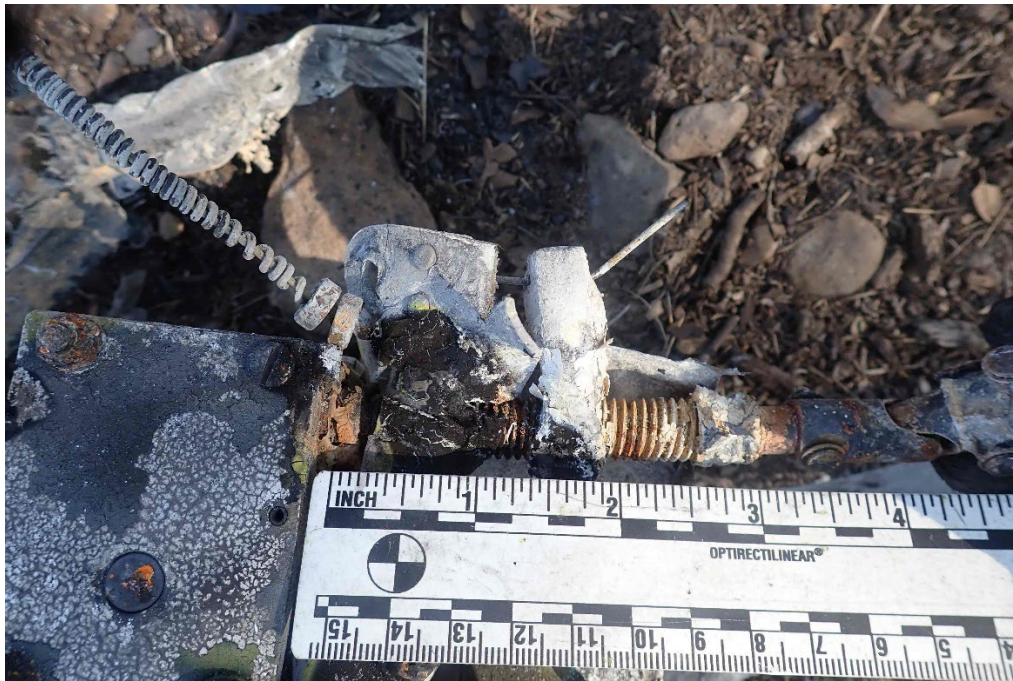
Figure 11 - Cabin pitch trim assembly
