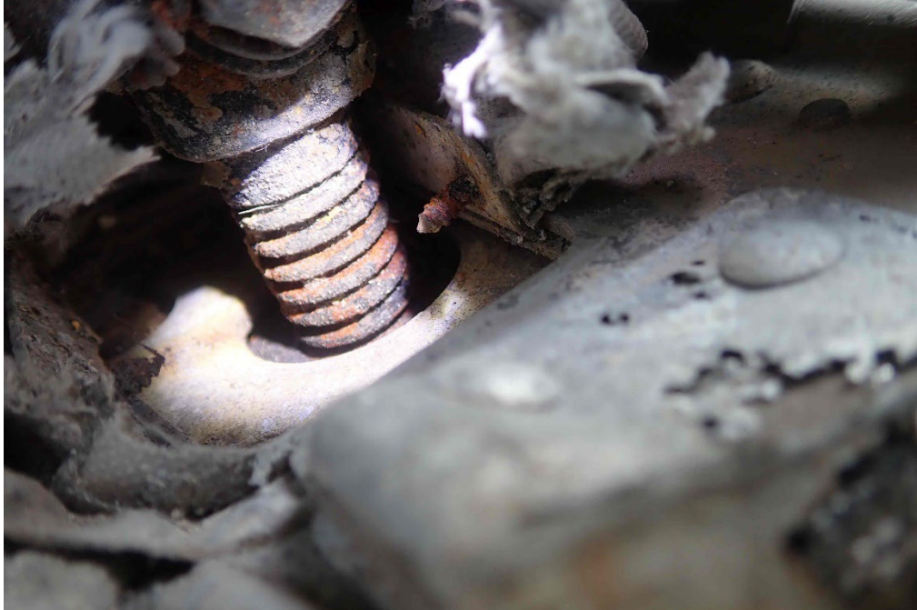
Figure 10 - Moving tail aft assembly jack screw threads
