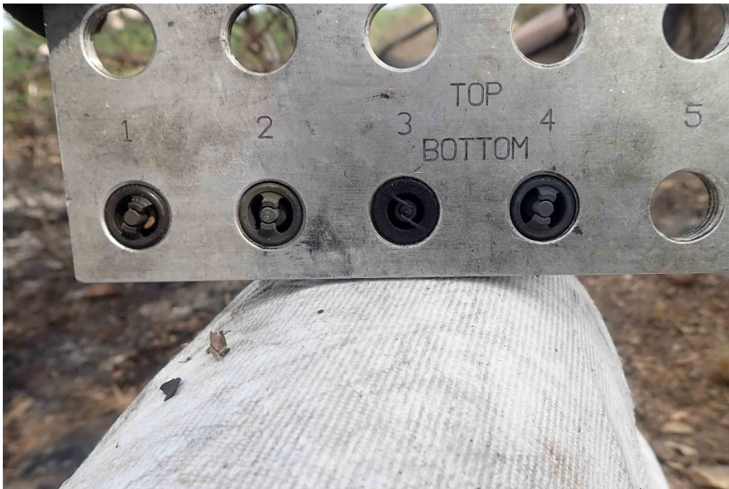
Figure 10 - Bottom spark plugs at accident the site
