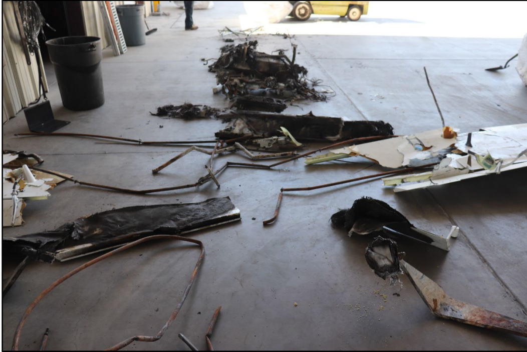
Figure 1: View of flight control torque tubes.
