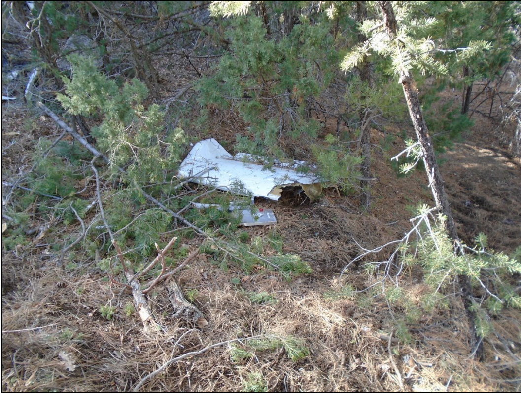
Figure 4: View of right wing fragment (photo courtesy of the NTSB)
