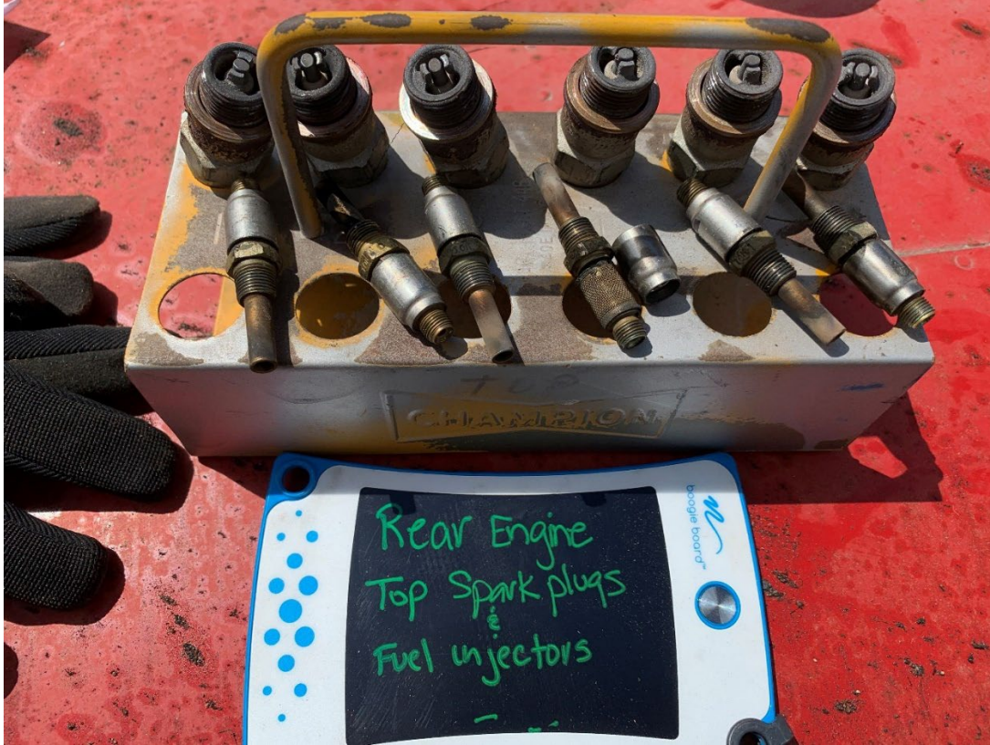
Figure 23 - View of Rear Engine Top Spark Plugs and Fuel Injectors
