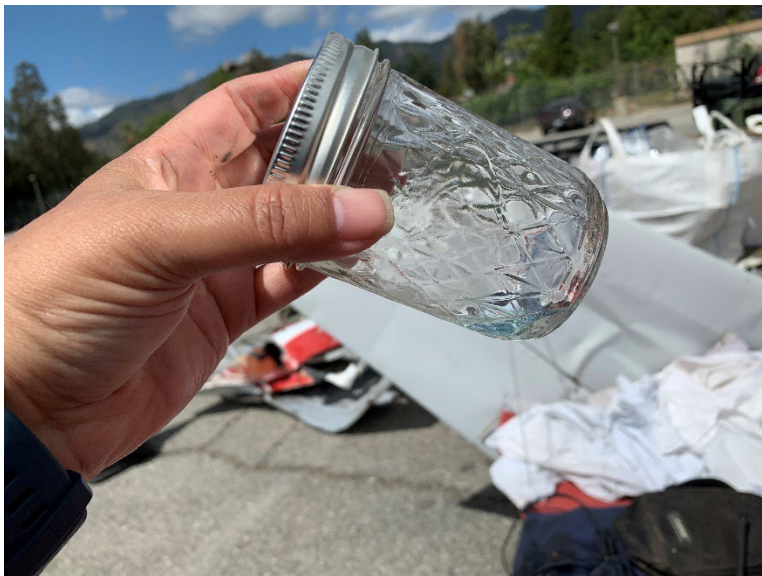
Figure 25 - Residual Fuel from Fuel Pump
