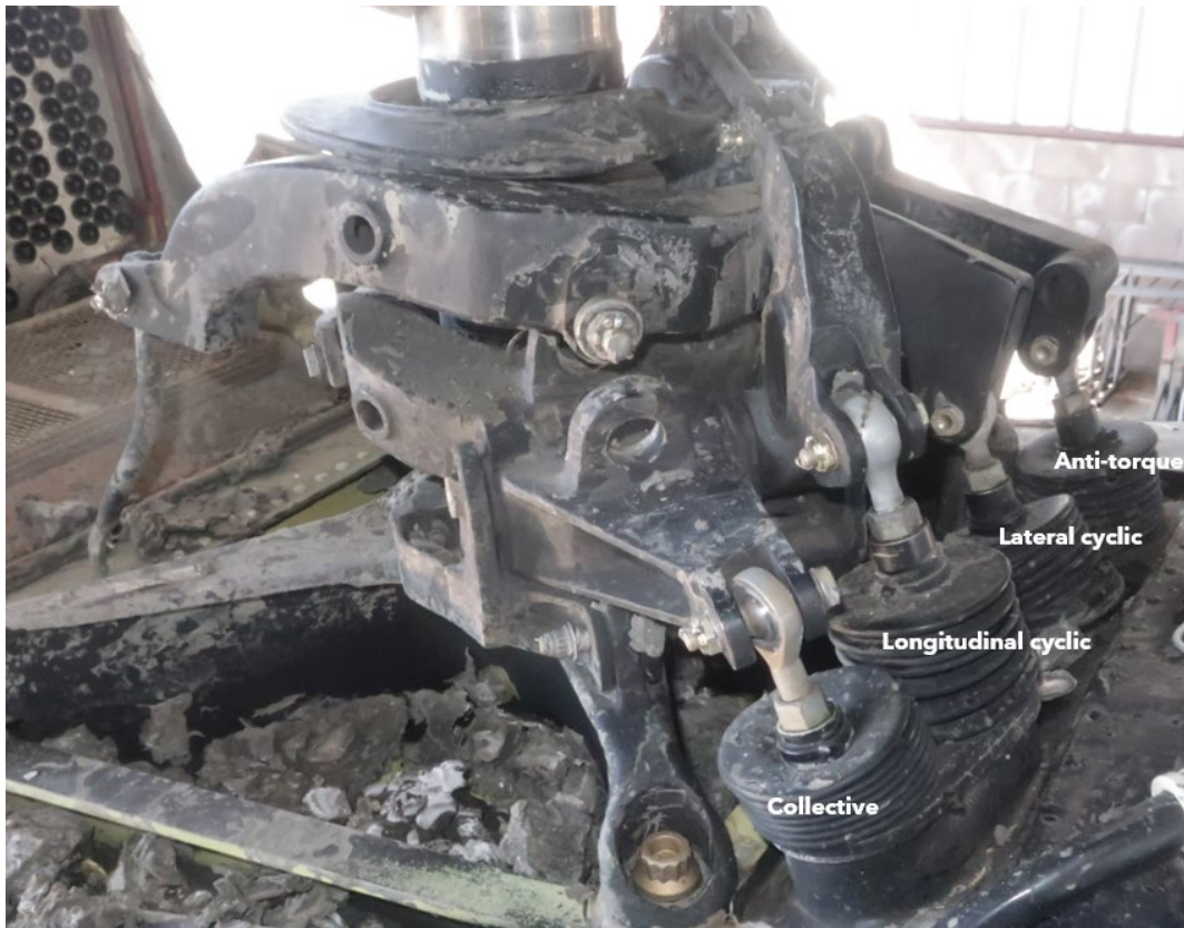
Figure 4. Photo of the upper control connections.
