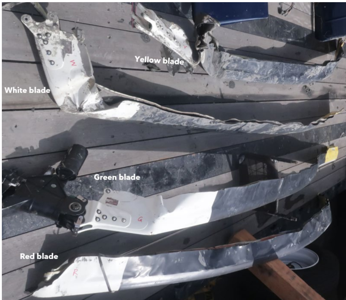
Figure 6. Rotor blades and horizontal stabilizer laid out. The blue blade remained connected to the main rotor hub.
