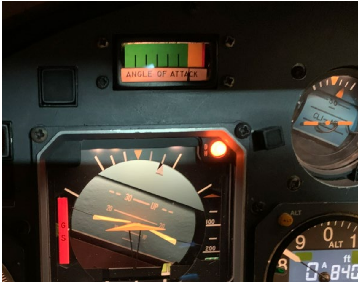
Figure 11: Photo of Lear 35A AOA gauge. 36
