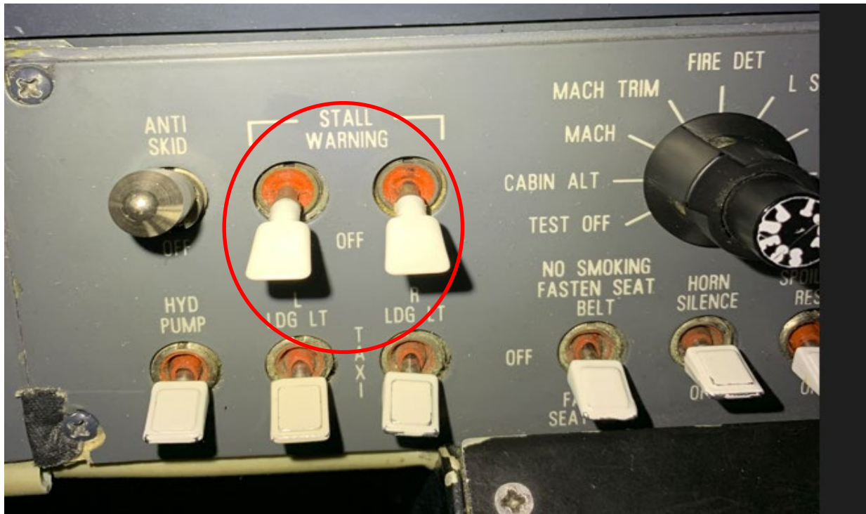
Figure 10: Source: NTSB Photo. Lear 35A Stall Warning Switches on Captains side forward instrument panel, indicated by red circle. 34 Picture taken inside an exemplar Lear 35.
