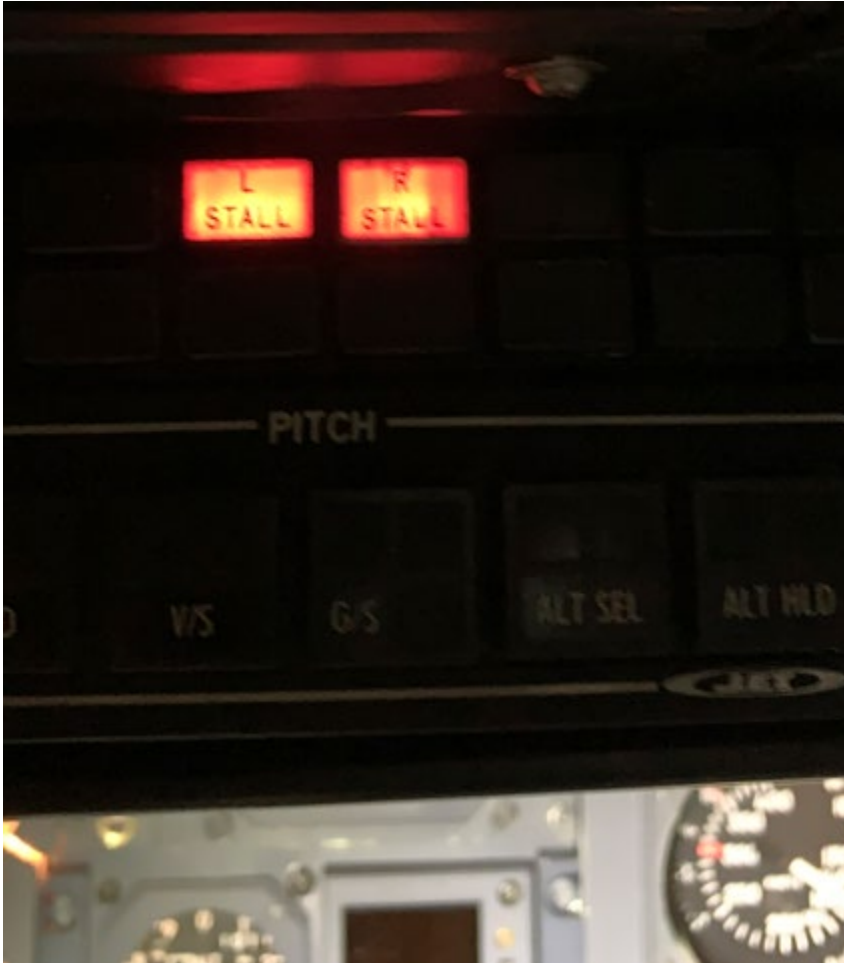
Figure 12: Photo of Lear 35A stall warning lights. 37
