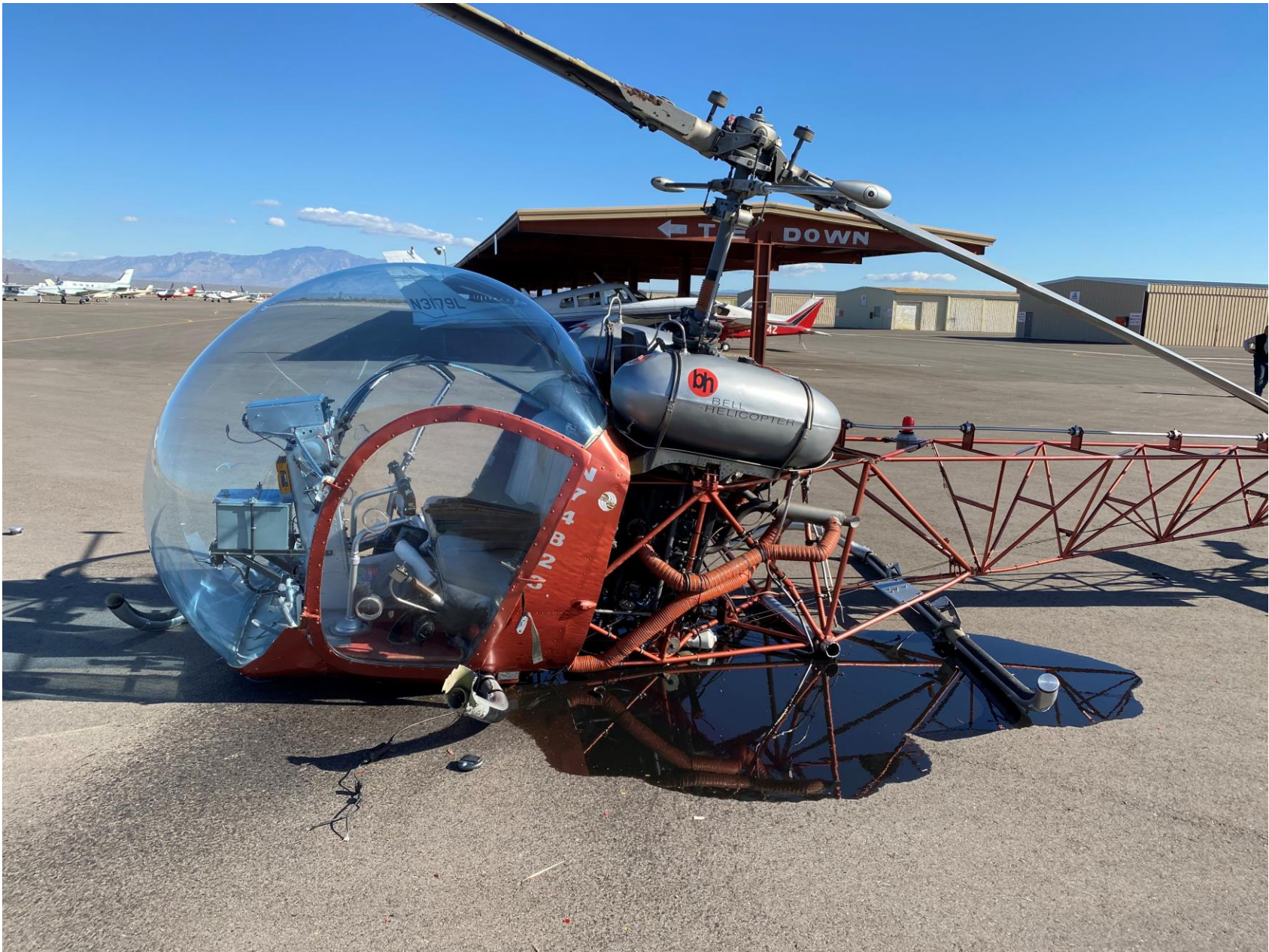
Photo 1 – Damage to cross tubes in tail boom
