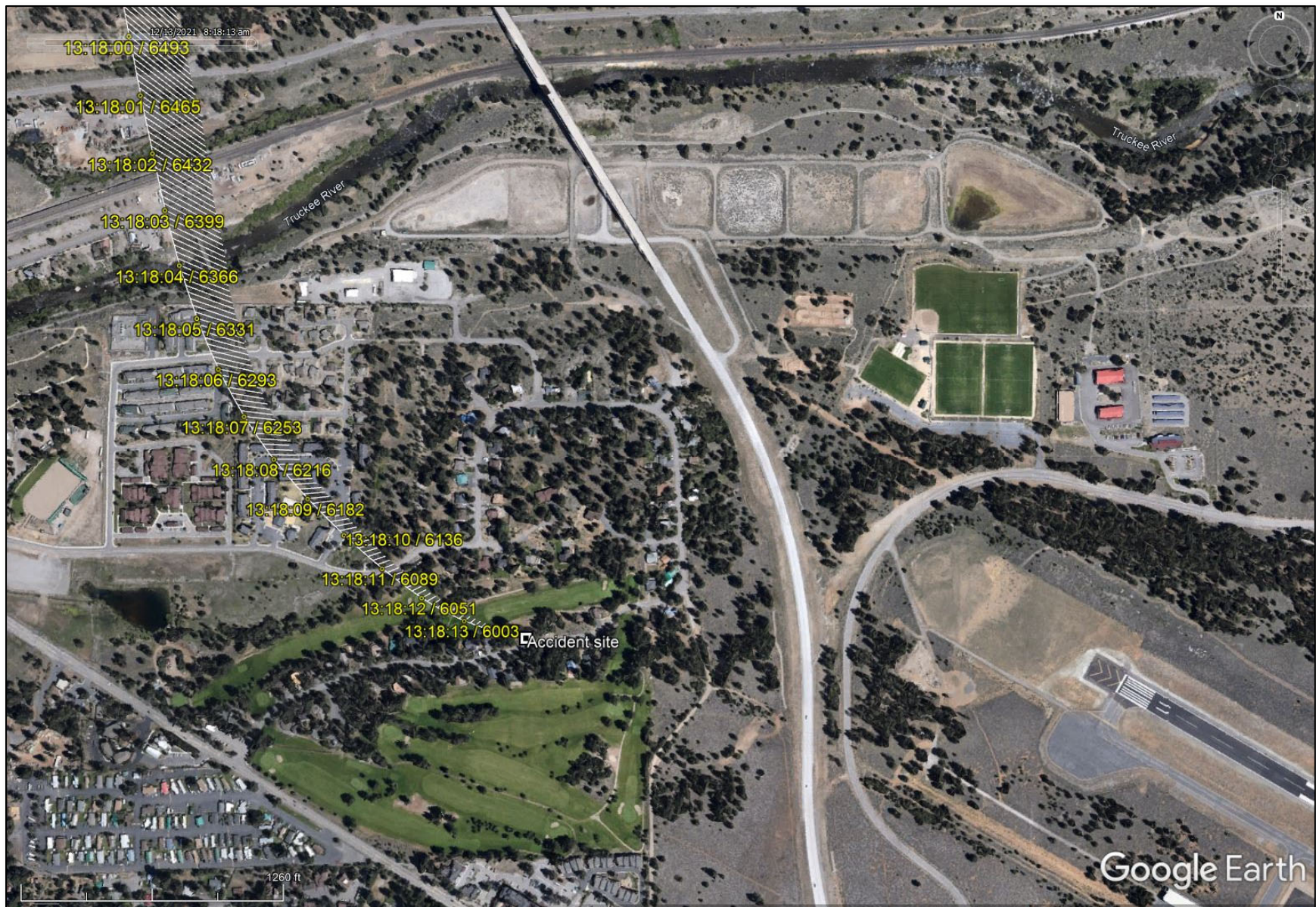
Figure 7. Final segment of N605TR's flight path and the accident site depicted over a Google Earth satellite image. Labels along the flight path indicate ADS-B time in PDT and altitude in feet MSL.
