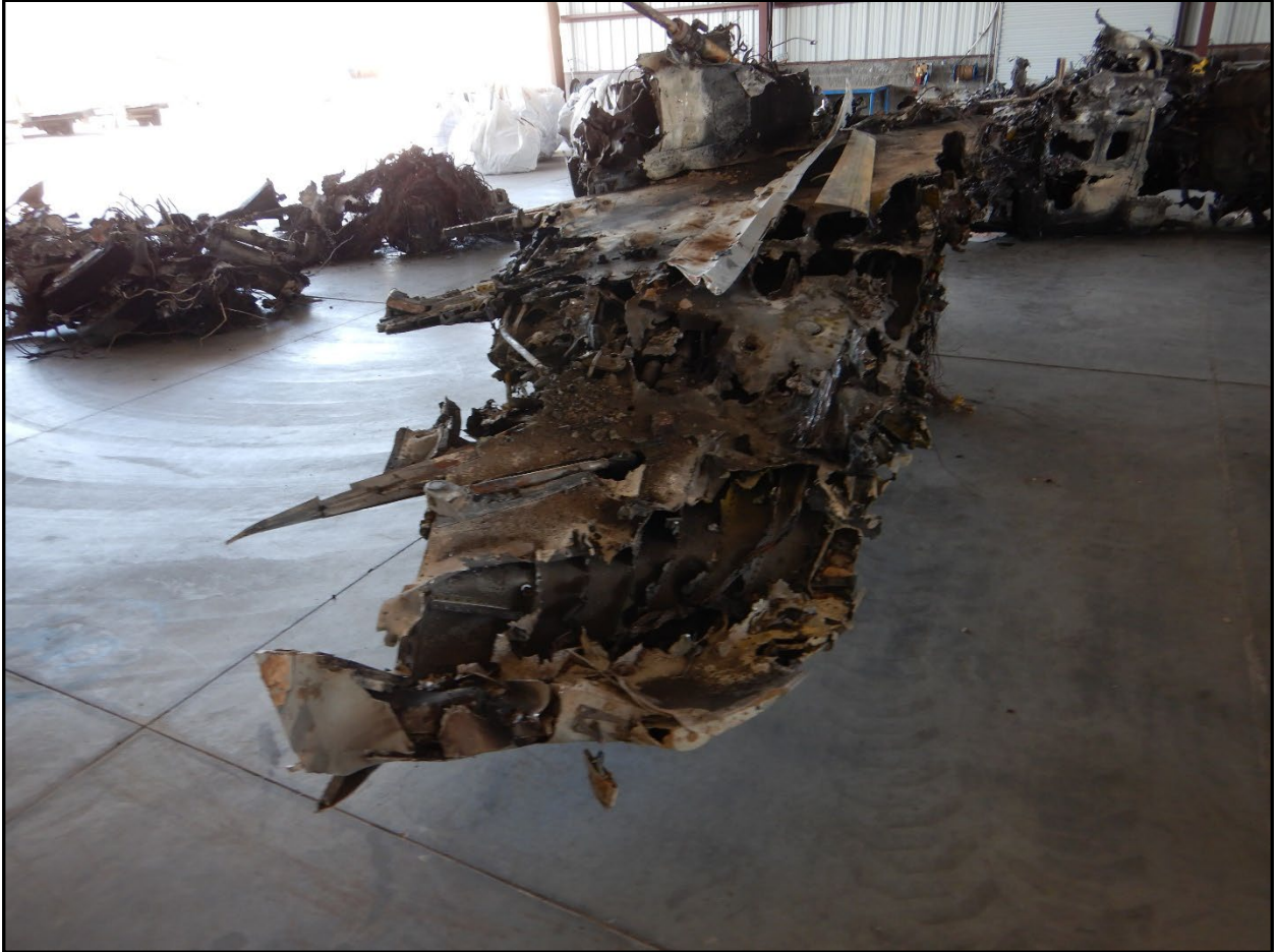
Figure 3: Picture of wing showing the extent of thermal and impact damage sustained.
