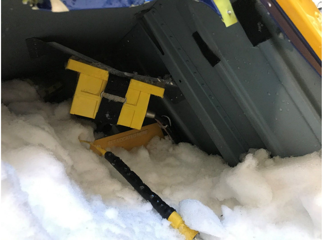
Figure 7. The ELT and portable antenna, as found in the right baggage compartment.
