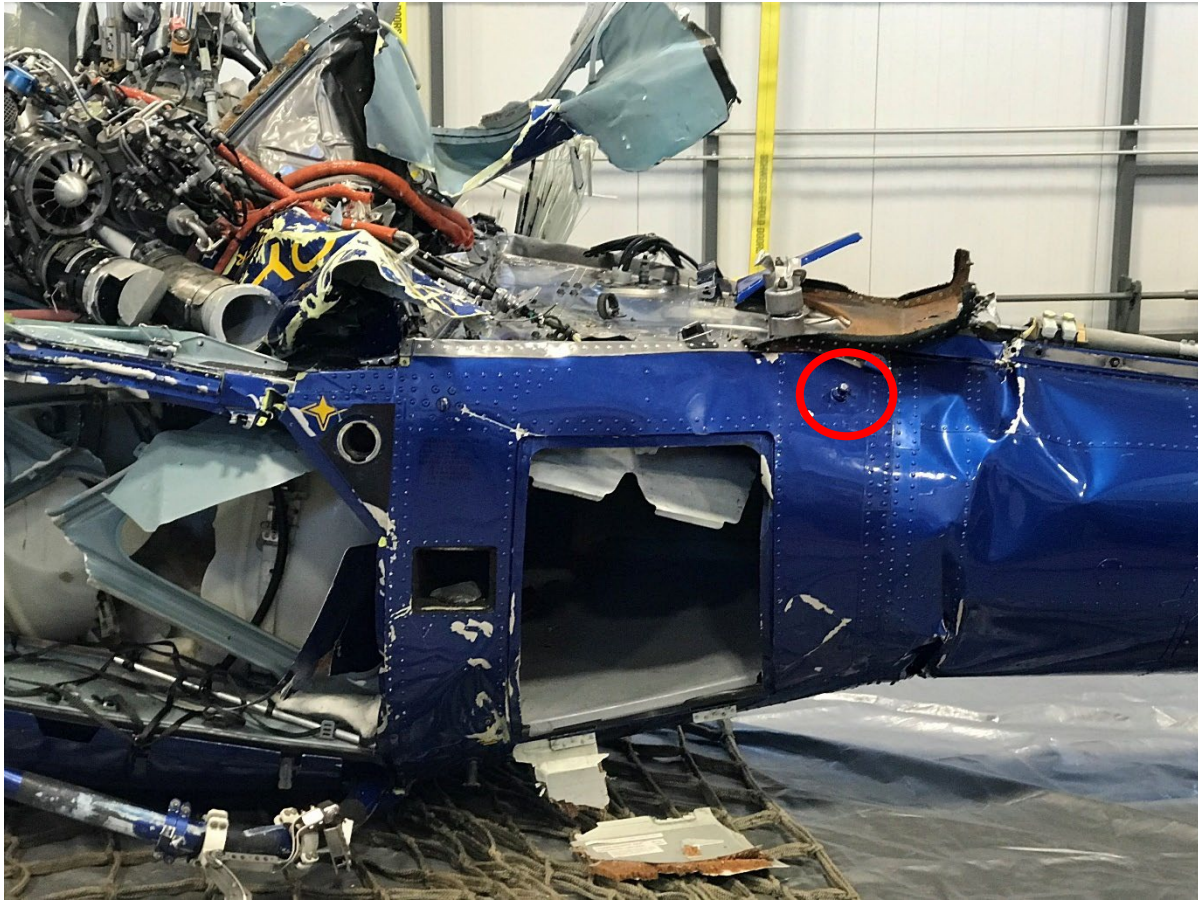
Figure 8. The ELT antenna mount on the upper left side of the tailboom.
