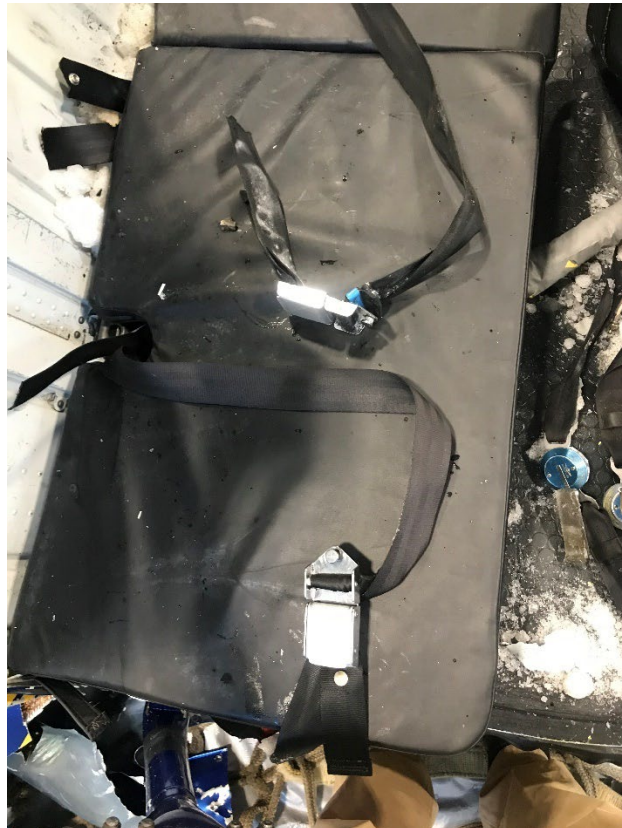
Figure 6. The lap belts for aft passenger seats #3 and #4. The upper buckle belongs to the restraint system for aft passenger seat #2.
