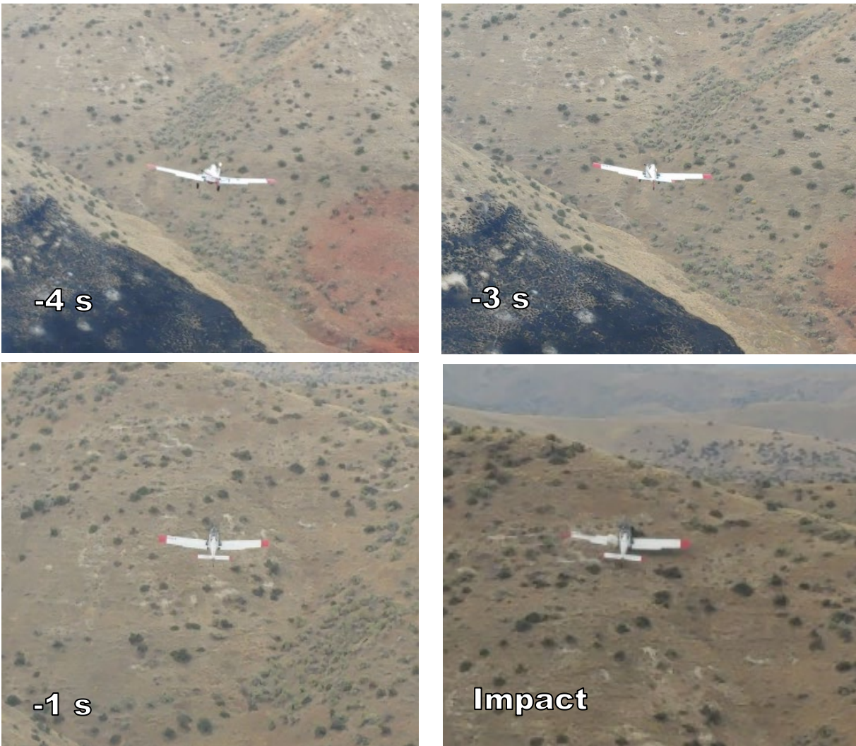
Figure 6. Frames from accident video showing transition from descending ( - 4s to impact) to climbing ( - 3s to impact) to impact with terrain.
