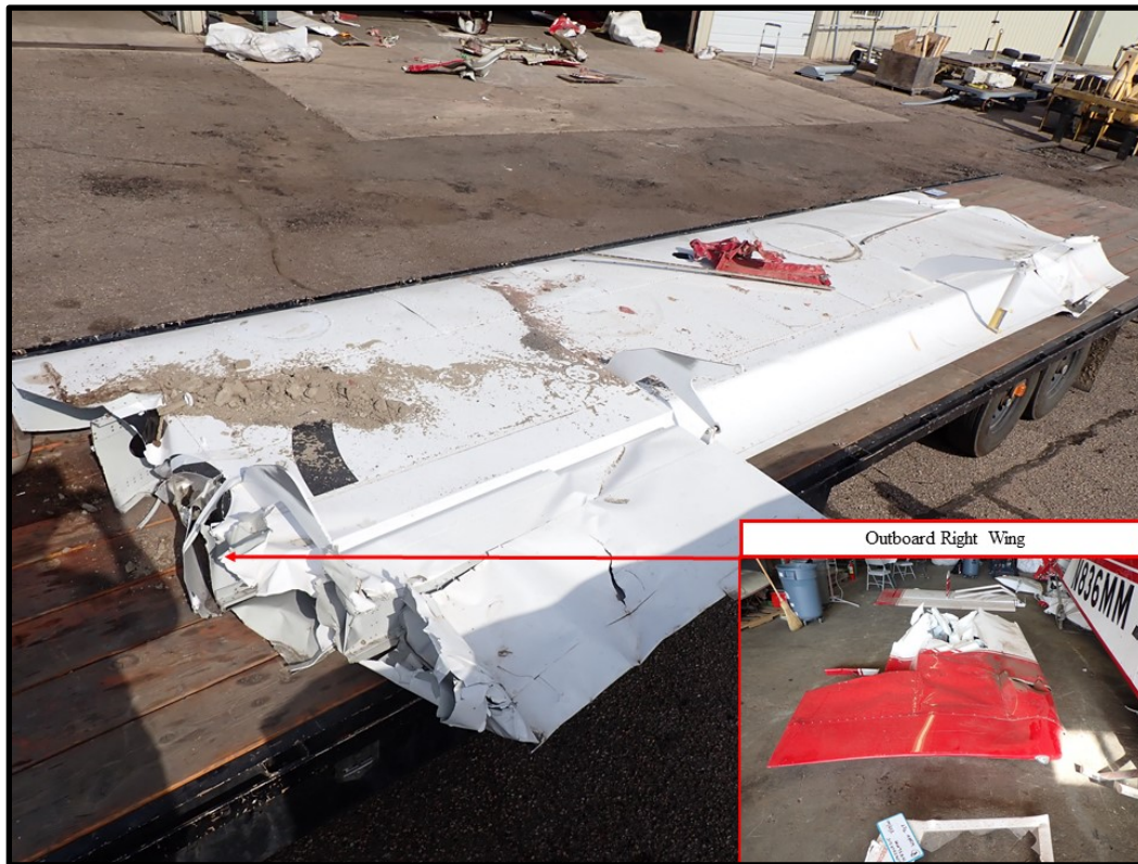
Figure 5: View of ring wing damage.
