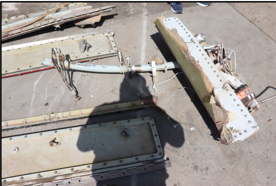
Figure 10: View of aft fire gate bulkhead.
