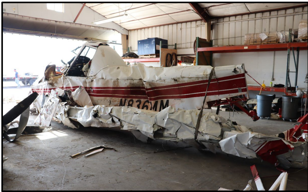
Figure 4: View of left wing damage.
