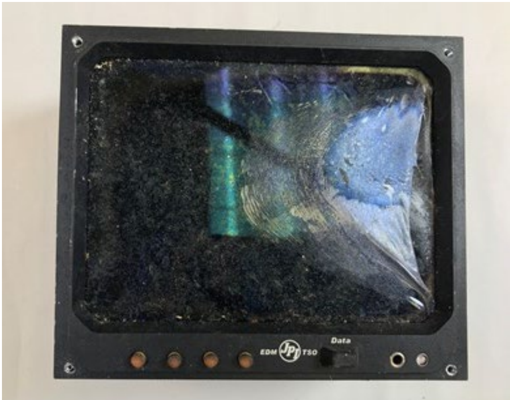
Figure 1. Damage to JPI EDM 930.
