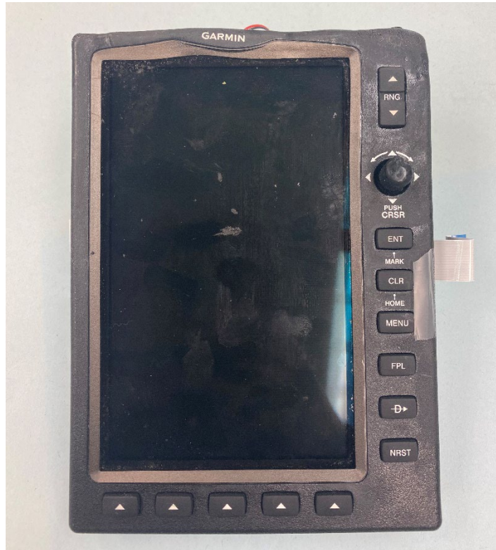
Figure 3. Damage to Garmin GPSMAP 695.
