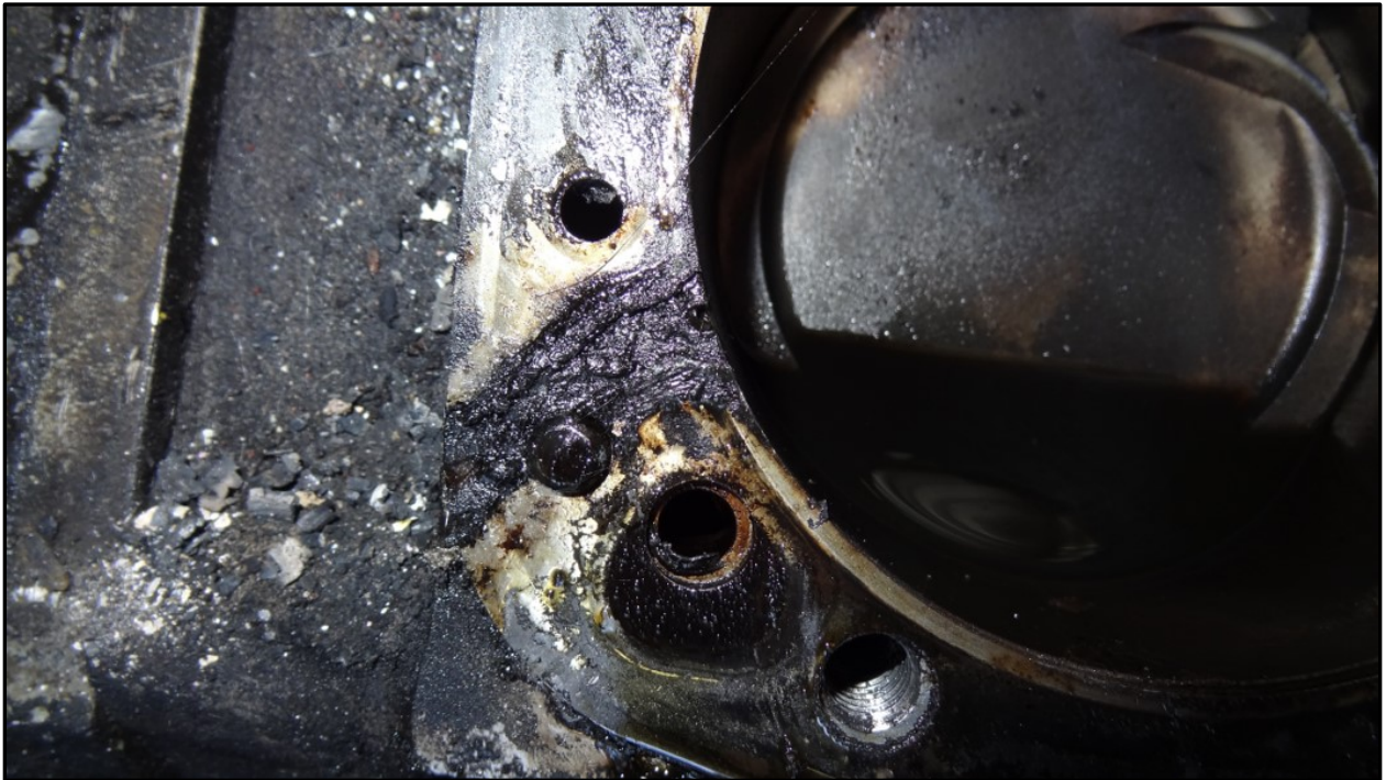
Figure 3: No. 1 cylinder metal deformation.
