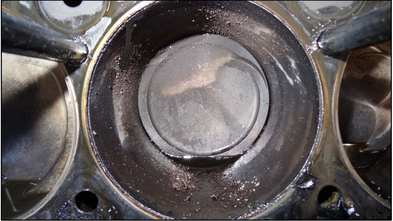
Figure 2: No. 2 cylinder internal damage.
