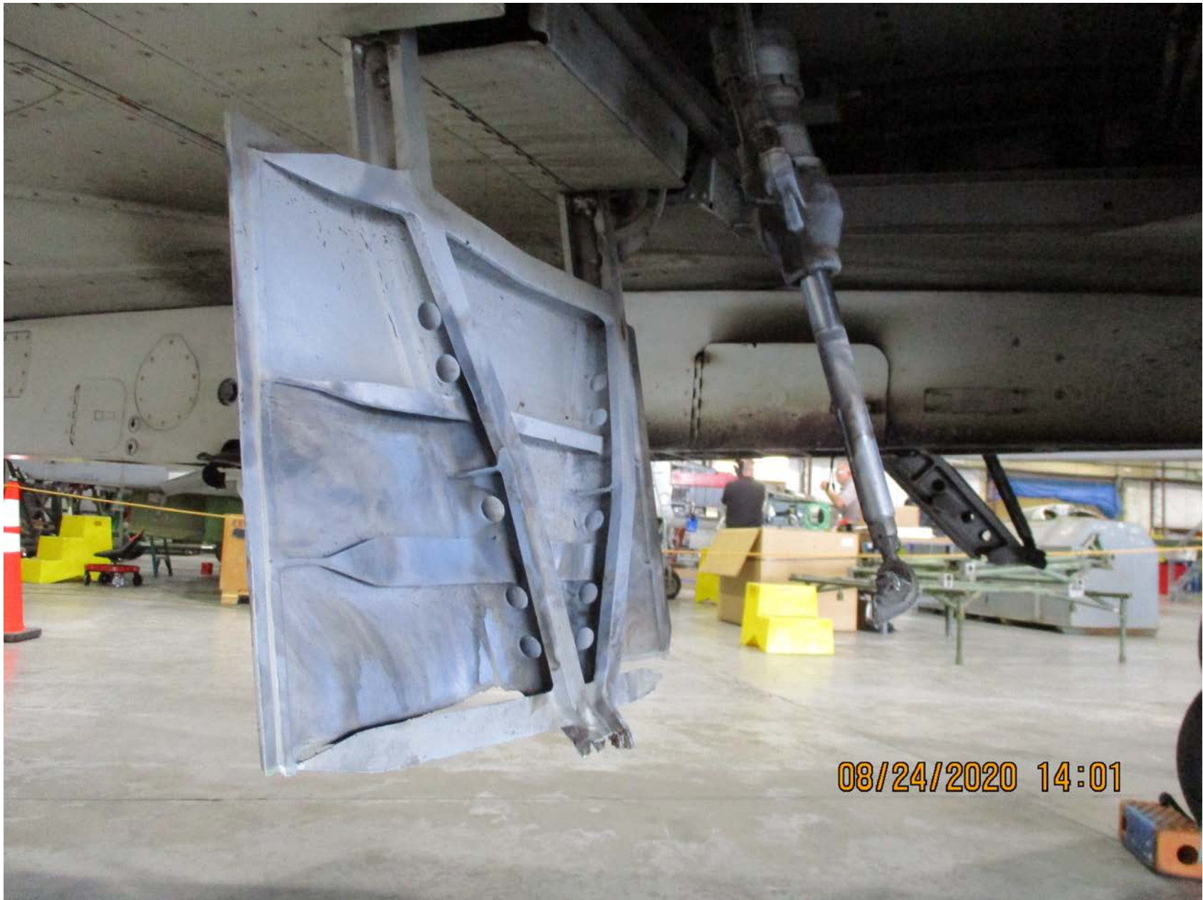
Photo 2 - View of left speed brake damage (photo courtesy of Owner)
