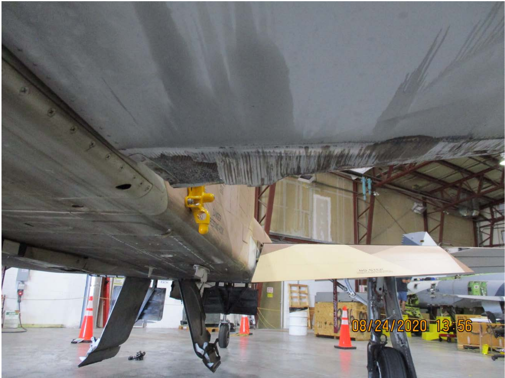
Photo 1 – View of right stabilizer damage (photo courtesy of Owner)
