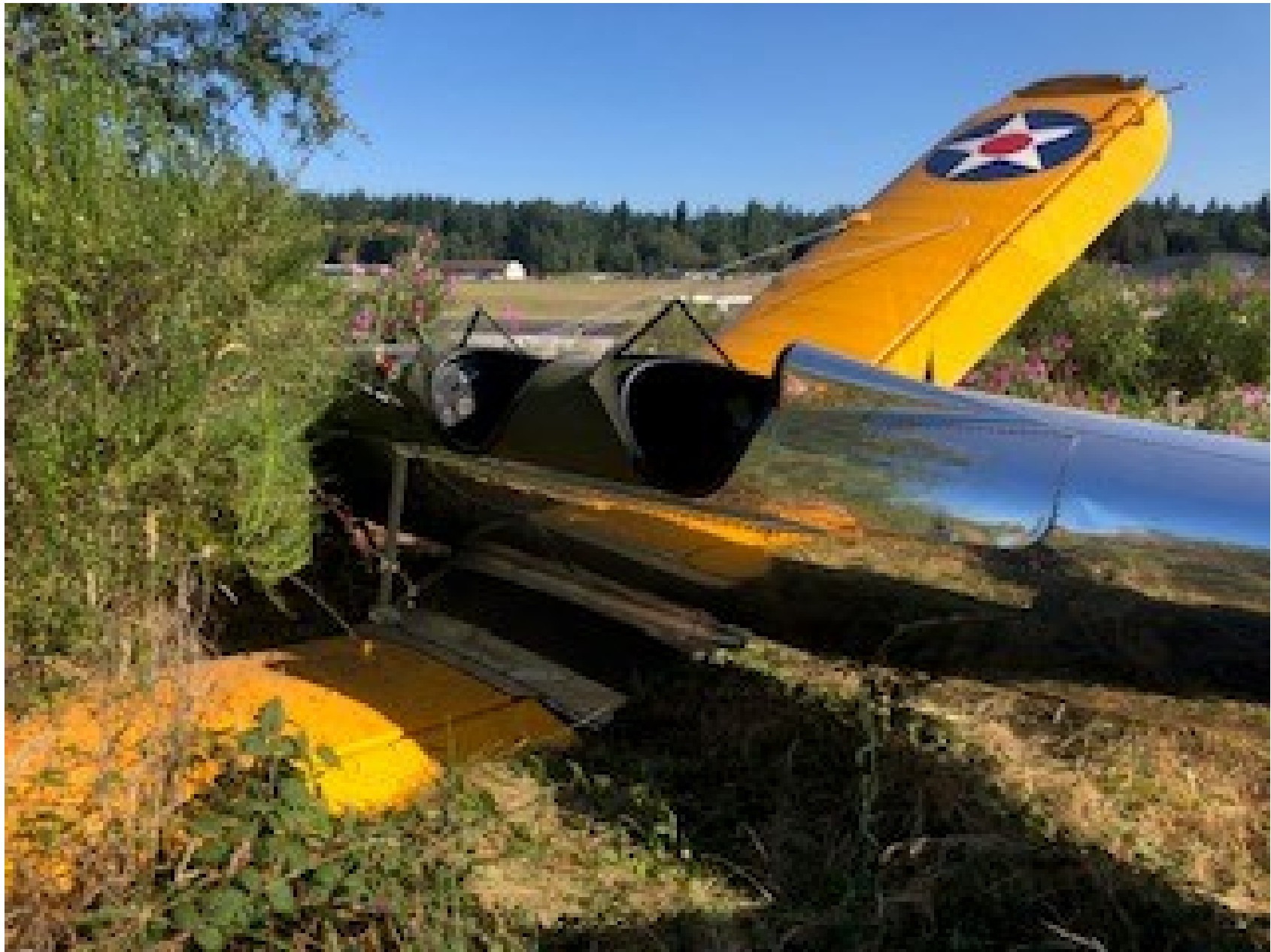
Photo 1 – View of left wing spar damage (photo courtesy of Pilot)
