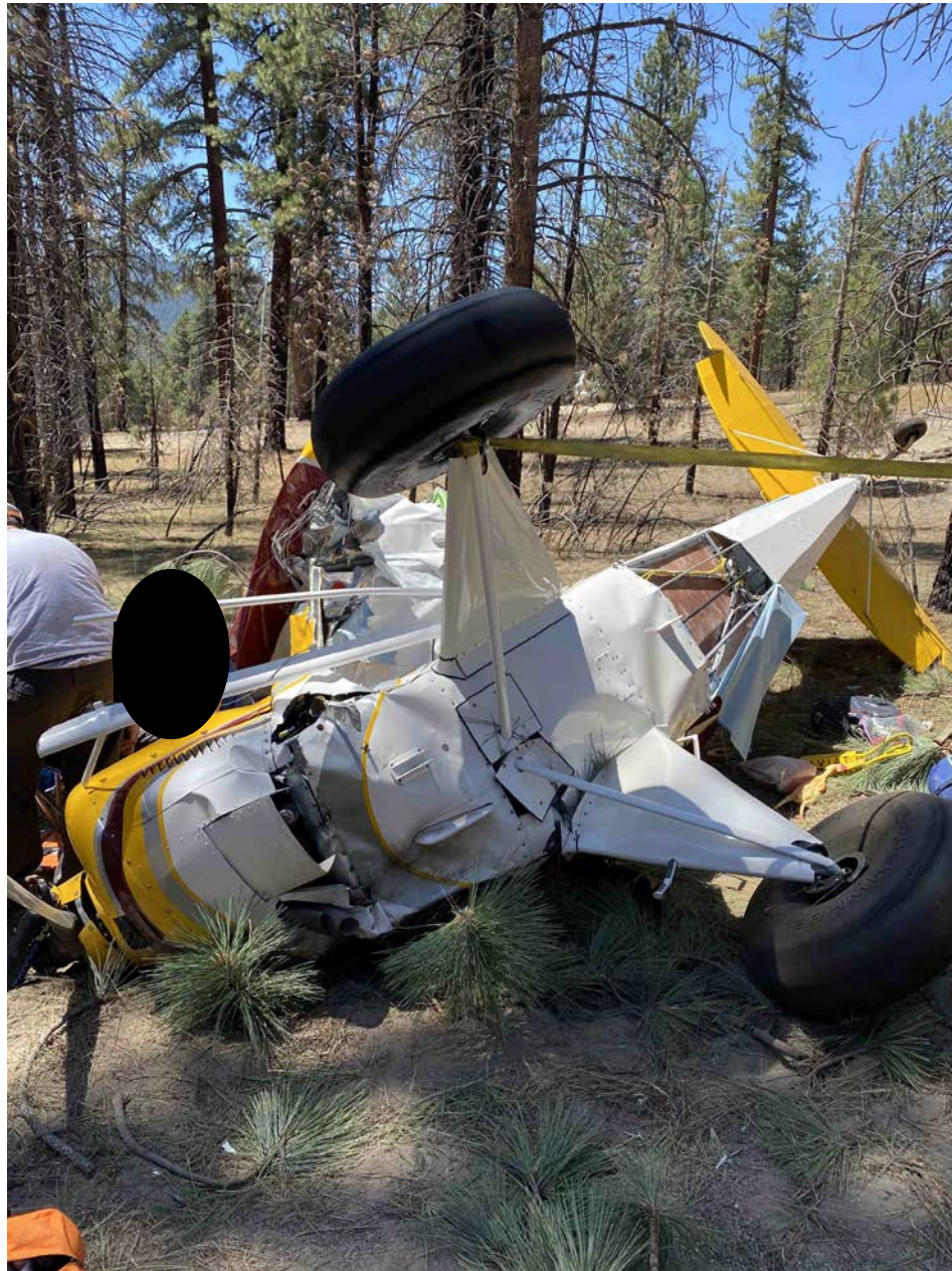
Photo 1 – View of wing and Fuselage damage (photo courtesy of unknown)
