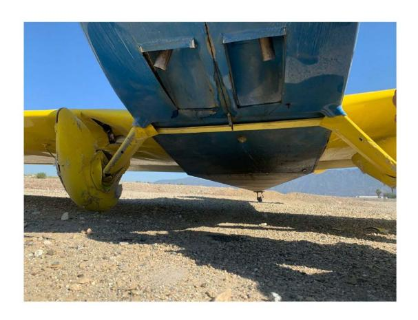
Photo 1: Underside view of airplane. Note damage to the right wing (Airport Ops)
