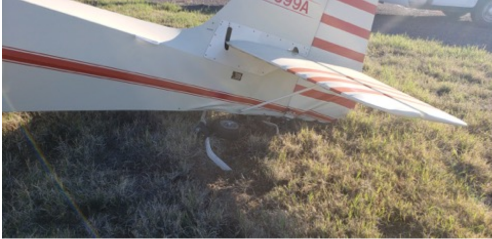
Photo 1: View of wrinkled Rudder (GYR Airport Ops)
