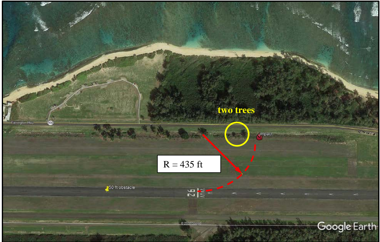
Figure 16: Steady, Coordinated Turn from End of Runway (two trees) until Final Impact (Note: this is the turn radius and not necessarily the actual ground track.)
