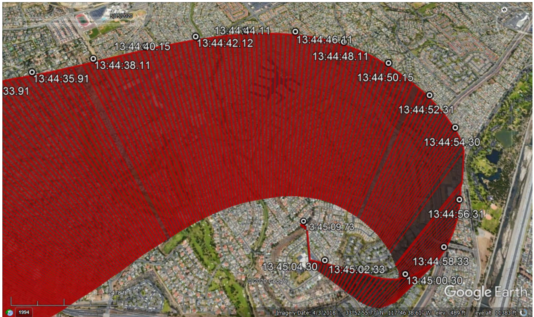
Figure 7. Google Earth overlay of the end of the accident flight recorded on the Appareo Stratus 2S.
