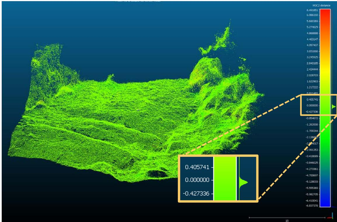
**Figure 6 - Results of M3C2 point cloud comparison**
