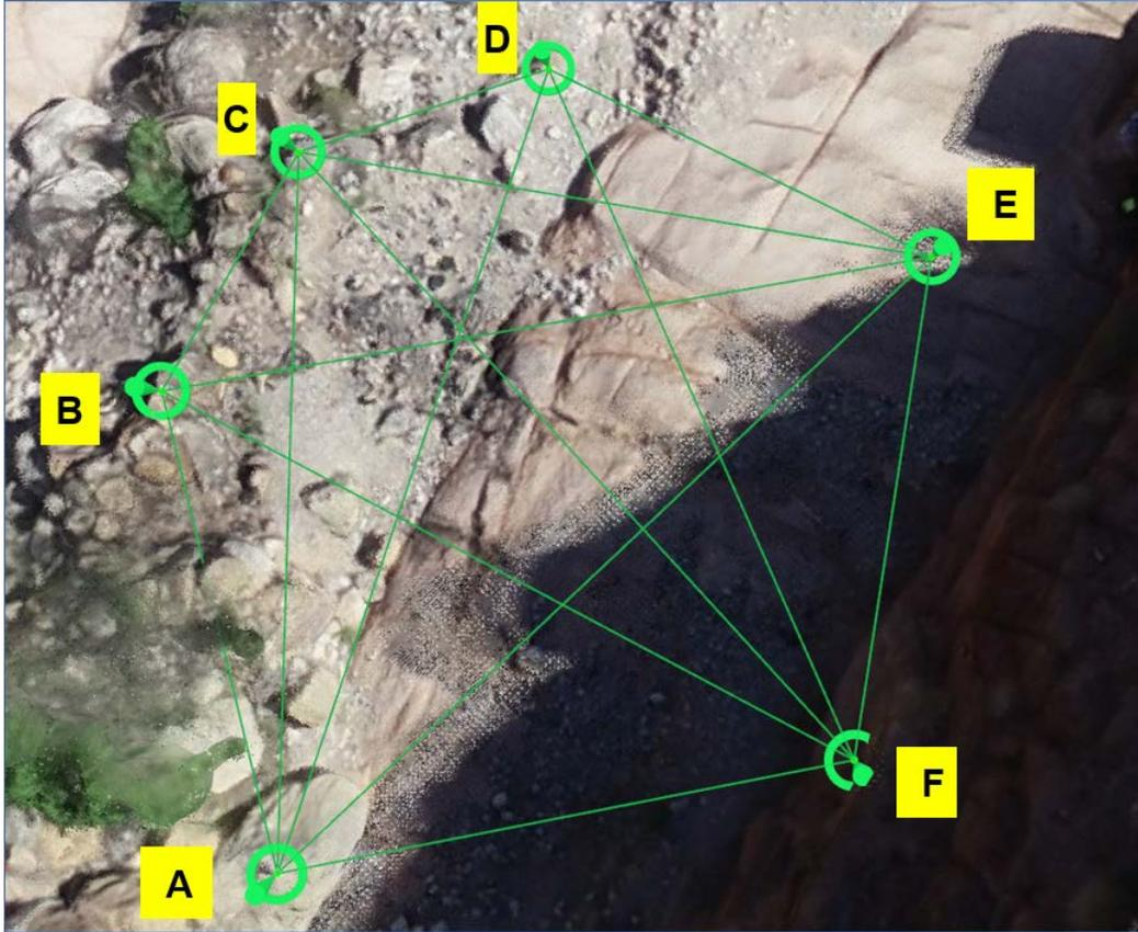
Figure 7 - Location of laser reference spheres used in distance comparison
