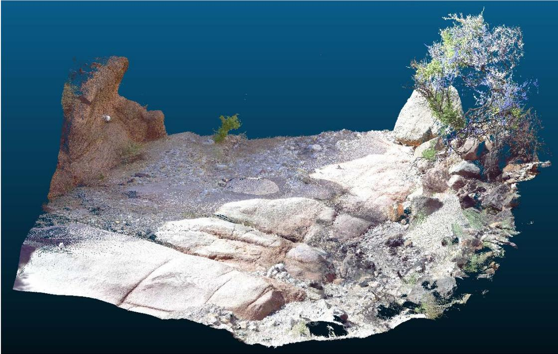
Figure 4 - Screenshot image of FARO laser scanned point cloud
