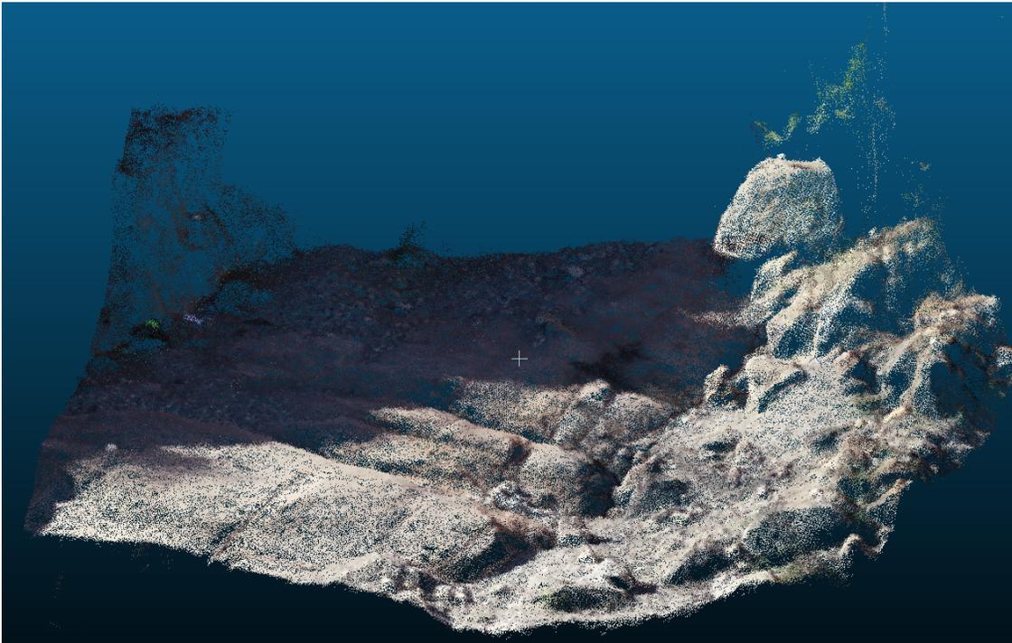
Figure 5 - Screenshot image of UAS point cloud from low altitude flight
