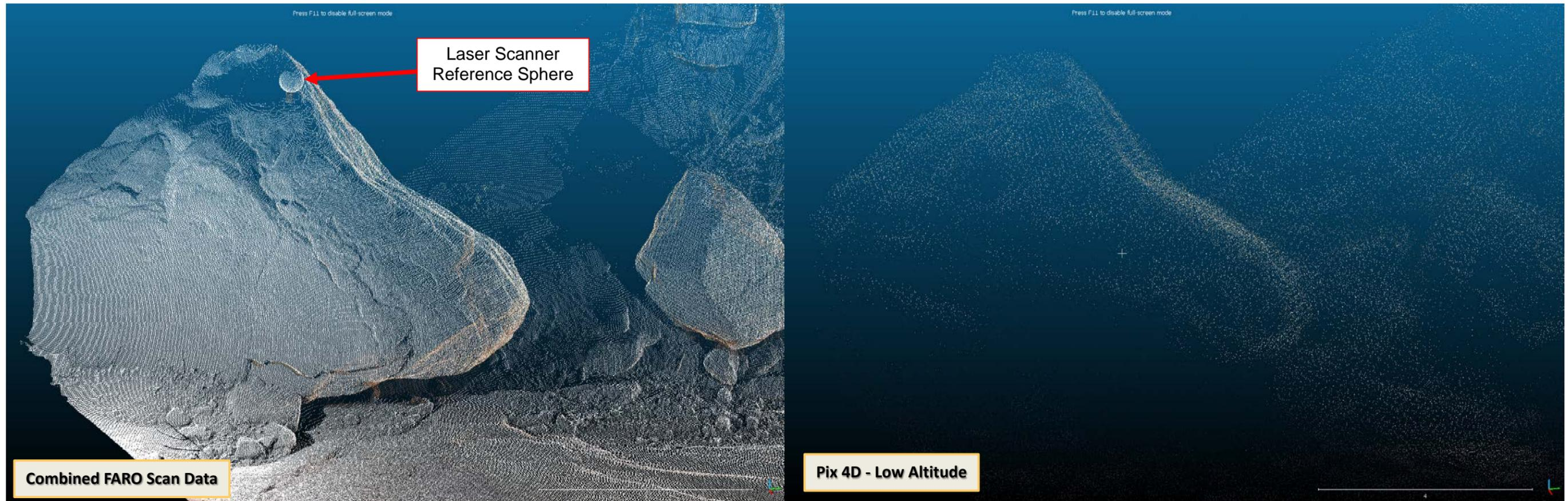
Figure 14 - Side by Side comparison of FARO and UAS point clouds
