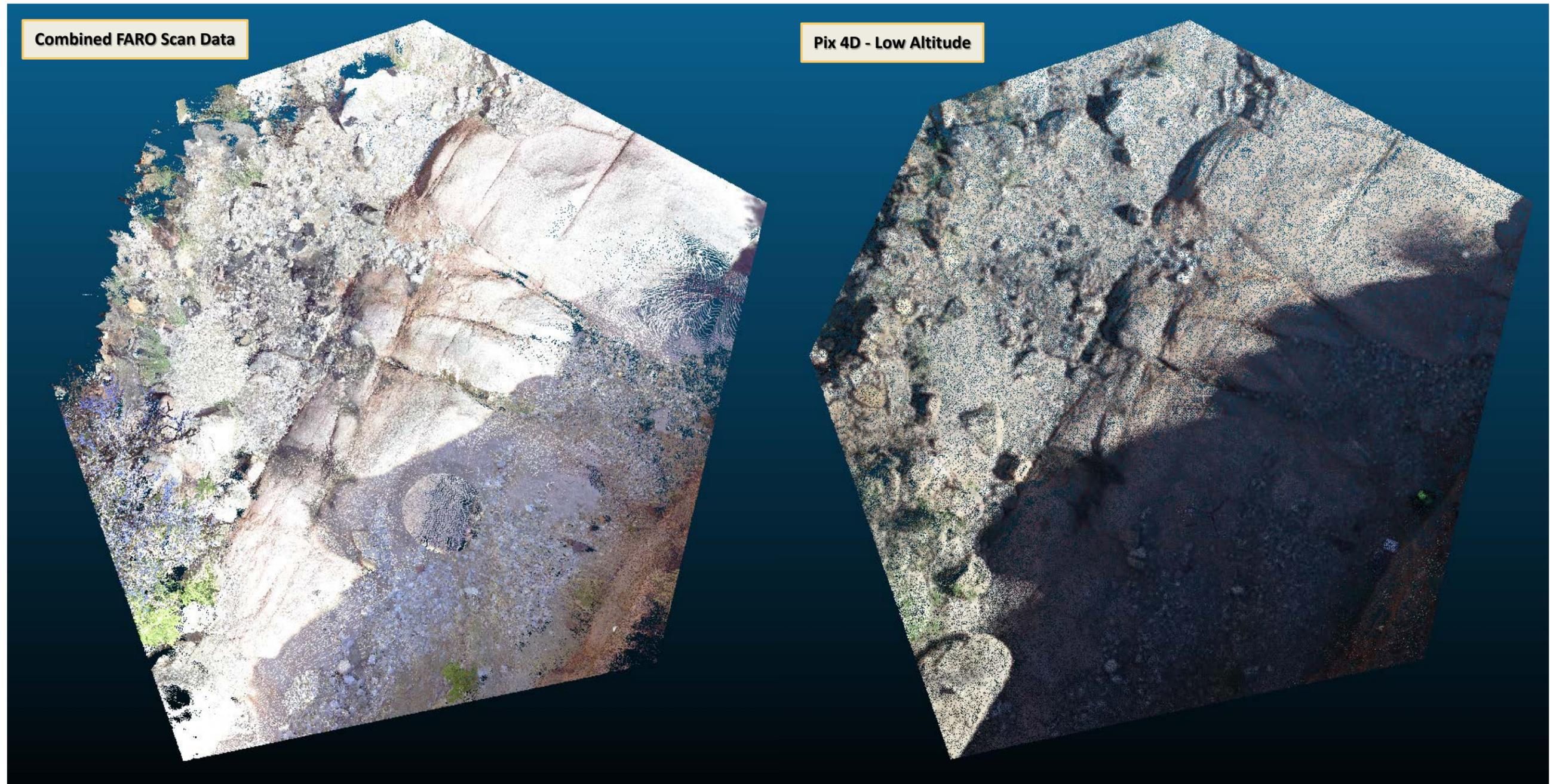
Figure 15 - Side by Side comparison of overhead view of FARO and UAS point clouds
