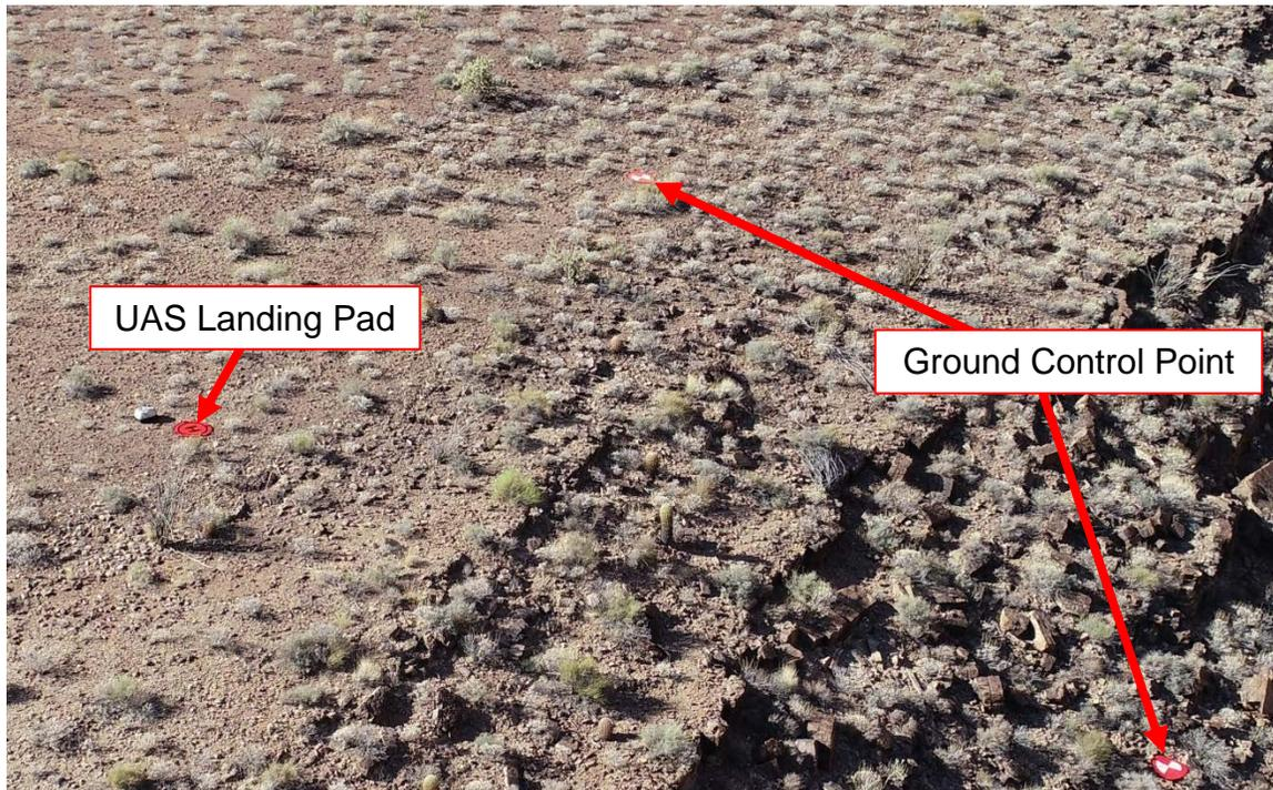
**Figure 1 - Aerial view showing UAS landing pad and removable GCPs (not all GCPs shown)**
