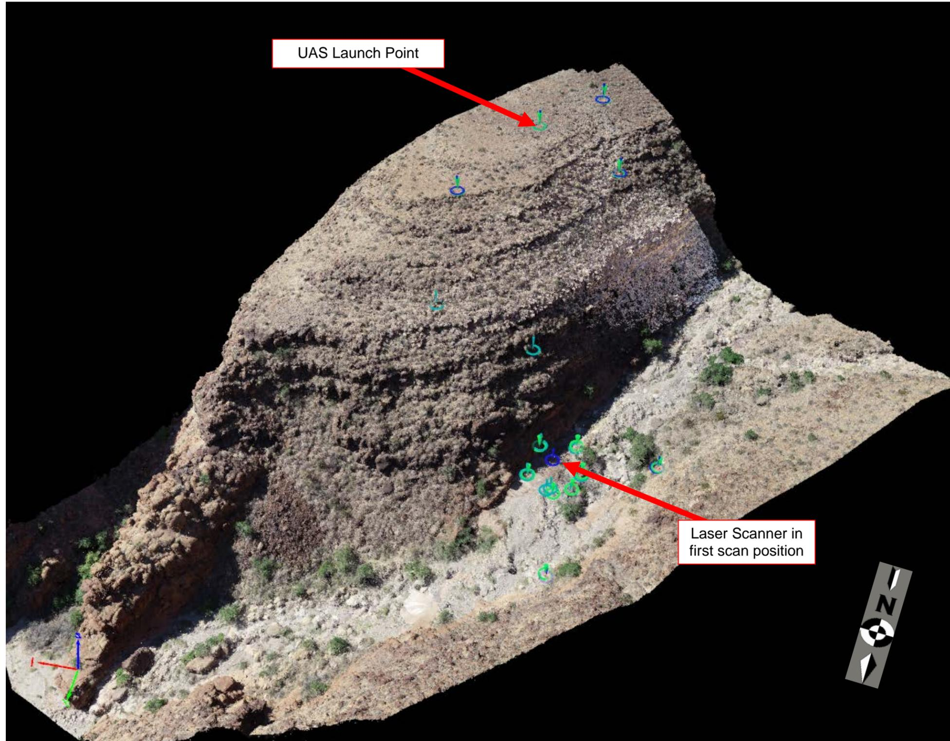
Figure 10 – Screenshot – Pix4D point cloud of low altitude dataset, GCPs and laser reference spheres shown as blue/green markers (directional arrow approximated)
