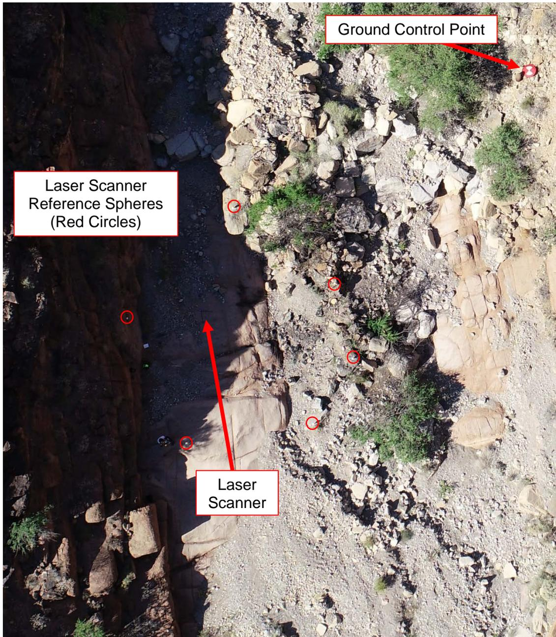
Figure 2 - Aerial view of the accident site showing laser reference spheres and one GCP
