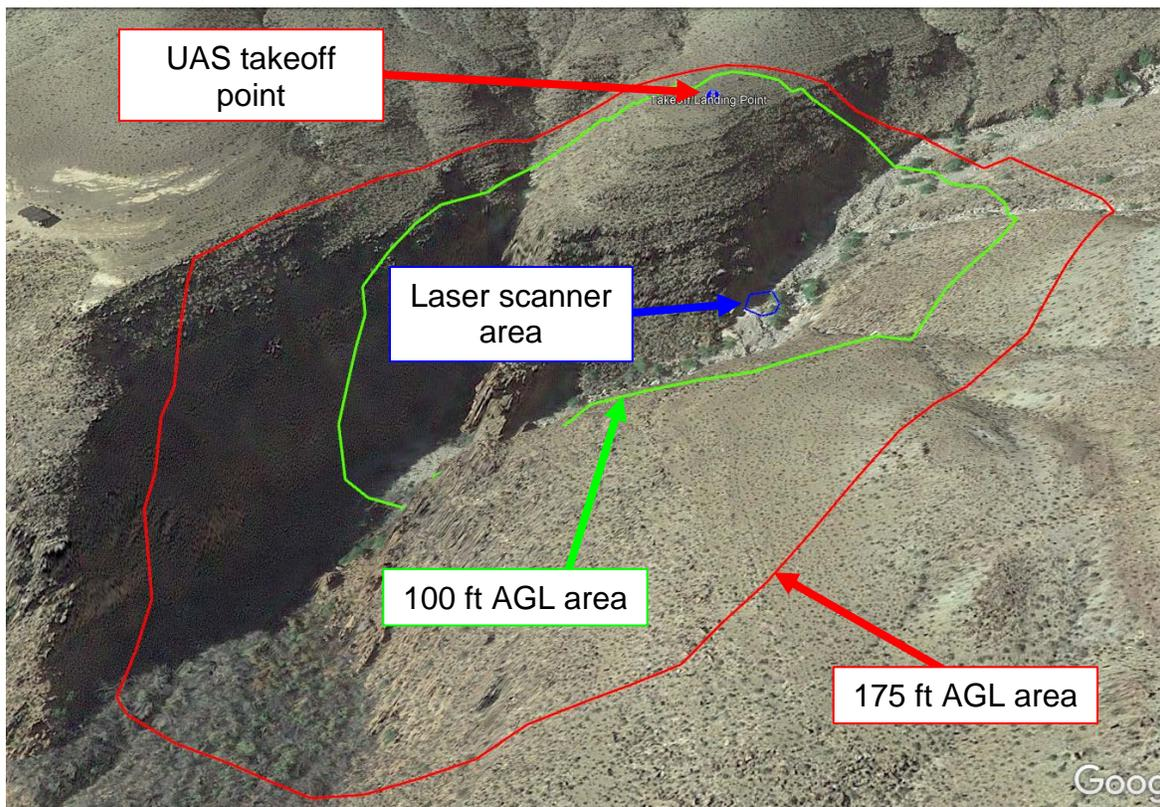
**Figure 3 - Approximate extent of area covered by the FARO scanner and UAS**
