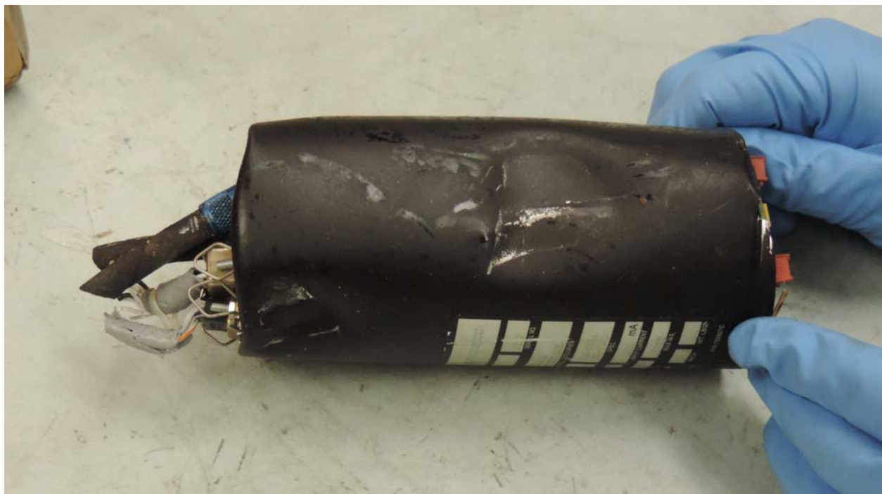
Figure 1. Damage to exterior of Shadin Fuel/Air Data Computer
