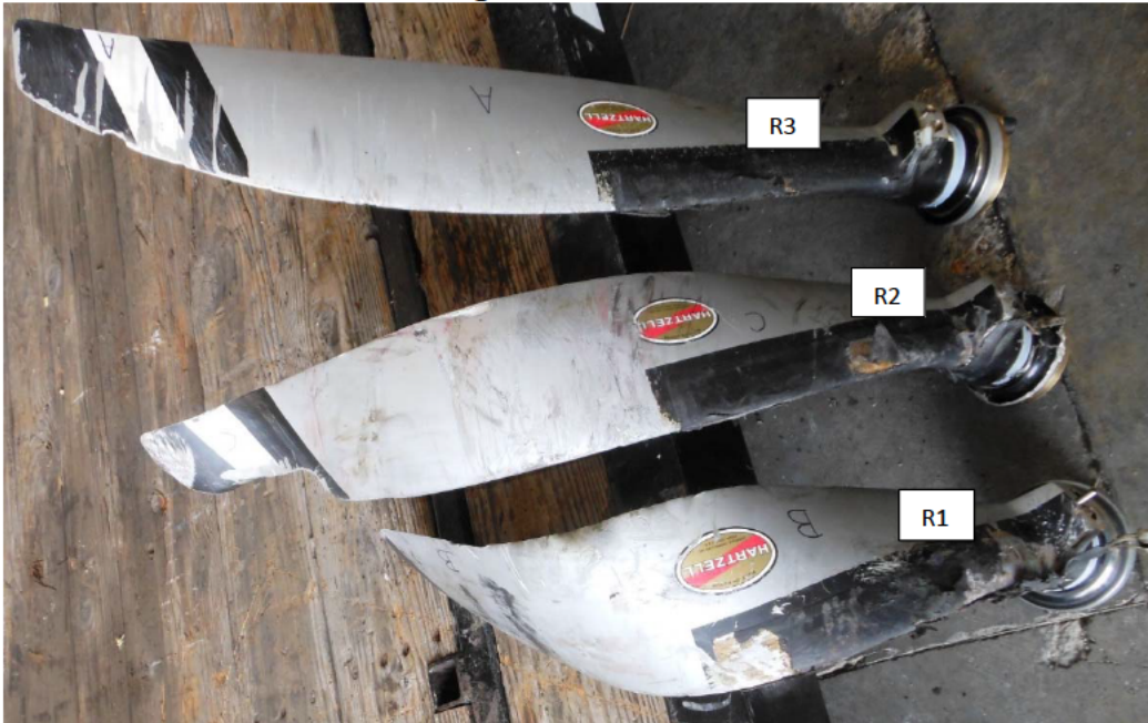
Photo #17 – Right blades camber side view
