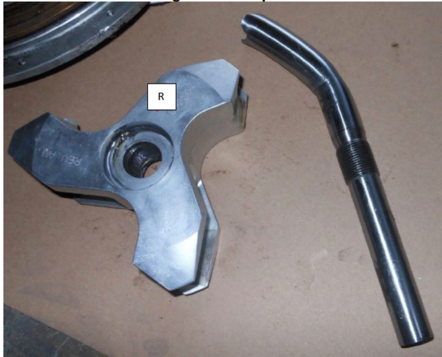
Photo #11 – Right fork and pitch change rod
