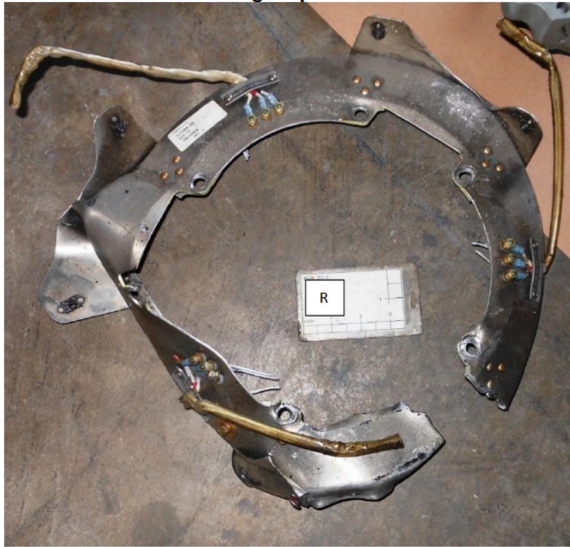
Photo #8 – Right propeller/hub mounting flange
