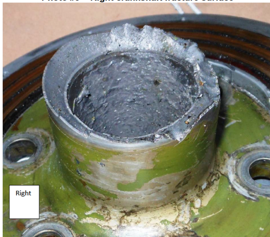
Photo #9 – Right crankshaft fracture surface
