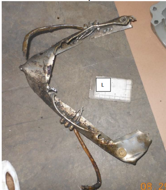
Photo #25 – Left spinner bulkhead
