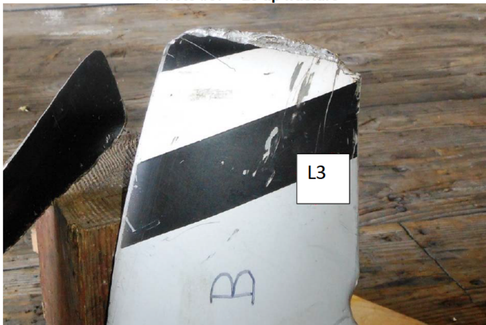
Photo #37 – L3 tip fracture
