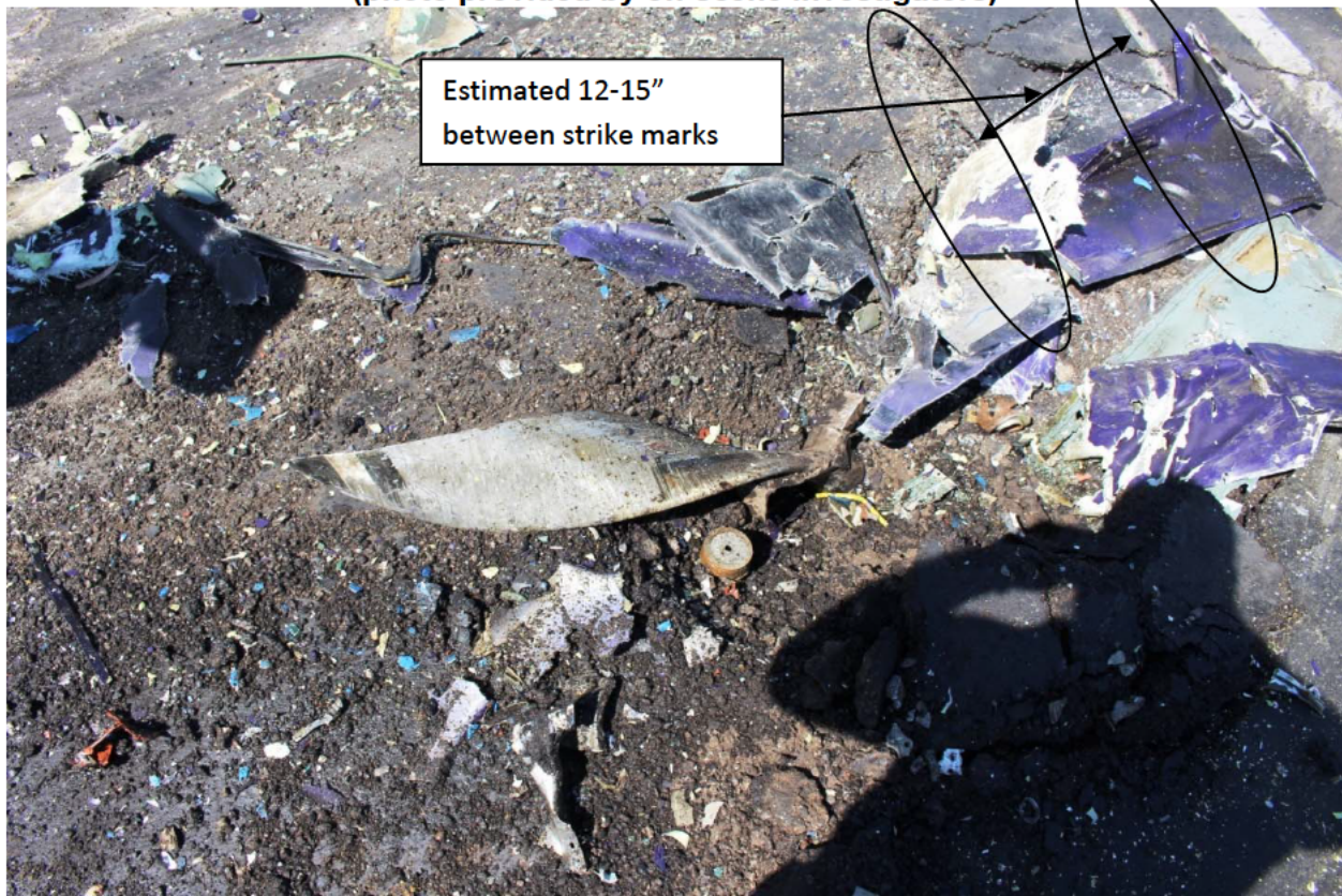
Photo #23 – L2 blade in impact crater (photo provided by on-scene investigators)
