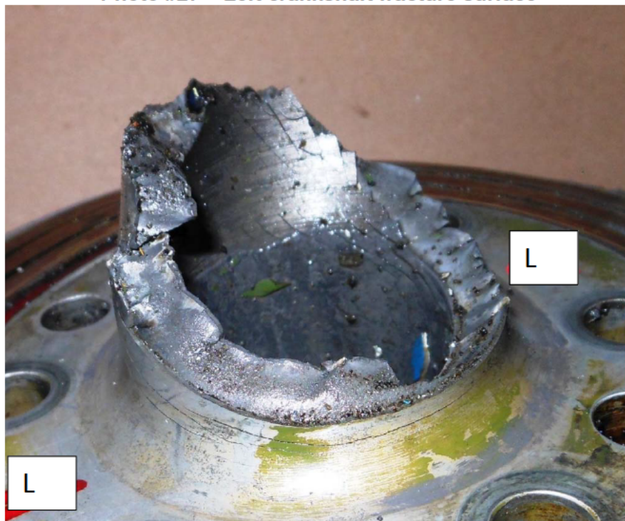
Photo #27 – Left crankshaft fracture surface
