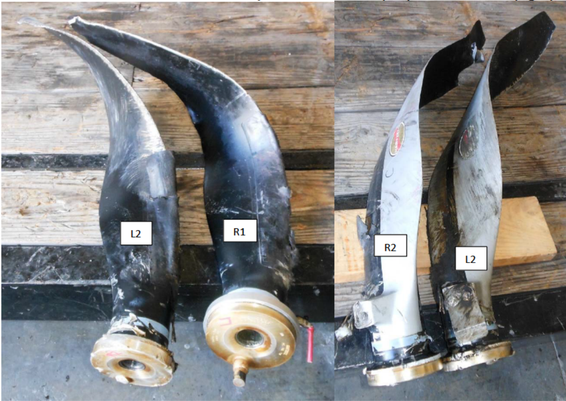
Photo #1 – Relative bend/twist comparison L2 vs. R1 (left) and R2 vs. L2 (right)
