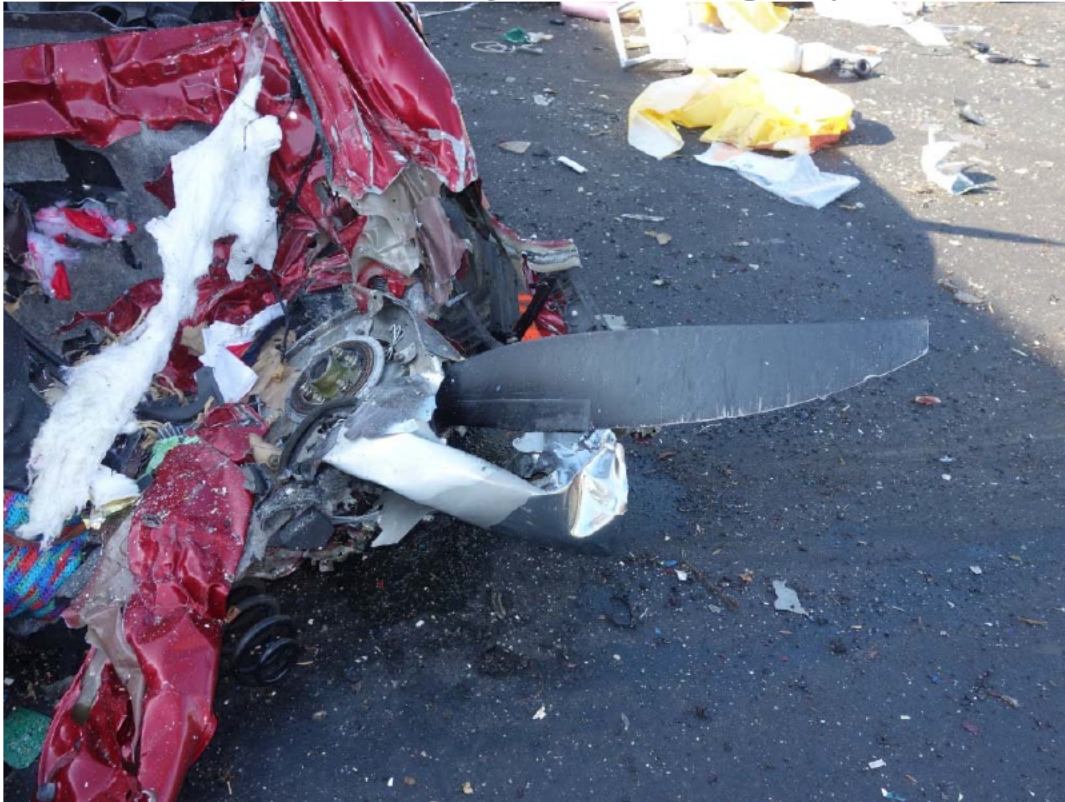
Photo #3 – Right propeller in-situ embedded in car (Photo provided by on-scene investigators)
