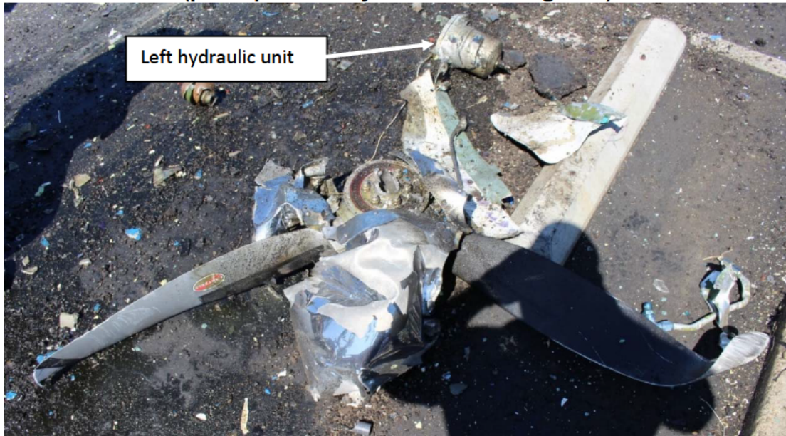
Photo #22 – Left propeller in-situ (photo provided by on-scene investigators)
