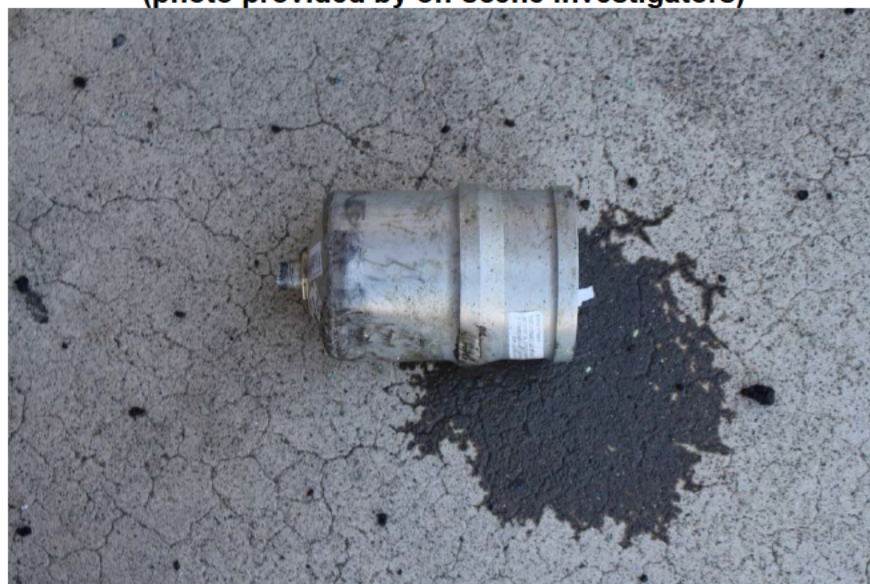
Photo #10 – Right hydraulic unit in-situ (photo provided by on-scene investigators)
