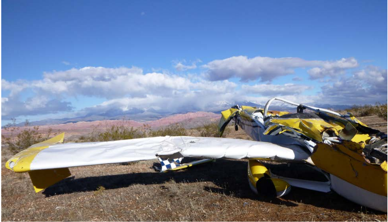
Figure 4 – Right wing deformation
