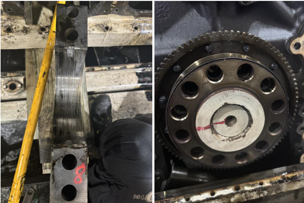
COUNTERWEIGHT, BEARINGS AND DAMAGED SHAFT
