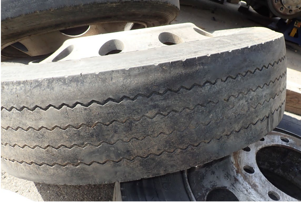
Photo shows the tread wear to the left rear outside dual tire.
