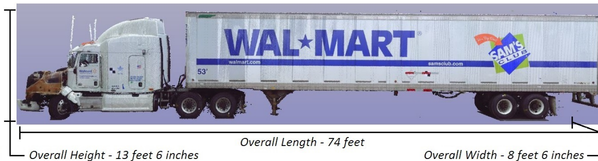
Figure 1. Driver (left) side profile from the 3-dimensional model of the damaged 2011 Peterbilt combination unit.
