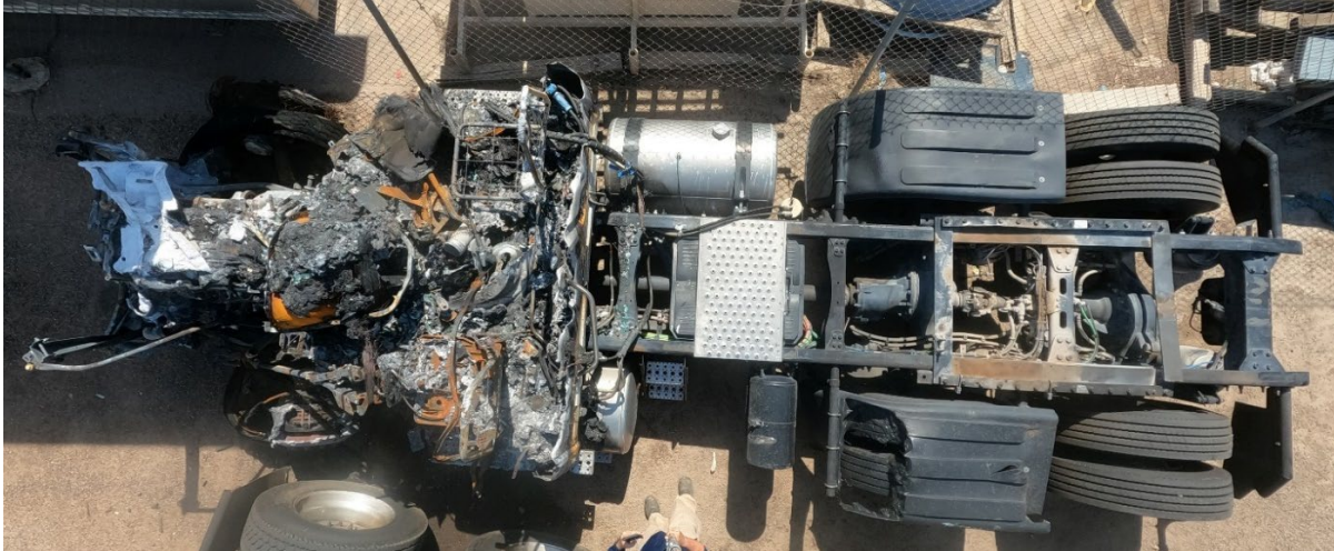
Figure 2 - A top-down view of the truck-tractor, showing collision and post fire damage.
