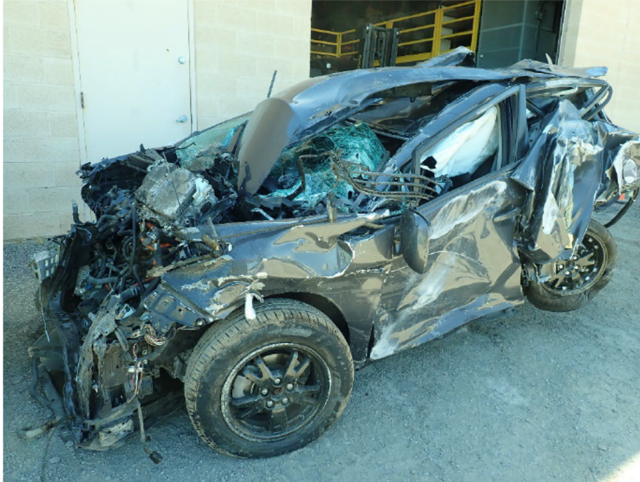
Figure 17 - Left-side view of the 2013 Toyota Prius showing extensive collision damage.
