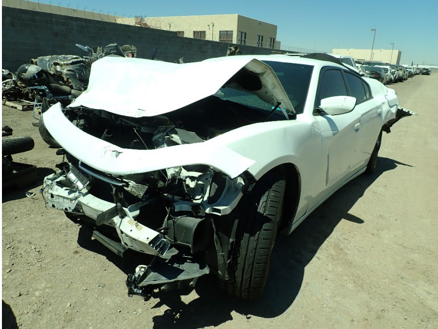
Figure 15 - A front and left-side view of the 2015 Dodge Charger showing front end collision damage.
