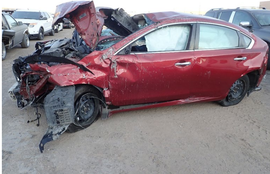
Figure 9 - A left-side view of 2015 Nissan Altima showing front, side roof and rear damage.
