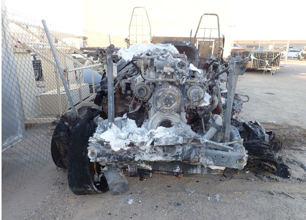
Figure 4 - A front view of the truck-tractor, showing collision and post fire damage.
