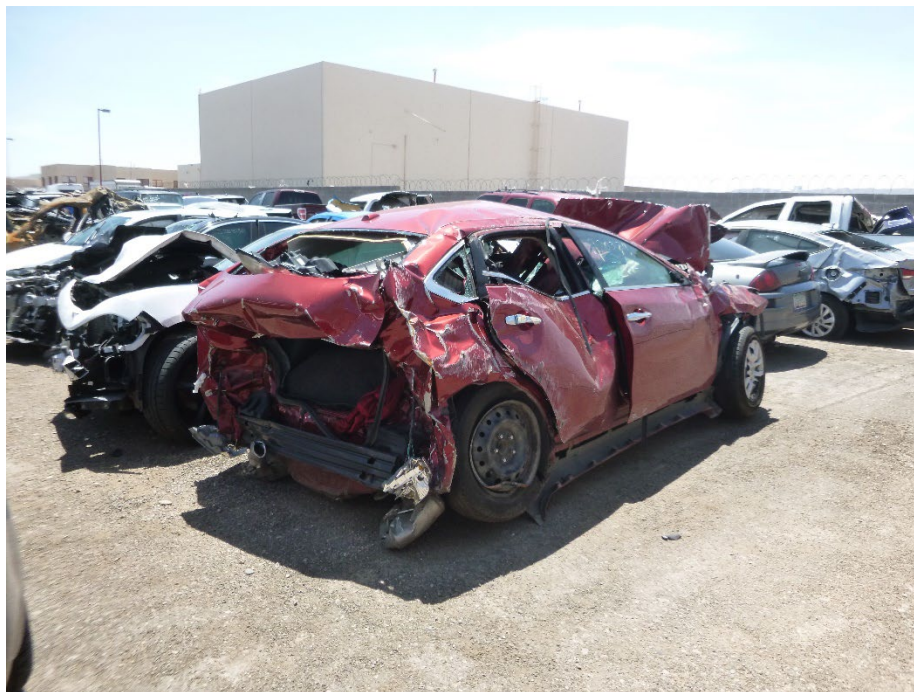
Figure 10 – A rear and right-side view of the 2015 Nissan Altima showing rear and right-side collision damage.
