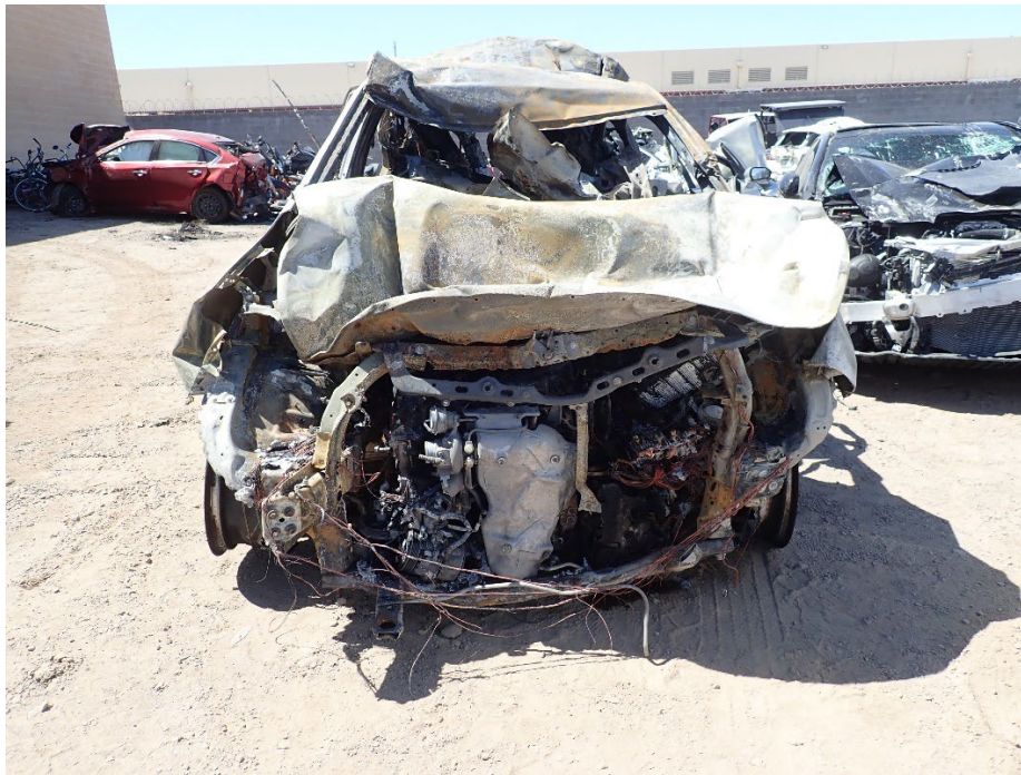
Figure 7 - A front view of the 2021 Chevrolet Equinox LS showing extensive front-end collision and post-crash fire.
