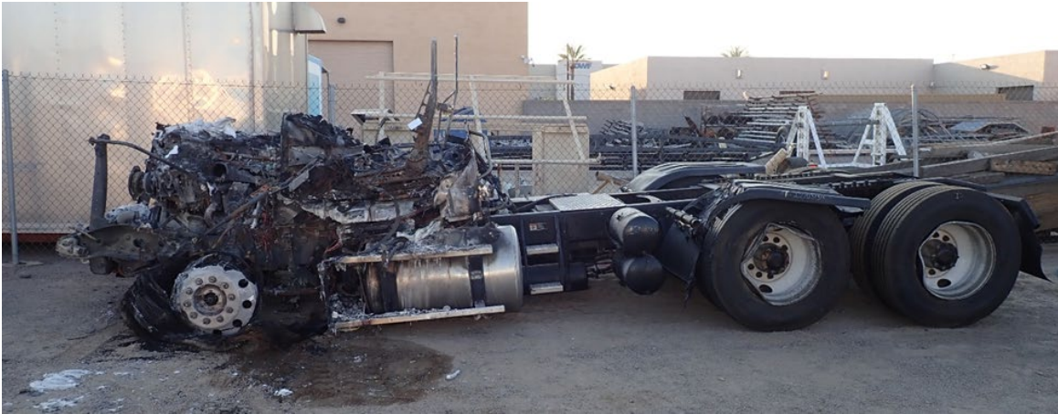
Figure 1 - A left-side view of the truck-tractor showing collision and post fire damage.
