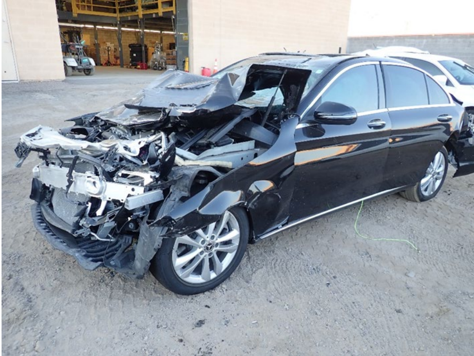
Figure 11 - A front left-side view of the 2018 Mercedes C300W showing front end and rear bumper collision damage.
