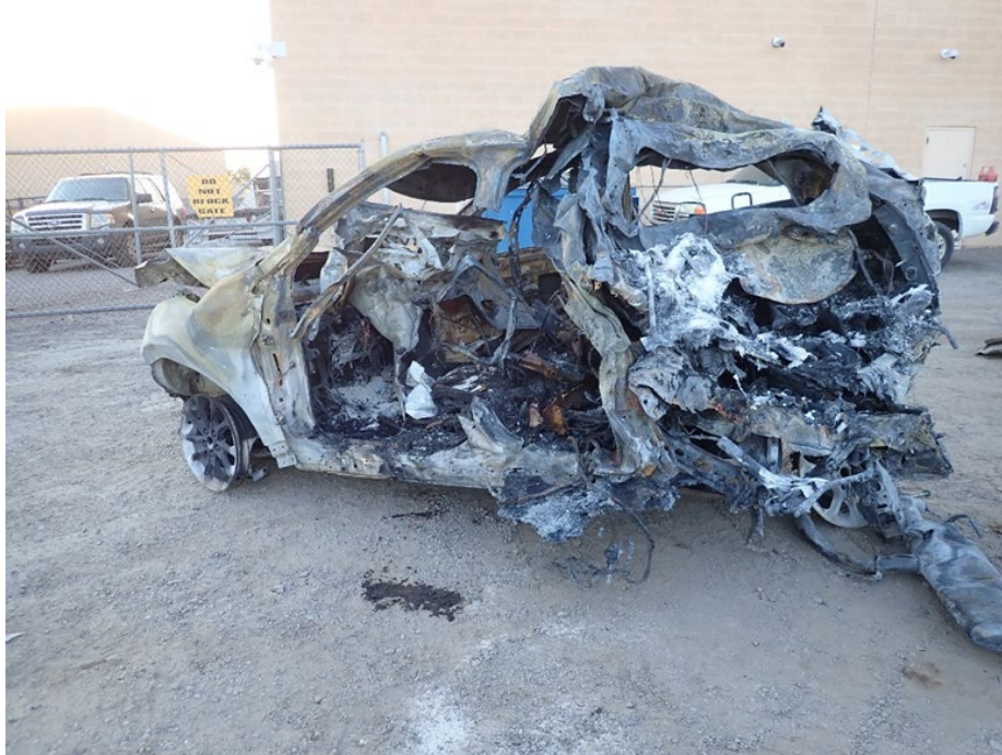
Figure 8 - Left-side and rear view of the 2021 Chevrolet Equinox LS showing extensive collision and post-crash fire damage.
