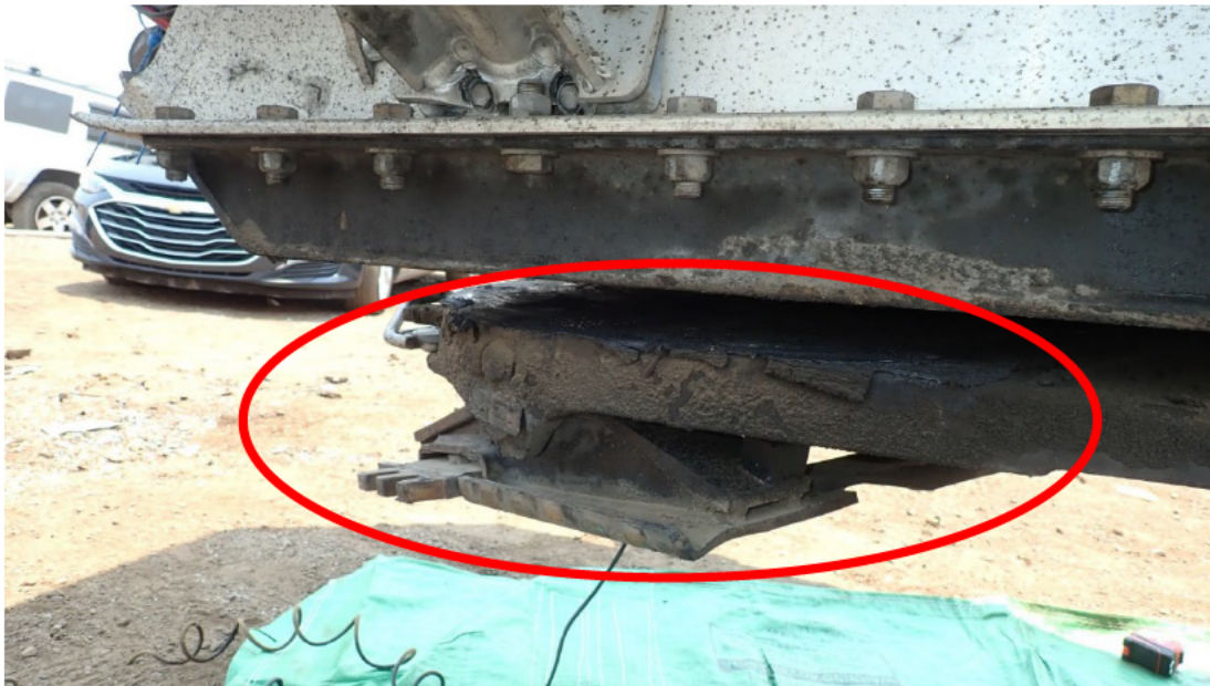
Figure 6 - The 5 th wheel plate from the truck-tractor torn from the tractor still attached to the tank-trailer's kingpin.
