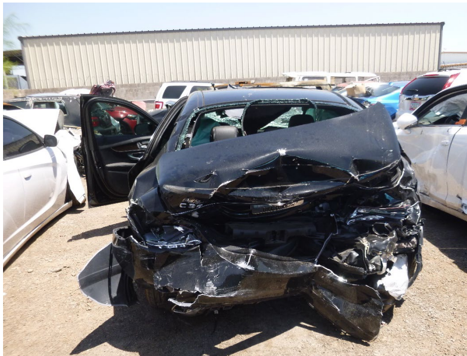
Figure 12 - A rear view of the 2018 Mercedes C300W showing collision damage.
