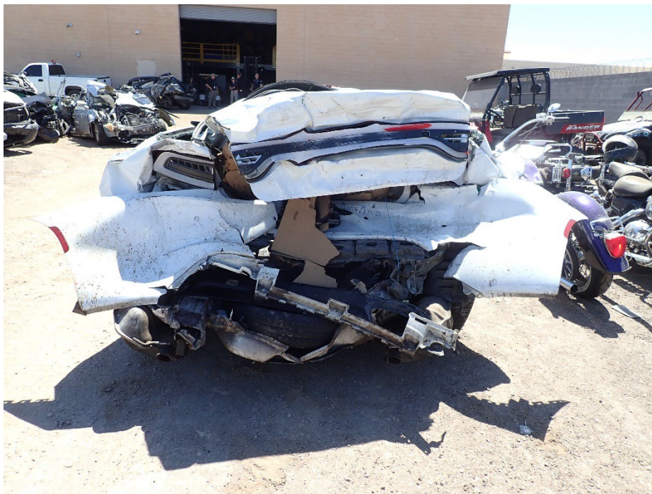
Figure 16 – A rear view of the 2015 Dodge Charger showing rear collision damage.
