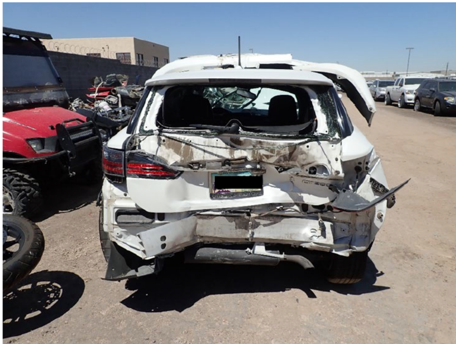
Figure 14 – A rear view of the 2013 Lexus CT200H, showing extensive rear contact damage.
