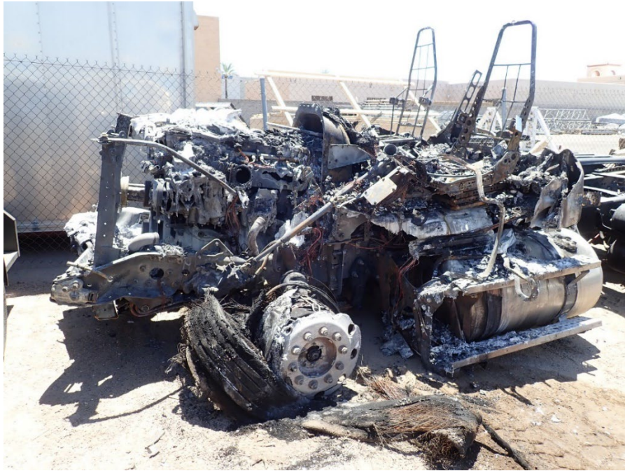
Figure 3 - A left-side view of the truck-tractor showing the entire cab and engine severely fire damaged.
