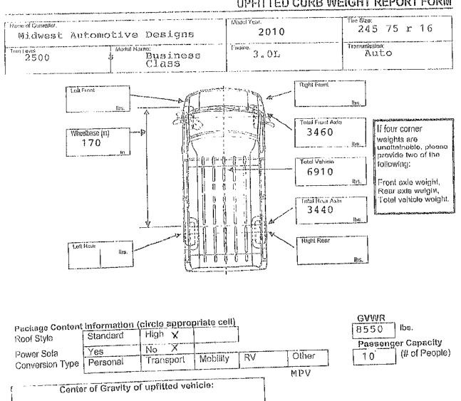
GVWR: Gross Vehicle Weight Rating set forth by the Original Equipment Manufacturer (OEM), it is the maximum allowable Definitions weight the vehicle may sustain. GVWR is equal to the sum of the Unloaded Vehicle Weight (UVW) and the Cargo carrying
