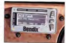
DIU: System Problem Warning
