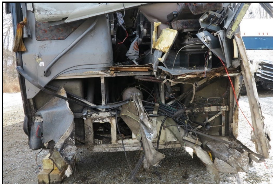
Photograph 2: A closer view of the front of the 2005 Van Hool motorcoach – notice the driver's seat.
