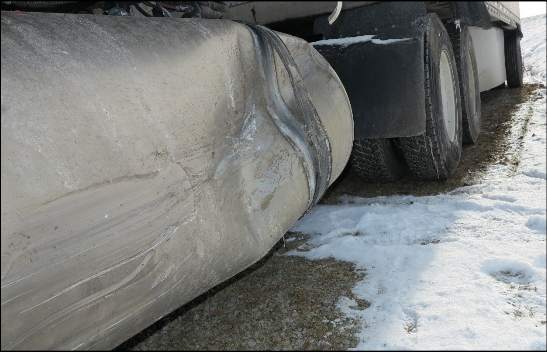
Photograph 22: A closer look at the damage to the left-side fuel tank mounted on the UPS #2 2018 Freightliner.
