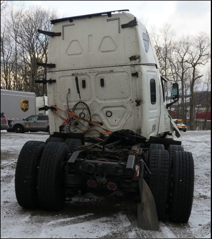
Photograph 8: Looking at the rear of the 2018 FedEx truck-tractor and displaced cab.
