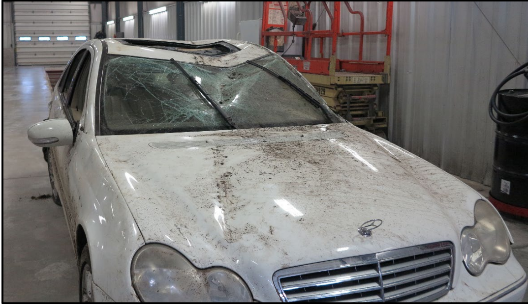
Photograph 19: A view of the crease that is on the hood and roof of the 2007 Mercedes.
