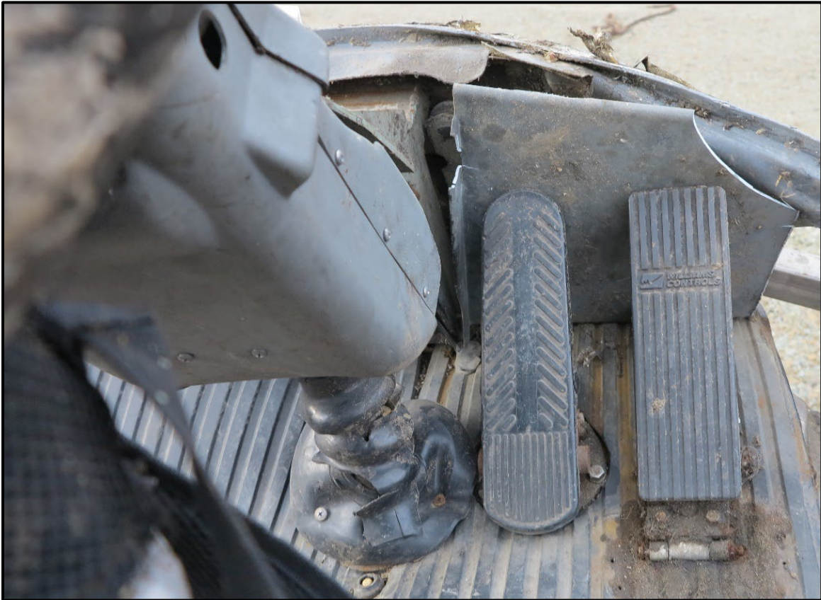
Photograph 6: A view of the accelerator and brake pedals from the 2005 Van Hool motorcoach.
