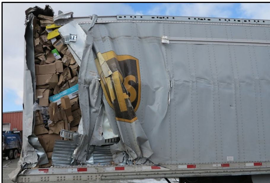
Photograph 18: Looking at the damage sustained to the forward section on the left side of the 2018 Stoughton semitrailer
