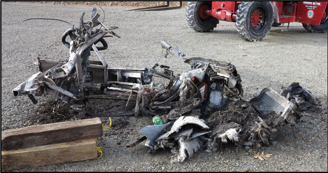
Photograph 5: The recovered steering components, dash, and stairwell from the 2005 Van Hool motorcoach.
