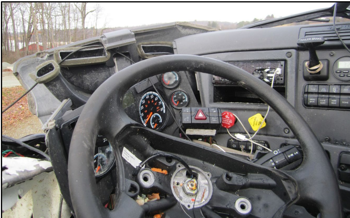
Photograph 16: This is a view of the displaced steering wheel and damaged instrument panel from the UPS #1 2018 Freightliner.
