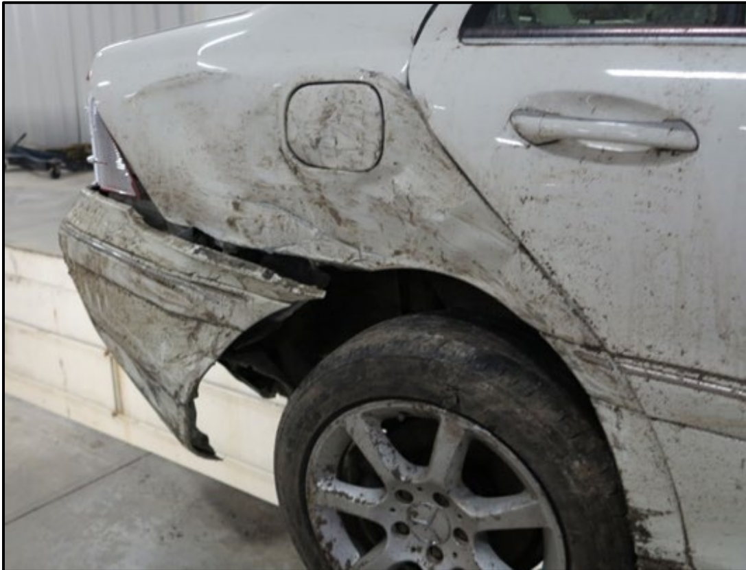
Photograph 20: A view of the damage sustained to the right-rear of the 2007 Mercedes.
