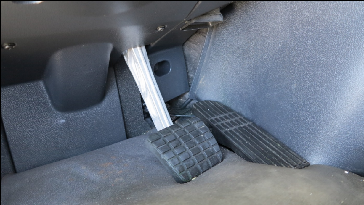
Photograph 10: Looking at the trapped brake and accelerator pedals of the 2018 FedEx truck-tractor.
