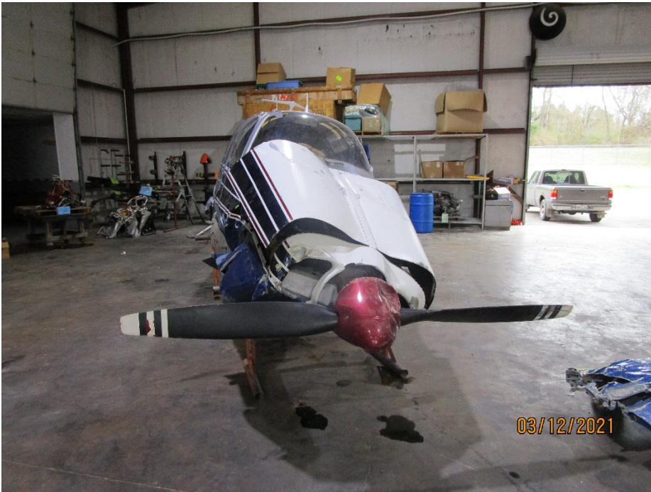
2-bladed propeller appeared to be absent power signatures
