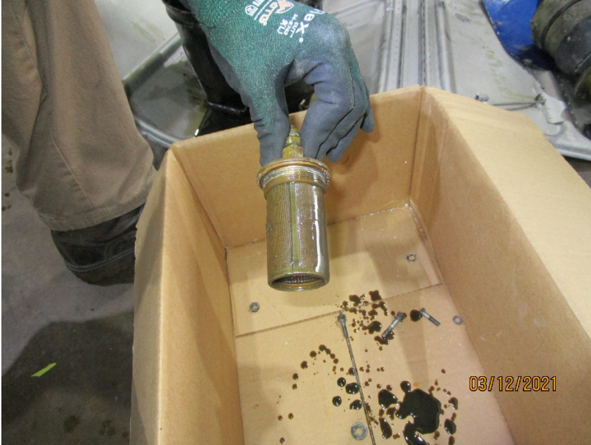
Oil screen contained unidentified contaminants
