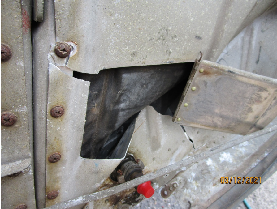
Left sided did leak, there appeared be a post-cash puncture at the wing root
