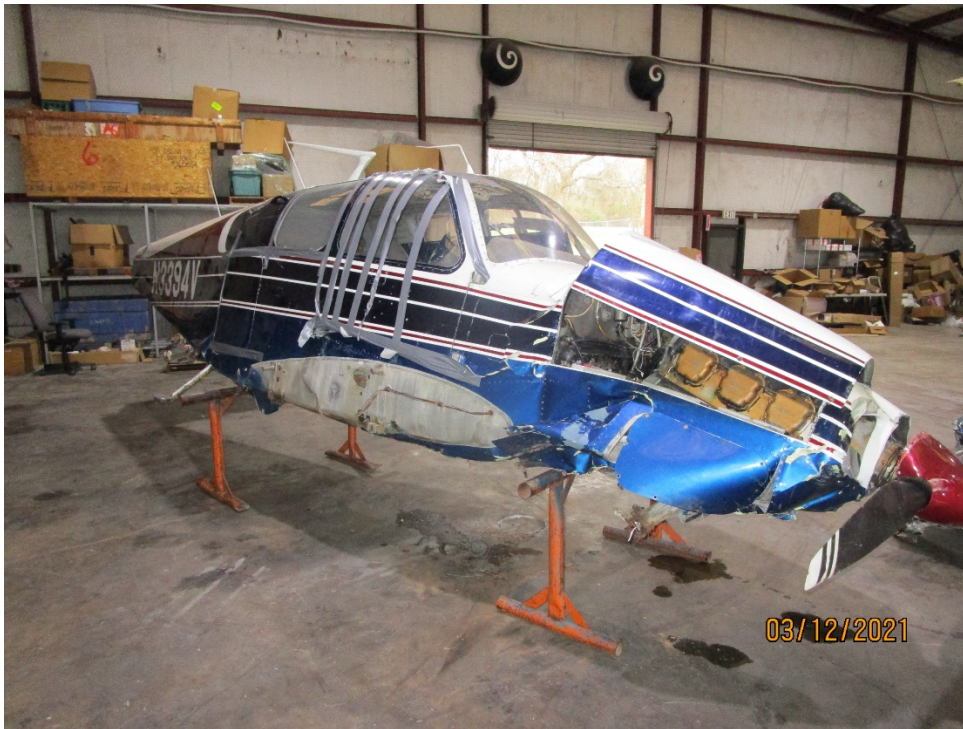
Airplane wreckage on stands, ready for inspection
