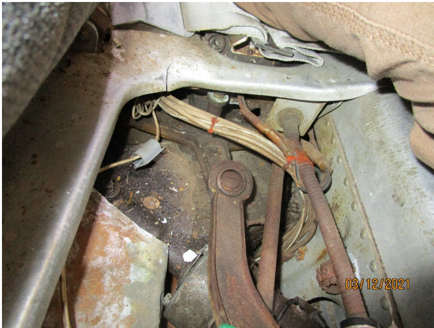
Landing gear circuit breaker was “popped”. Gear indicator in the down position And landing gear motor, indicate the landing gear was in the down position.
