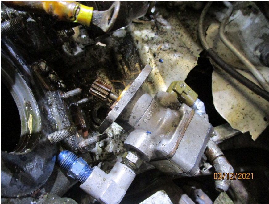
Fuel pump drive coupling, intact, pump rotated freely
