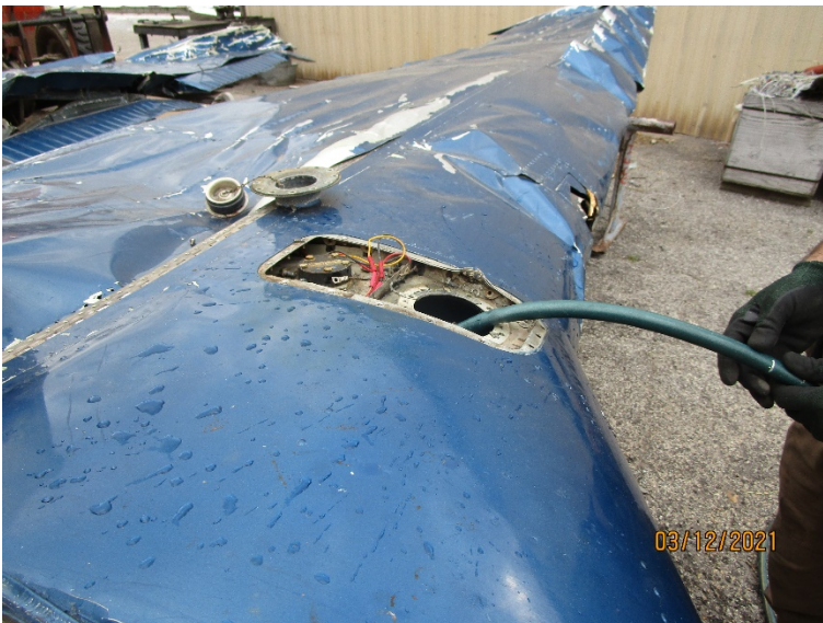
Testing fuel tank for leaks
