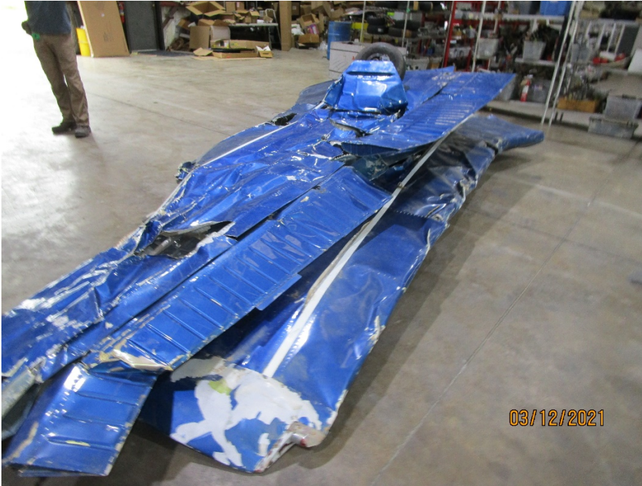
Heavy damage was noted to both wings
