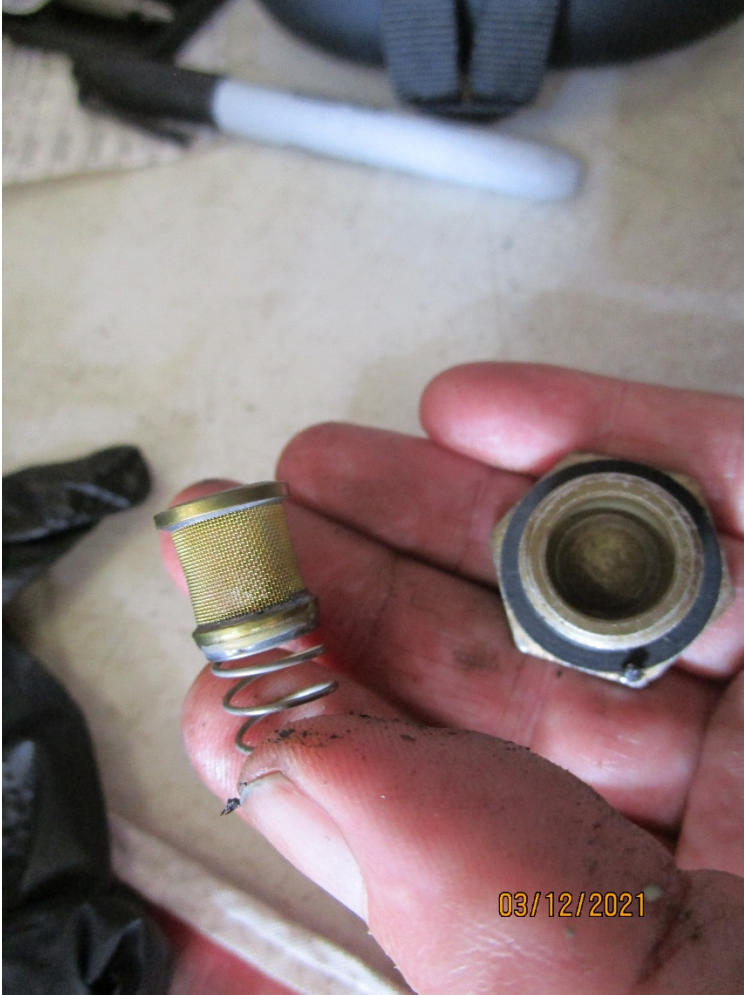
Fuel screen from the carburetor; clear of contaminants.
