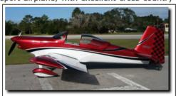
qualities and superior handling. A typical RV-7 can hold two FAA standard pilots, 100 lbs. of baggage and full tanks: 42 gallons. At aerobatic gross the weight of 1600 lbs., the RV-7/7A complies with the +6/-3G standards of the FAA's Aerobatic Category and can still two carry people,
