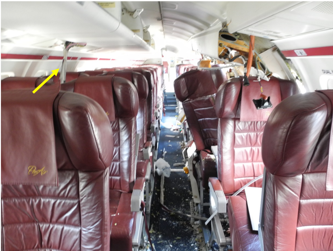
Photo 11. Aft-facing view showing inboard displacement of seat 4A's seatback and location of propeller blade near seat 4F.
