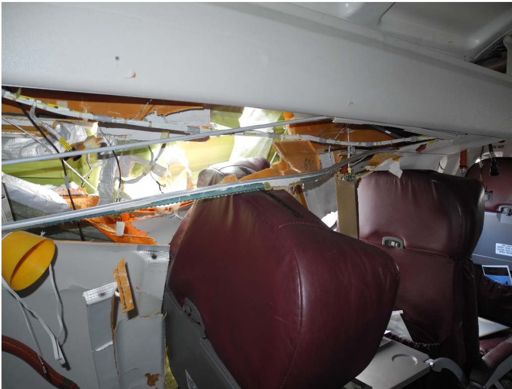
Photo 9. Interior damage above seat 4A.
