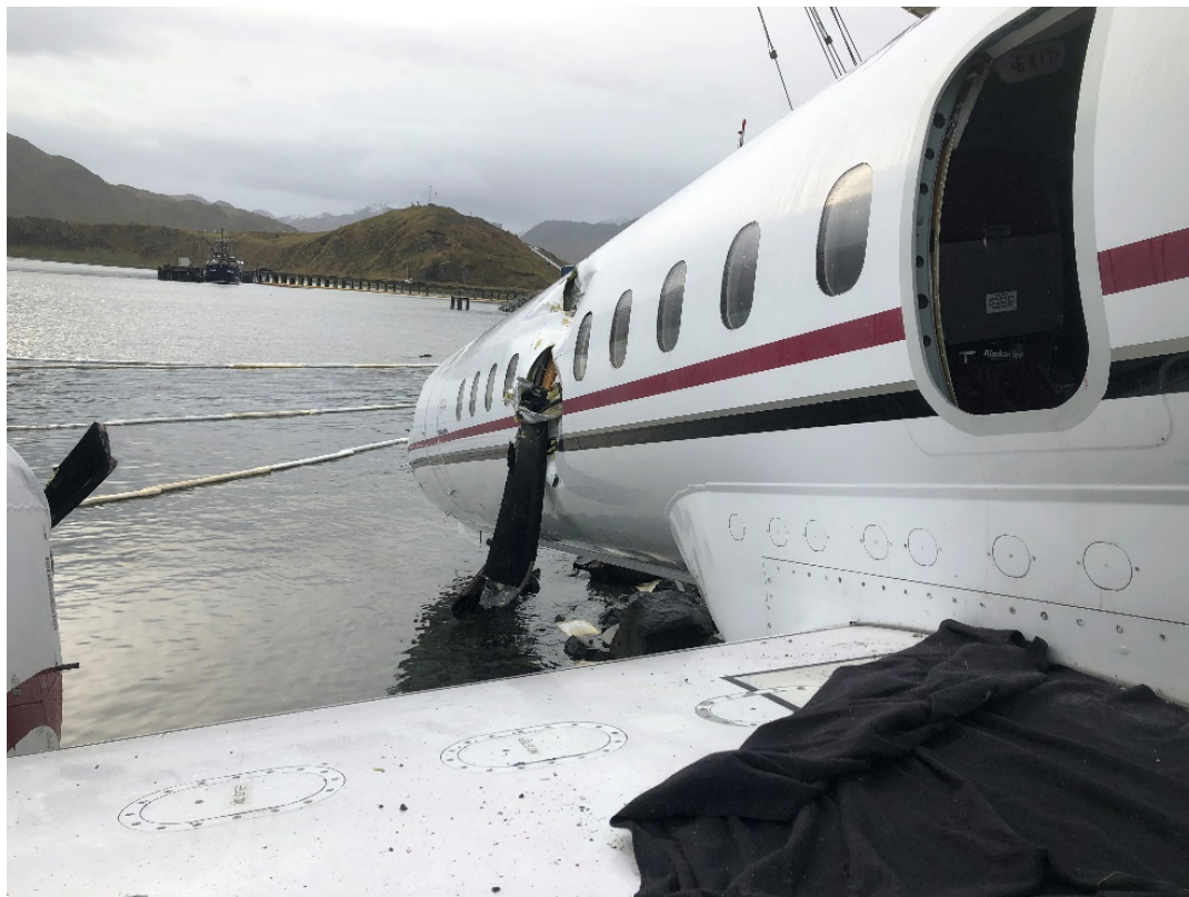
Photo 4. Left overwing exit and impact area of propeller blade.
