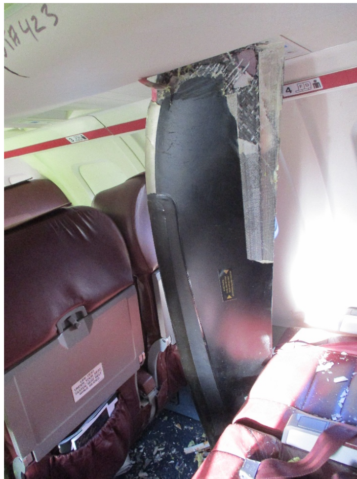
Photo 12. Location of propeller blade near seat 4F.
