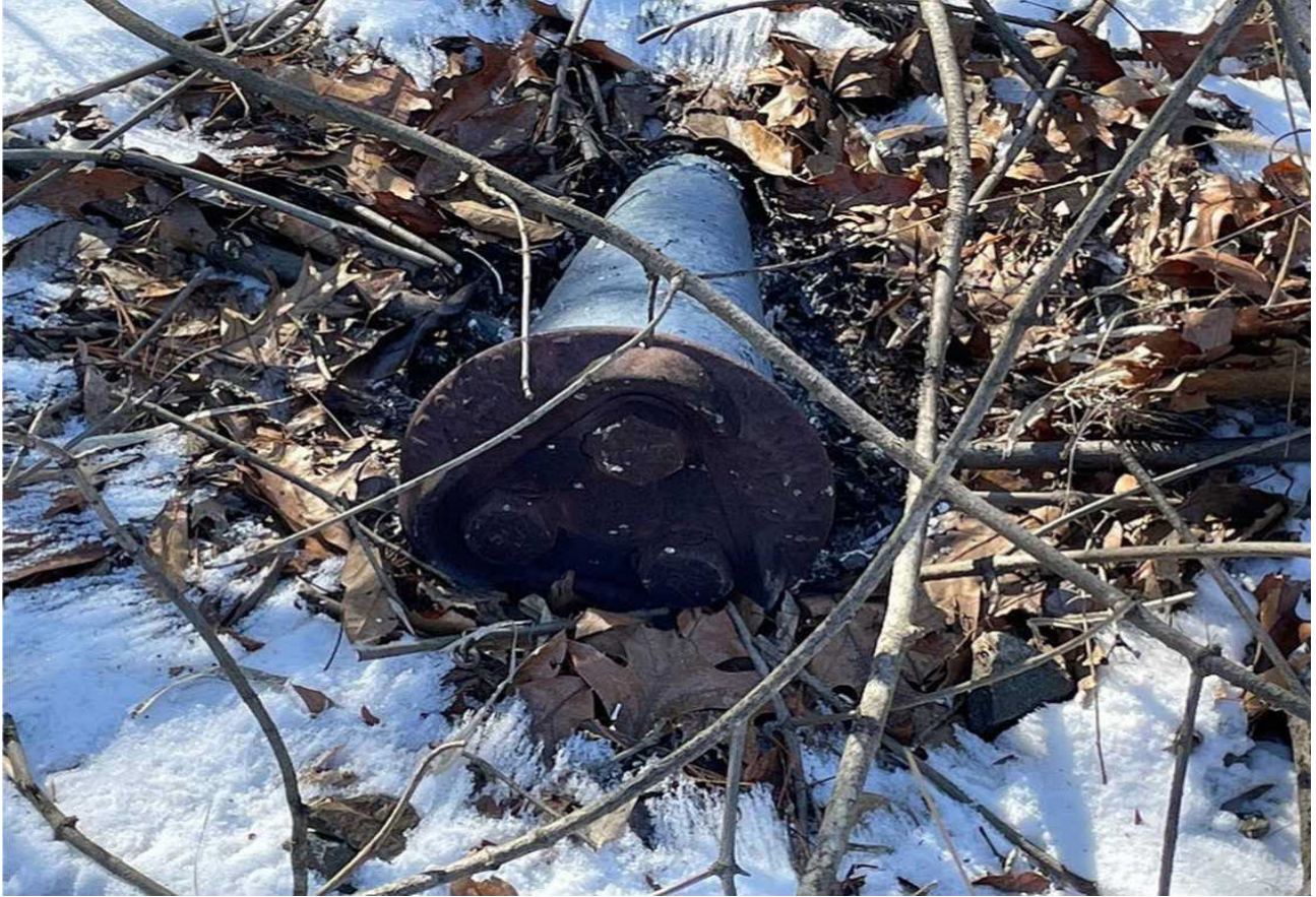
Figure 3- Final resting location of the burnt off journal.
