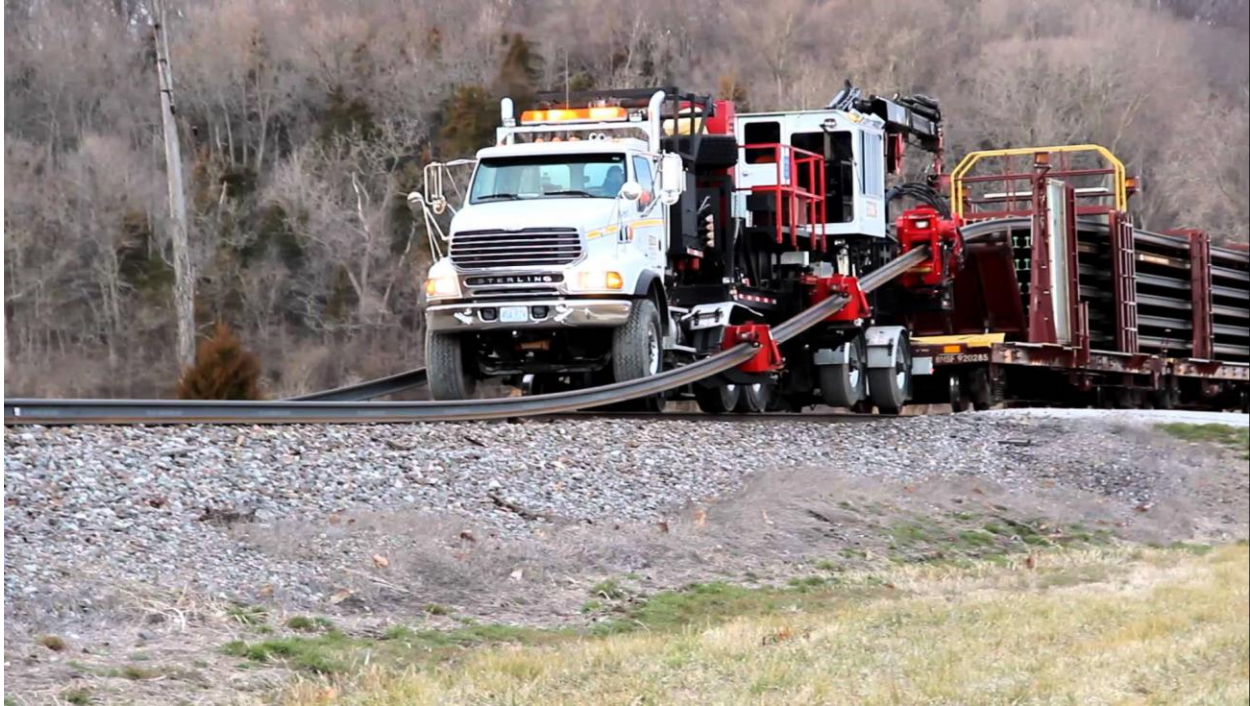
Figure 5. Photo of the RUM unloading rail from a CWR work train. Picture courtesy of BNSF.
