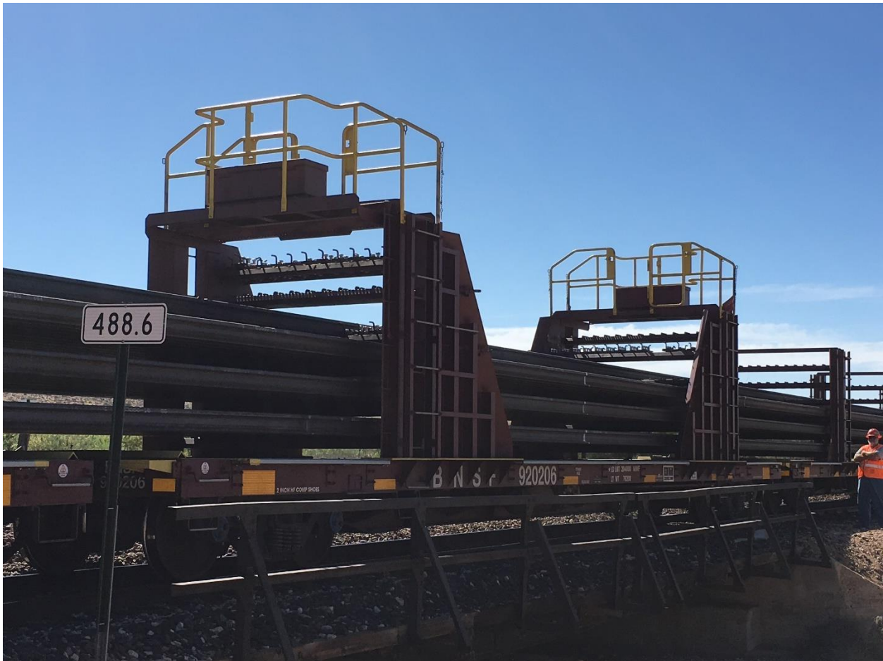
Figure 6. Photo of the last CWR flatcar with the 2- catwalks that span overtop the rails.
