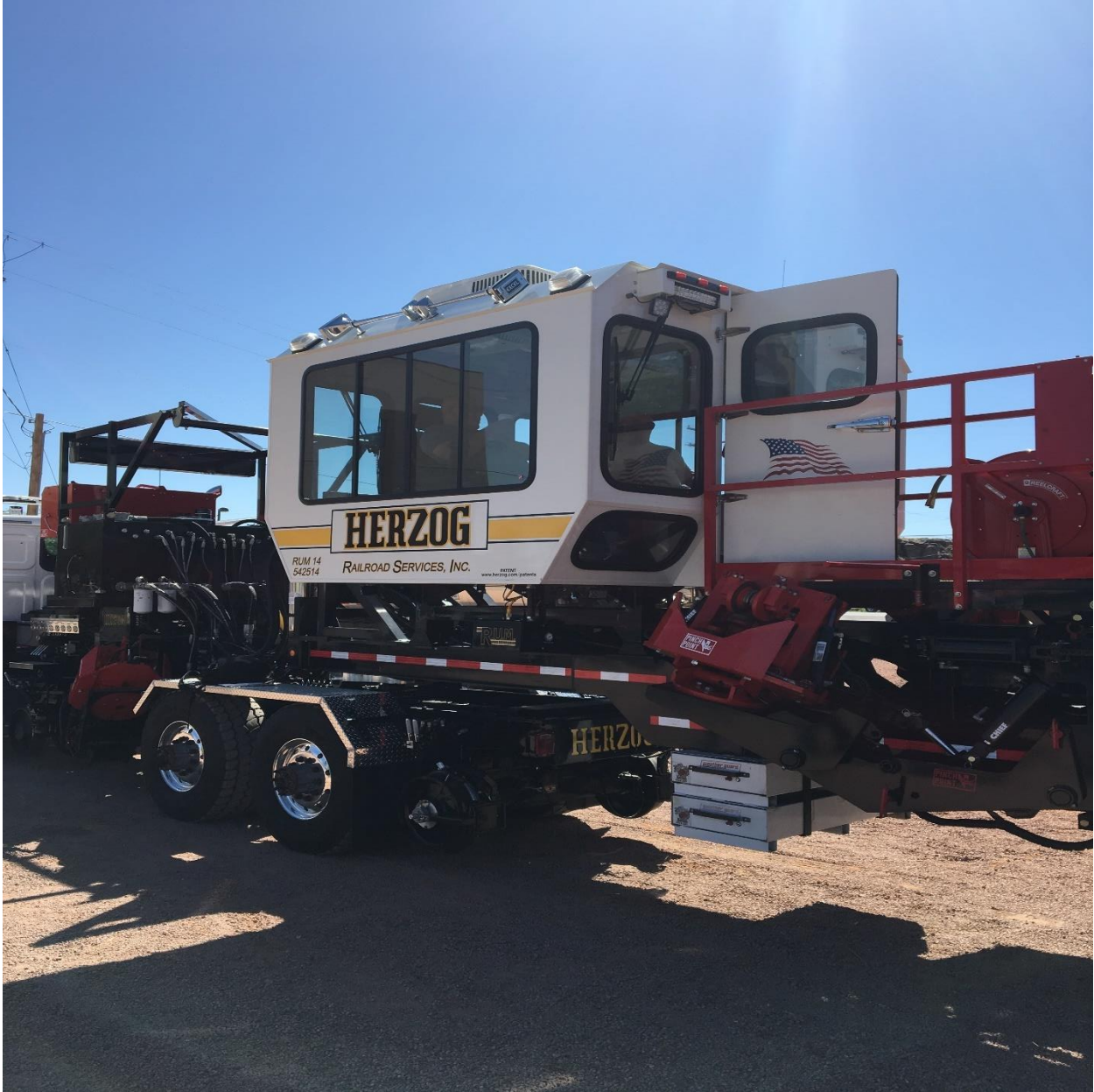
Figure 3. Photo of the RUM's attached trailer, work cab and rail handling attachments.
