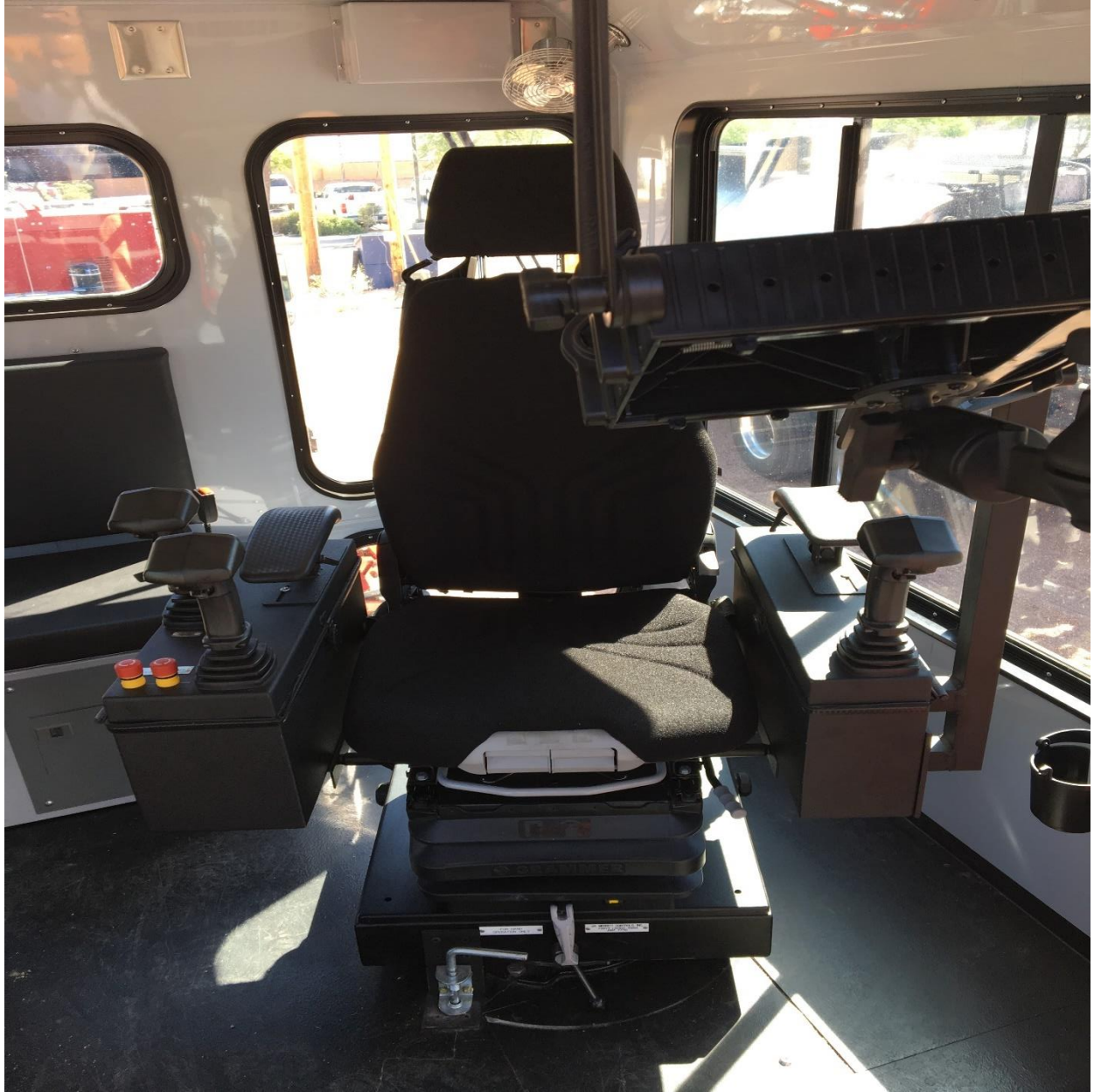
Figure 4. Photo of a high-back chair where the CWR rail attachments are operated via joy sticks
