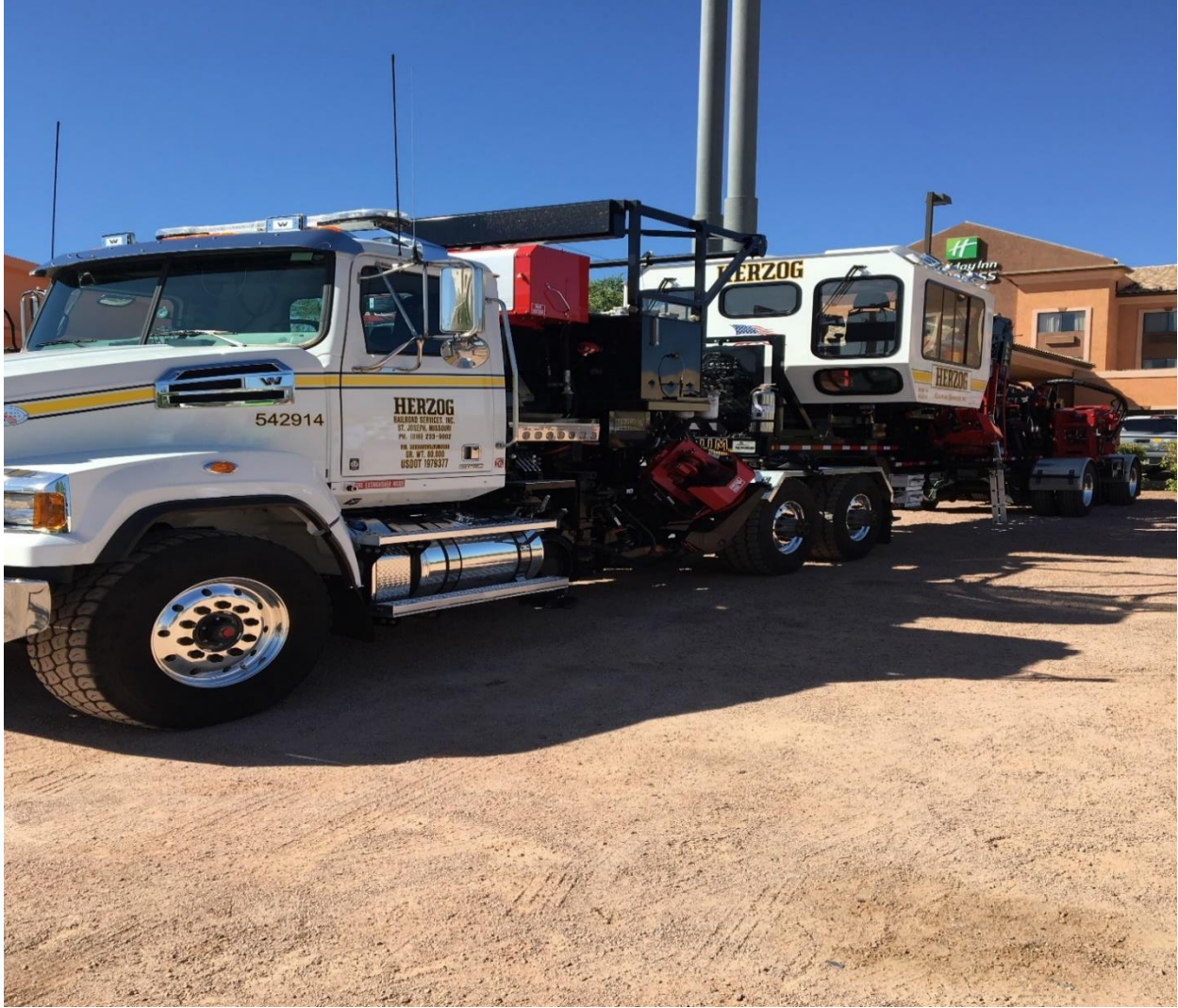
Figure 2. Photo of Herzog’s rail unloading machine or RUM.
