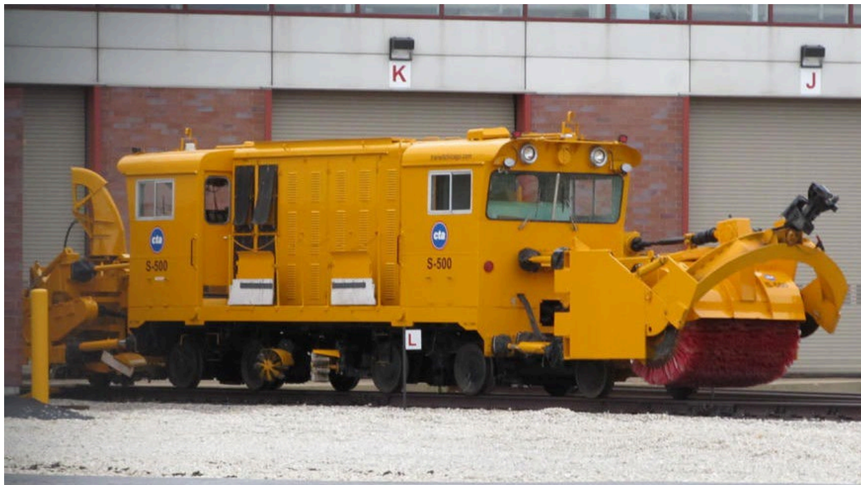
7 8 Figure 1: Photo of S-500 Diesel Snow Locomotive. (Source: rrpicturearchives.net) 9
