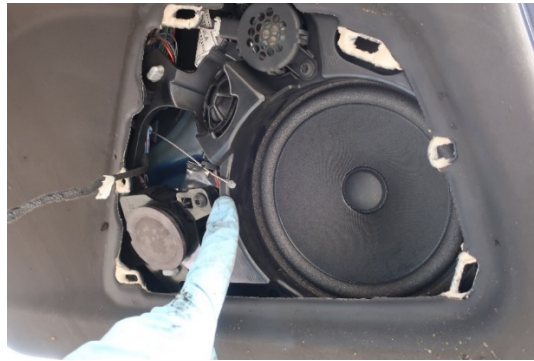
Figure 4. Cable in rear door speaker which needed to be pulled to manually open a rear door after removal of a speaker grill.
