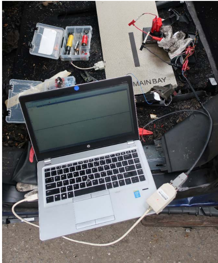
Figure 41. Connections between laptop, battery, and wires of the vehicle battery communication bus. The location is the floor inside of the left rear door, beneath where mid seat had been removed.
