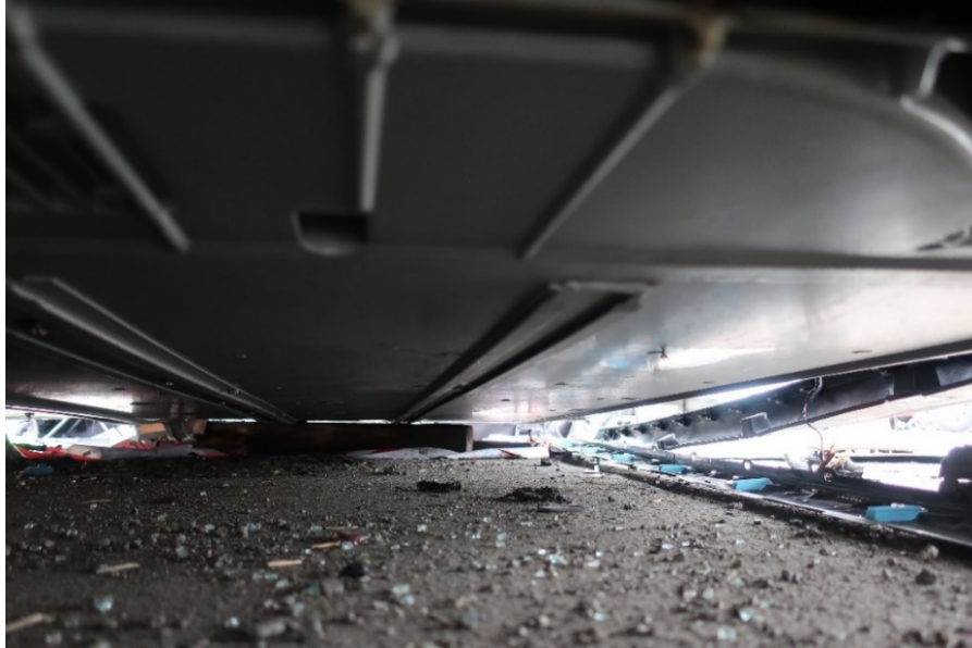
Figure 12 . Smooth bottom surface of battery and limited amount of clearance to ground. Note that wood elevates the front and rear of the vehicle. The discharge port is located to the left of this photo.
