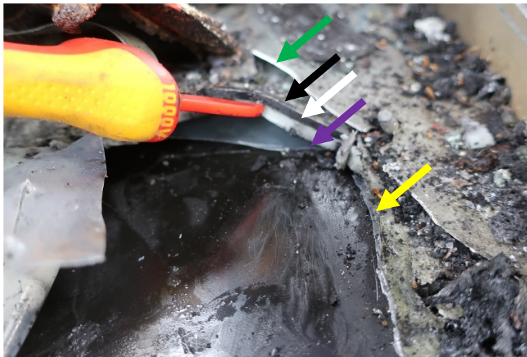
Figure 10. Layering of materials prevents ability of cooling water to flow in space between the vehicle body and steel top of battery. Green points to edge of aluminum vehicle floor pan, black to rubber-like material, white to compressible material, purple to vapor barrier, yellow to the steel top of the battery case.
