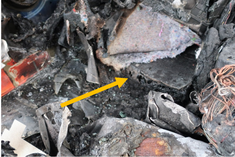
Figure 9. Cut back carpet and pad in driver footwell, lifted from the egg crate foam, which is referenced by the arrow.
