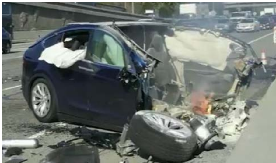
Figure 5. Still image from internet showing deployed side air bags at the scene of the accident with initial fire in front right of battery, prior to fire burning the seats and plastic interior materials.
