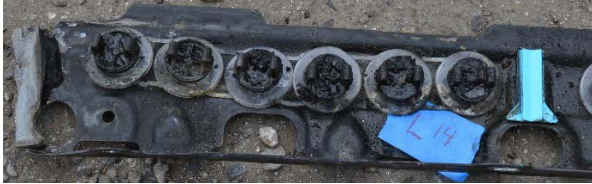
Figure 25. Module 14 poppets and baffle. Note that 25.39 had been measured on the 14 positive bus bar
