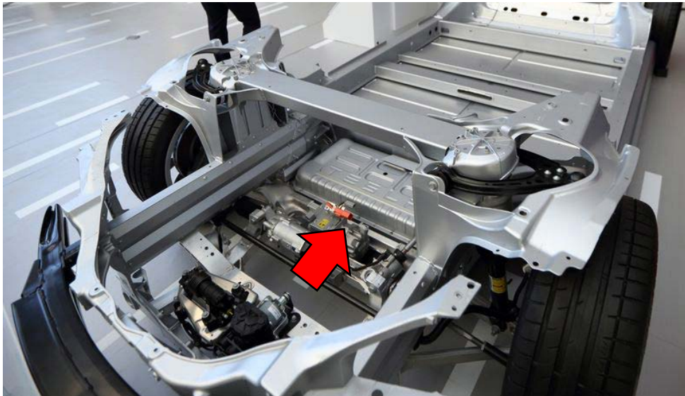
Figure 3. Photo of partial exemplar vehicle with arrow added to depict the leading edge of the battery visible in Figures 1 and 2. Parts of the missing forward structure, drive motor (concealed by arrow), and suspension are shown.
