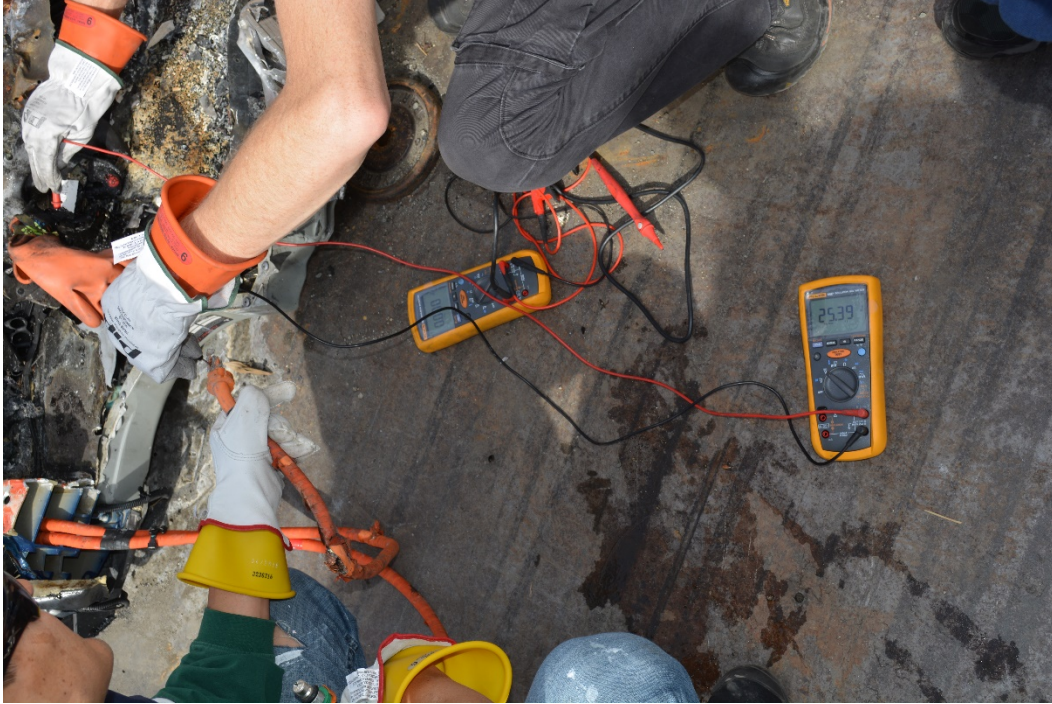
Figure 16. Multimeter display of voltage on the 14 positive bus bar.
