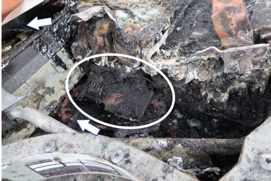
Figure 20. Oval around module 15 BMB. Base plastic of the pyrotechnic fuse remained beneath the BMB. The arrows point from the area of modules 15/16 to module 13 and partially covers a fragment of the pyrotechnic fuse.
