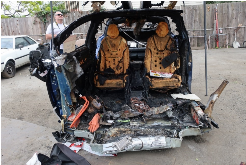
Figure 2. Frontal view of the vehicle, showing crush to front of battery casing at bottom.
