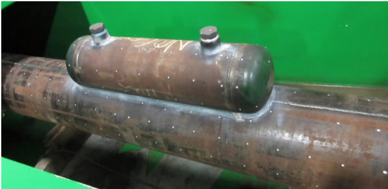
Figure 4-1: Photograph of test vessel enclosed in ADV's test chamber.
