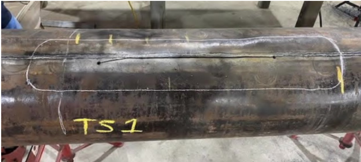
Figure 2-1: Photograph of test vessel with installed crack and drill stops.
