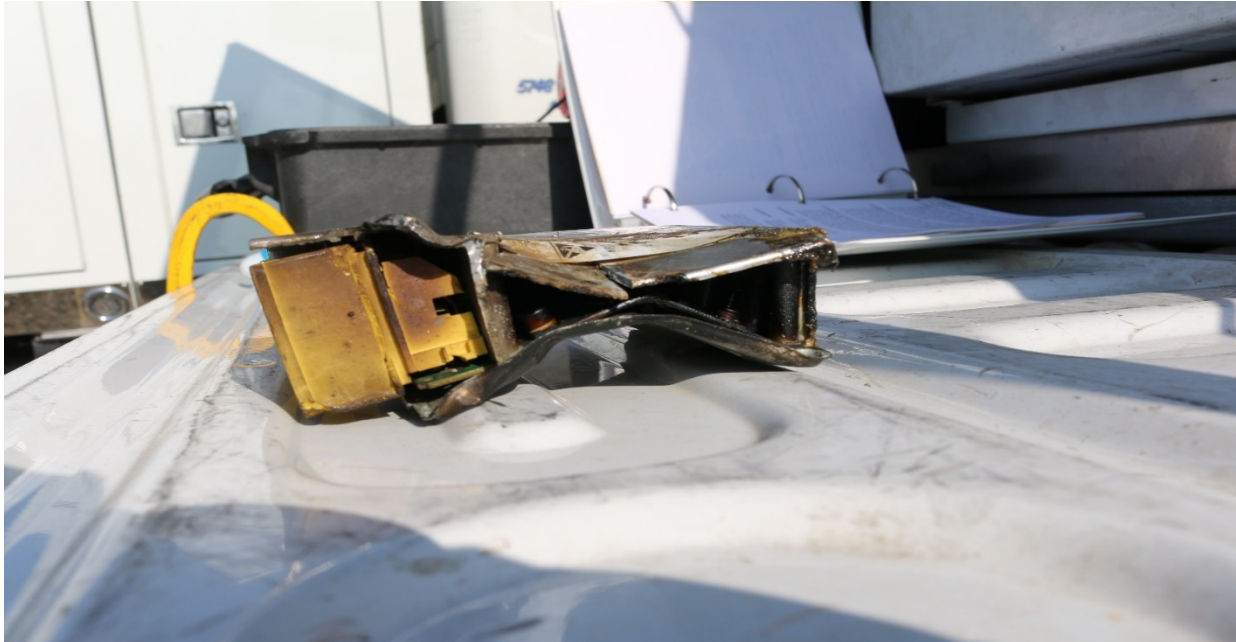
Figure 12: Image of damaged ACM that had been removed from the Dodge Journey. (Source: California Highway Patrol).
