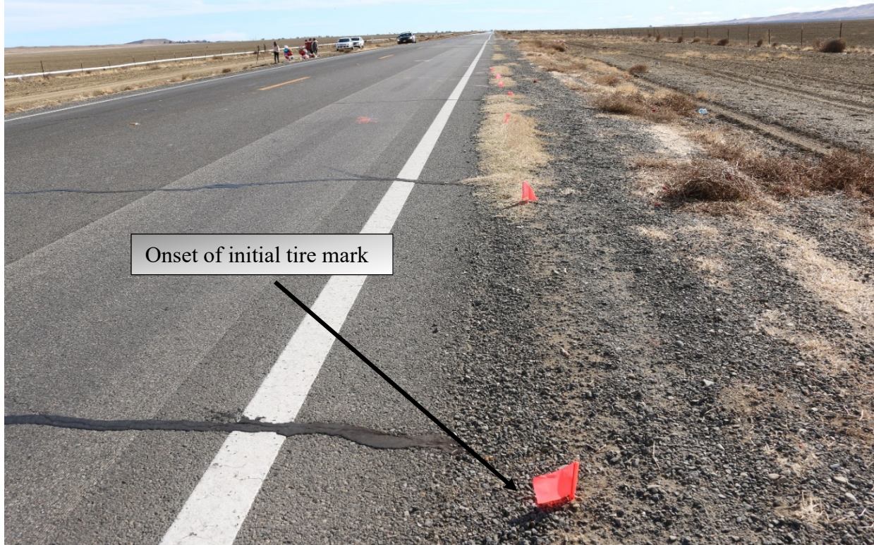
Figure 4: Southbound view of SR-33. Orange flags depict a tire mark deposited by the Dodge on the unimproved dirt/gravel. (Source: California Highway Patrol)
