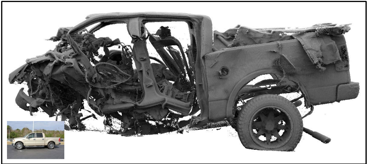
Figure 9: 3D scan image of the Ford pickup truck depicting damage to left side of the vehicle. An inset photo is included in the lower left-hand corner of the figure depicting an undamaged Ford. (Source: California Highway Patrol).
