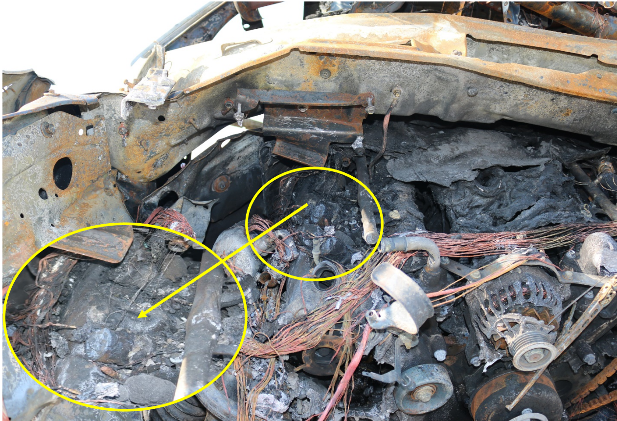
Figure 11: Image of engine compartment of Ford pickup truck. There is a zoomed window focusing on the PCM of the Ford. (Source: California Highway Patrol).
