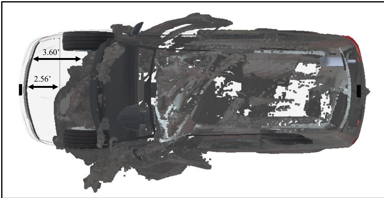
Figure 7: Overhead view of the 3D scan image of Dodge Journey overlaid on an exemplar vehicle. Measurements represent extent of crush damage and are for reference only. (Scan image source: California Highway Patrol).
