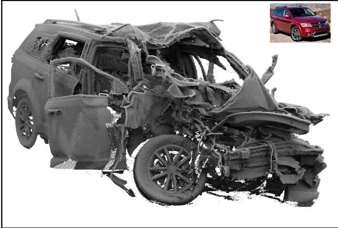
Figure 8: 3D scan image of the Dodge Journey depicting damage to front and right passenger side of the vehicle. An inset photo is included in the upper right-hand corner of the figure depicting an undamaged Dodge Journey. (Source: California Highway Patrol).
