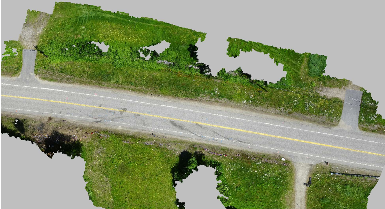
Figure 2: Screen capture of point cloud rendered from daytime aerial photographs provided by NHSP.
