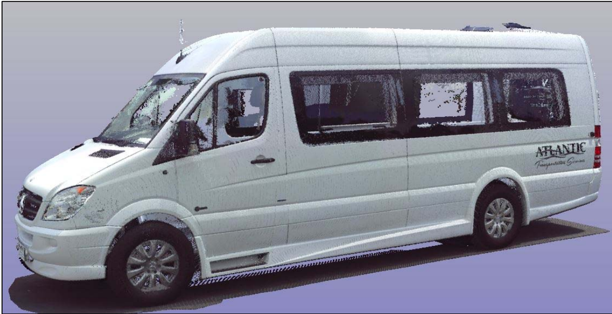
Figure 12: Screen capture of colorized, linked 3D scans depicting the left side of an exemplar Mercedes-Benz Sprinter outfitted for limousine service.
