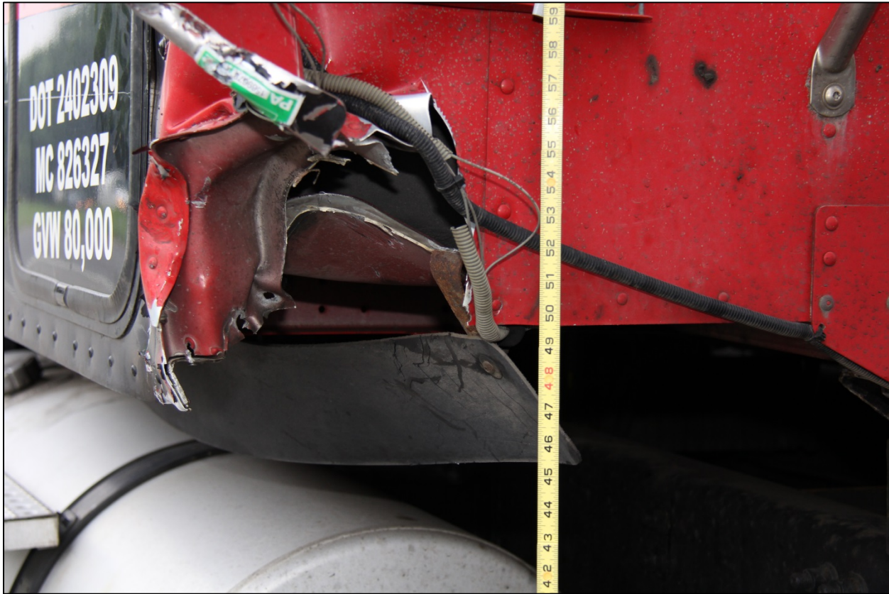
Figure 16: Photograph of Freightliner-Utility combination depicting impact damage on driver's side of vehicle.
