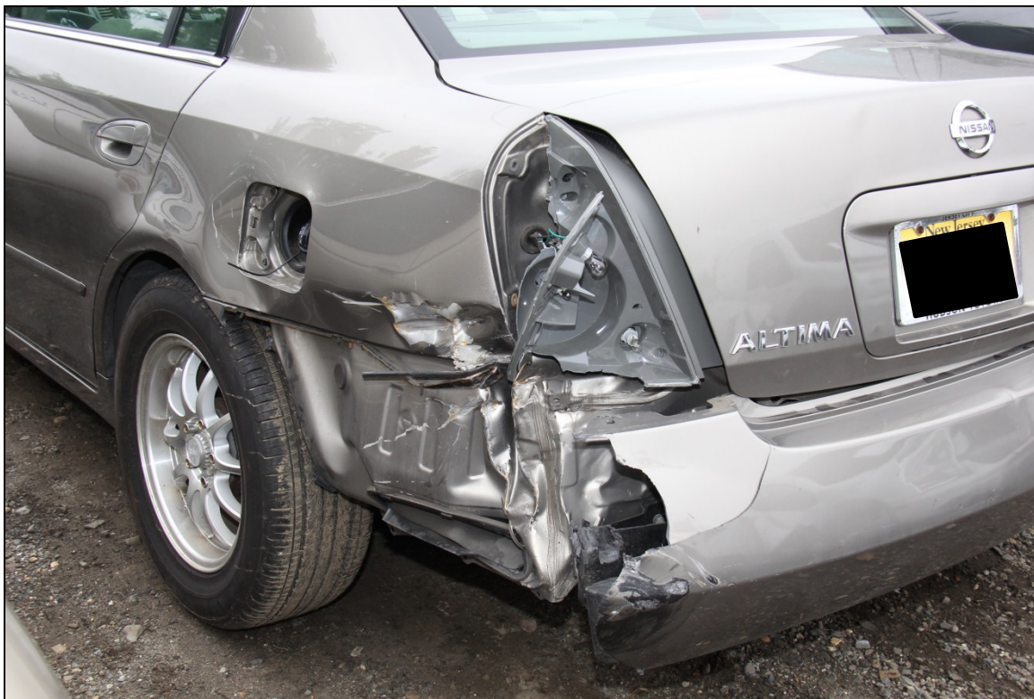
Figure 13: Photograph of Nissan depicting impact damage to the driver's side rear.
