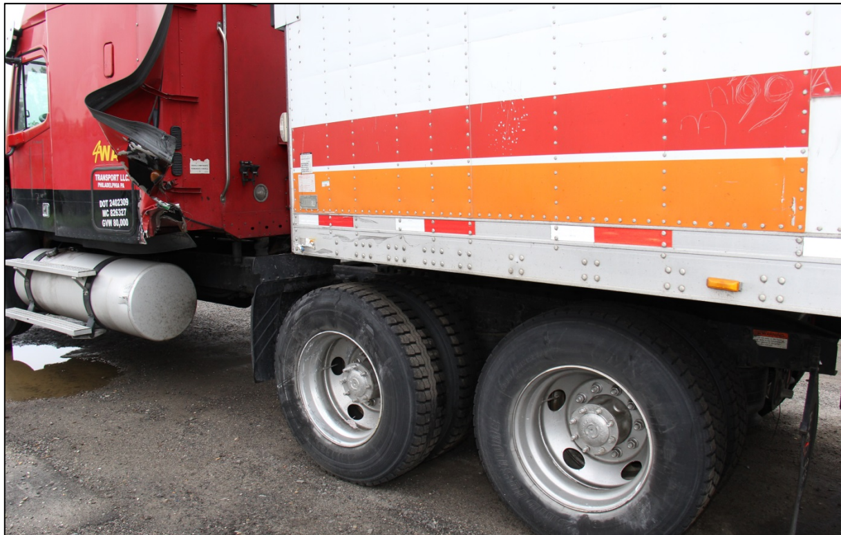
Figure 15: Photograph of driver's side impact damage to Freightliner-Utility combination.
