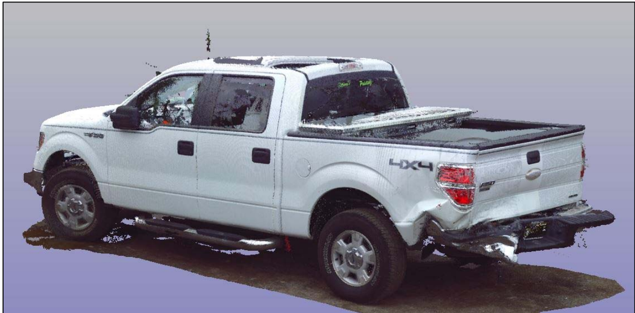
Figure 11: Screen capture of colorized, linked 3D scans depicting the left rear area of damage on the Ford F-150.
