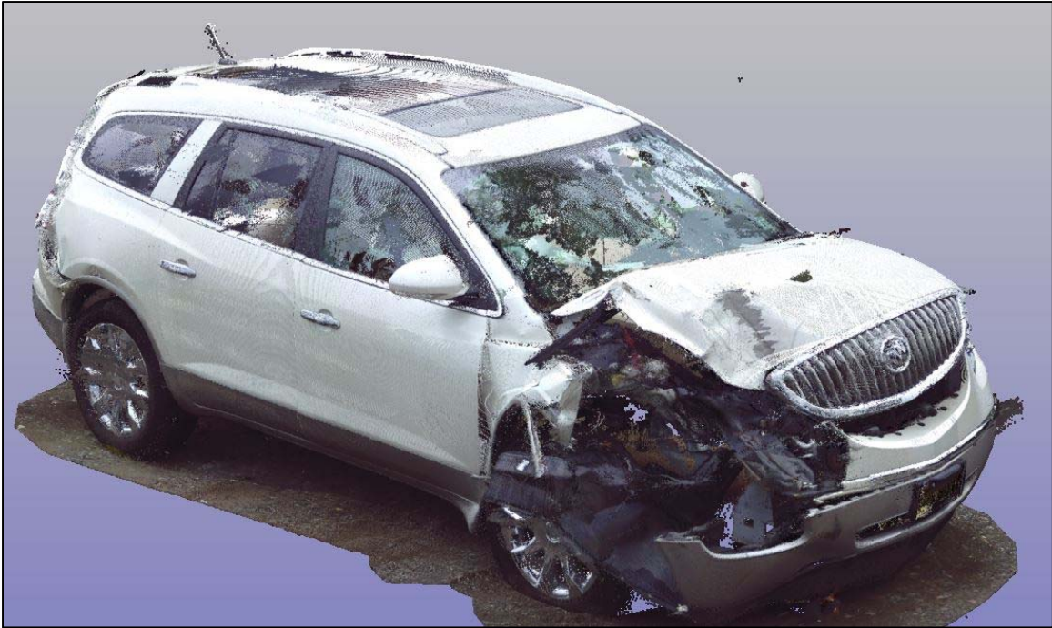
Figure 9: Screen capture of colorized, linked 3D scans depicting the right front area of damage on the Buick Enclave.
