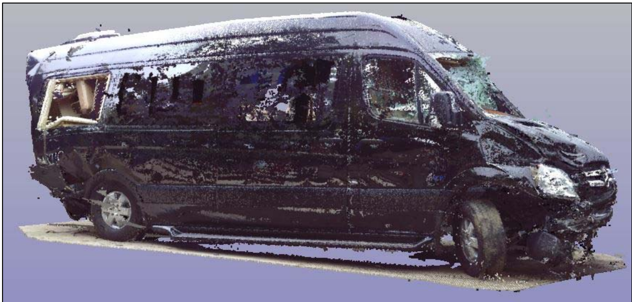
Figure 2: Screen capture of colorized, linked 3D scans of Mercedes-Benz Sprinter from the passenger's side.
