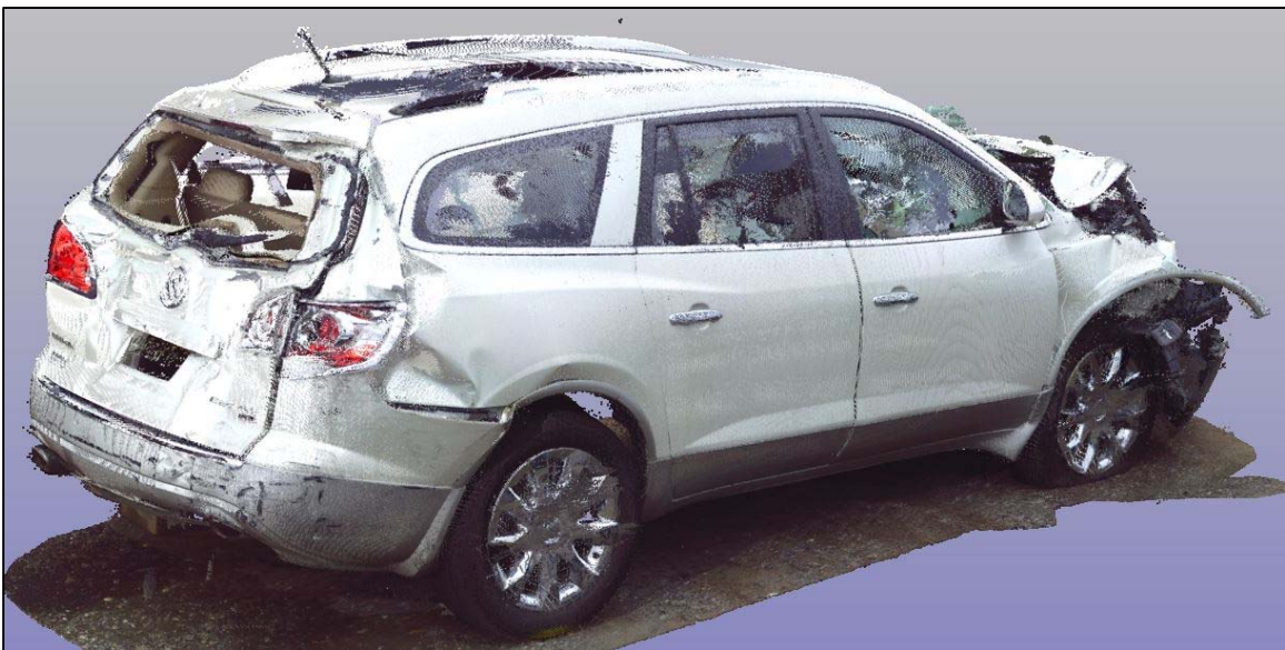
Figure 10: Screen capture of colorized, linked 3D scans depicting the right rear area of damage on the Buick Enclave.
