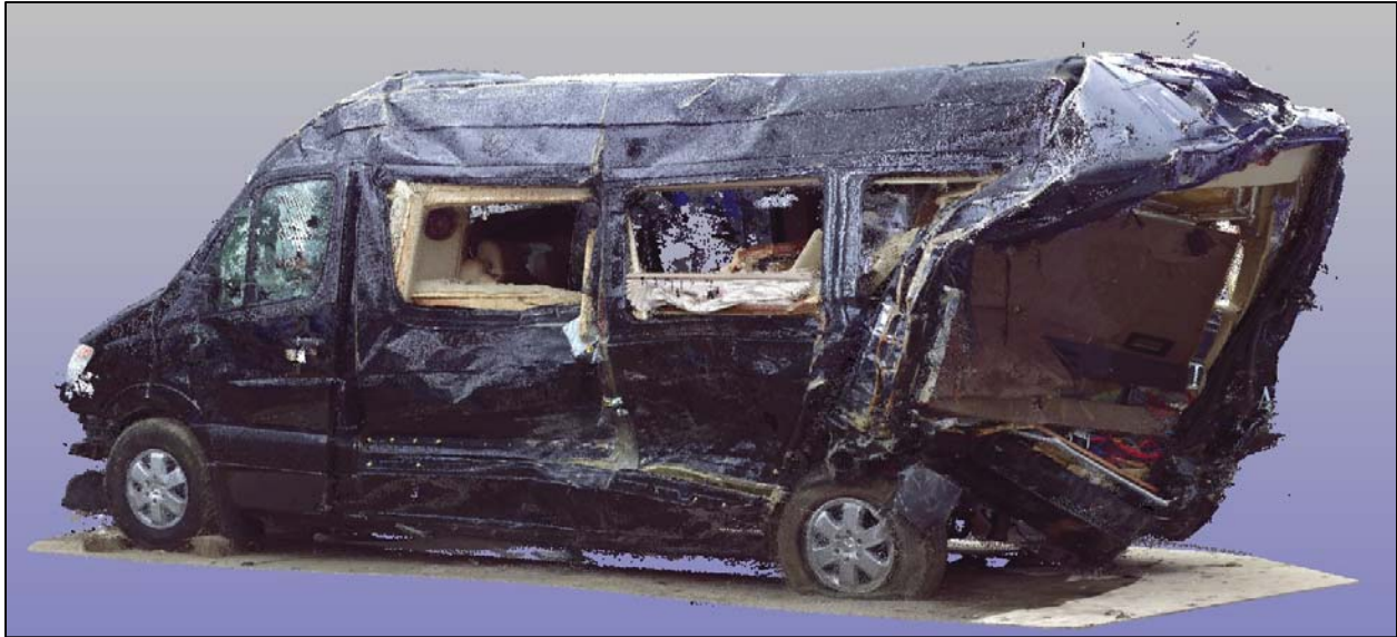
Figure 1: Screen capture of colorized, linked 3D scans of Mercedes-Benz Sprinter from the driver's side.
