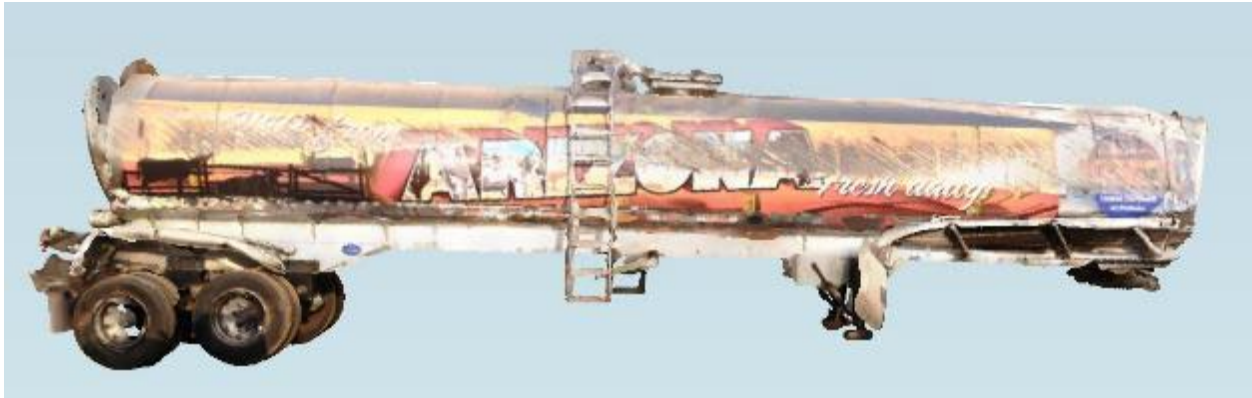
Figure 13: Screen capture depicting the tank-trailer's right side as viewed in the point cloud rendered from the three-dimensional scans through the FARO Scene software.
