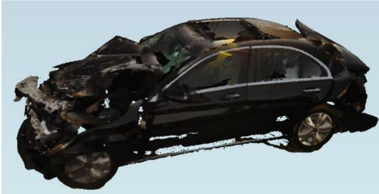
Figure 159: Screen capture depicting the Mercedes left side in the point cloud rendered from the three-dimensional scans through the FARO Scene software.
