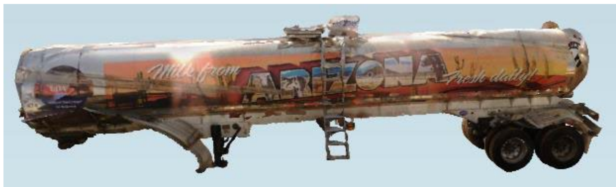
Figure 12: Screen capture depicting the tank-trailer's left side as viewed in the point cloud rendered from the three-dimensional scans through the FARO Scene software.
