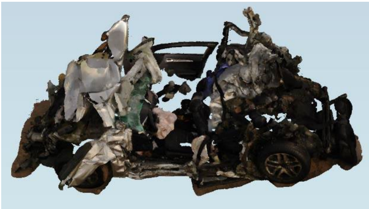
Figure 104: Screen capture depicting the Ford top left side as viewed in the point cloud rendered from the three-dimensional scans through the FARO Scene software.
