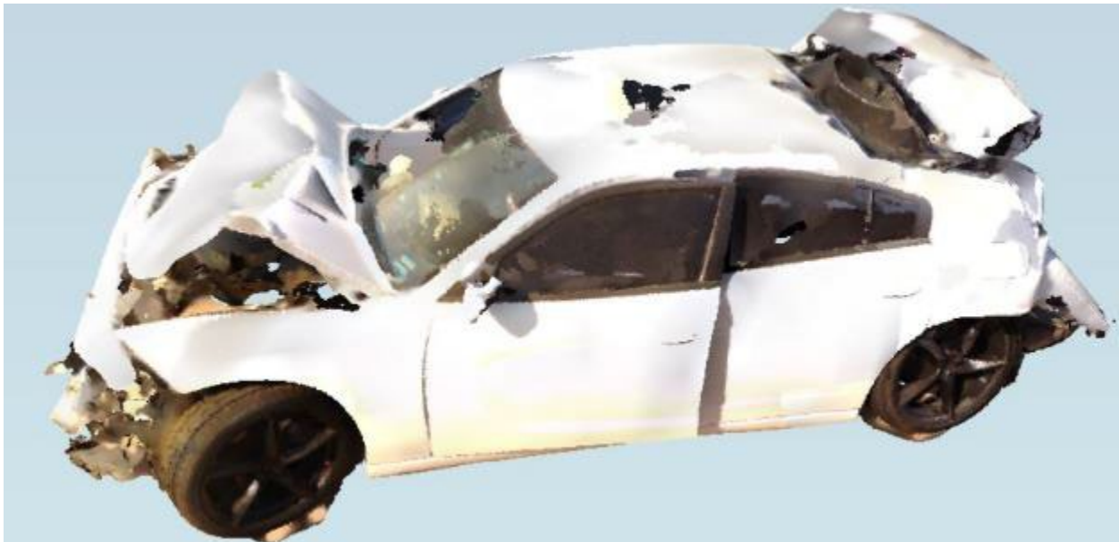
Figure 14: Screen capture depicting the Dodge left side in the point cloud rendered from the three-dimensional scans through the FARO Scene software.
