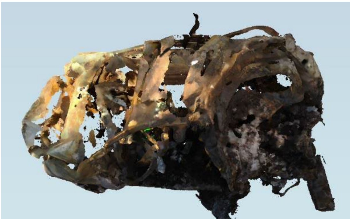
Figure 12: Screen capture depicting the Chevy top left side in the point cloud rendered from the three-dimensional scans through the FARO Scene software.
