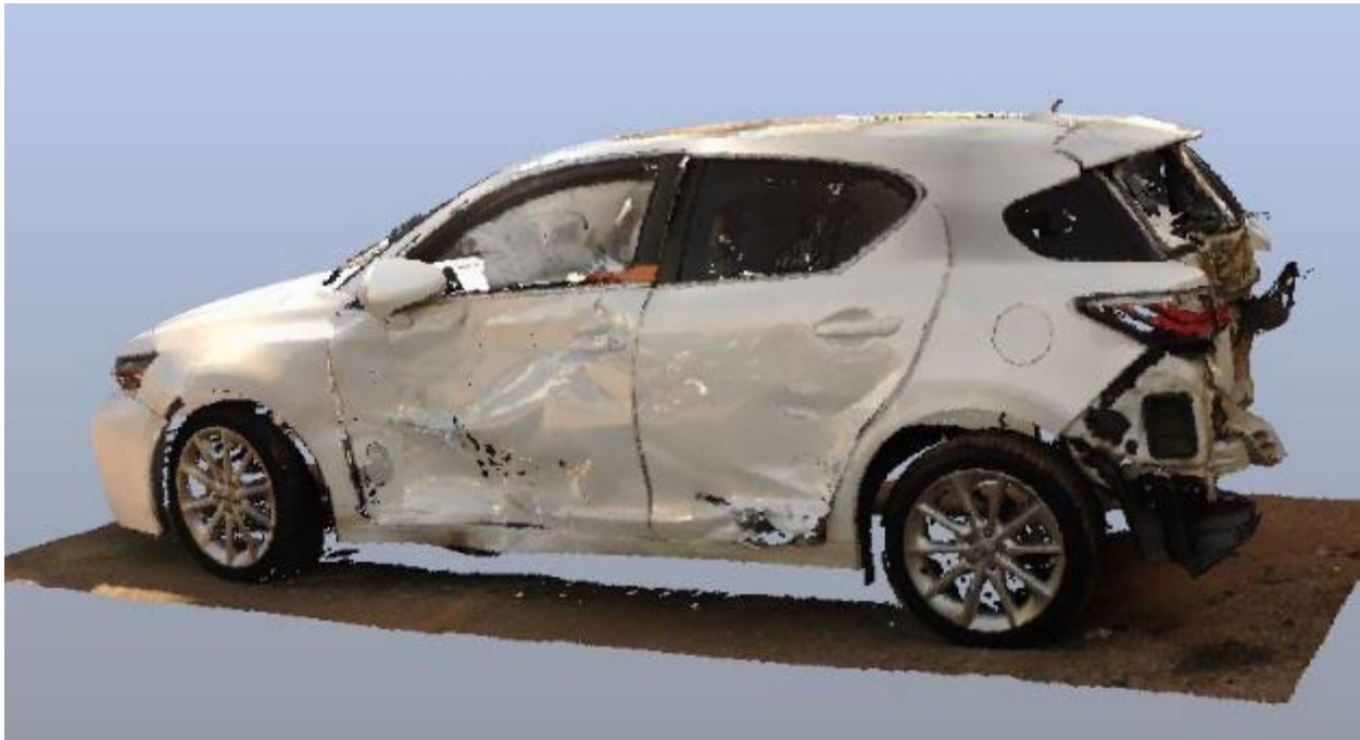
Figure 20: Screen capture depicting the Lexus from the left side as viewed in the point cloud rendered from the three-dimensional scans through the FARO Scene software.
