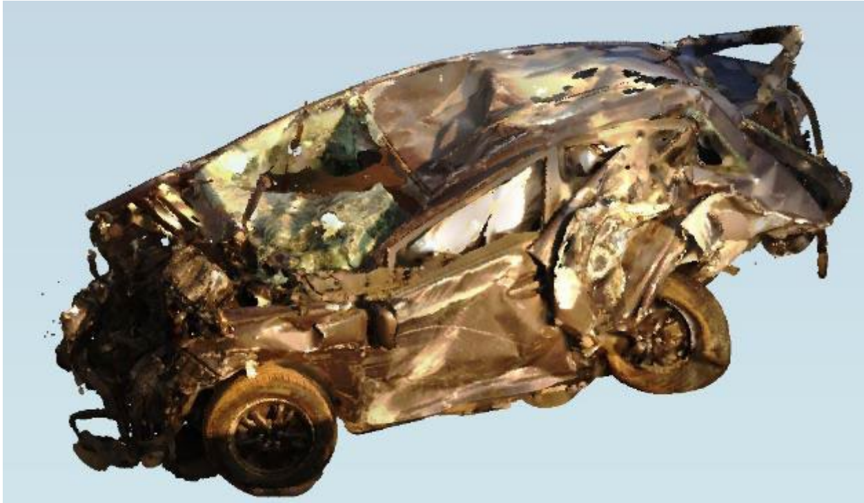
Figure 11: Screen capture depicting the Prius top left side in the point cloud rendered from the three-dimensional scans through the FARO Scene software.
