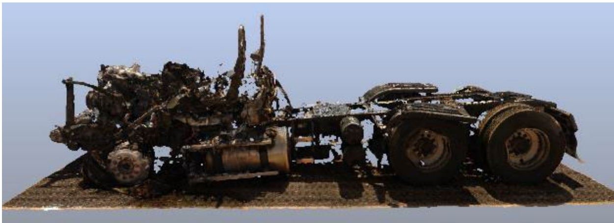
Figure 11: Screen capture depicting the Freightliner left side as viewed in the point cloud rendered from the three-dimensional scans through the FARO Scene software.
