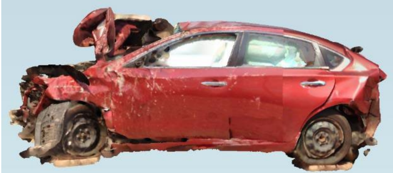
Figure 13: Screen capture depicting the Nissan left side in the point cloud rendered from the three-dimensional scans through the FARO Scene software.
