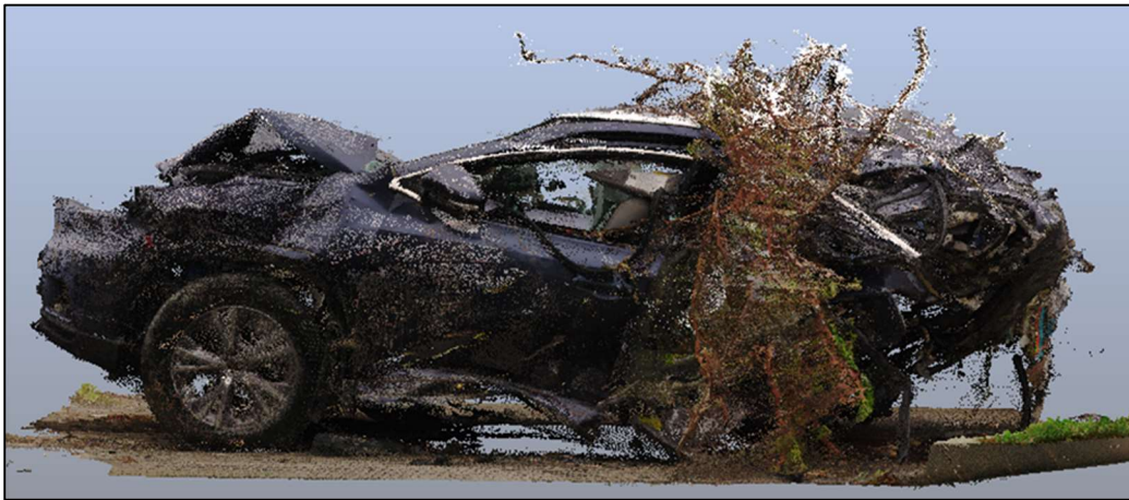
Figure 7: Image depicting the 3D point cloud rendering of the Toyota Highlander as viewed from the driver side. Foliage debris that remained embedded in vehicle damage as a result of the collision were not removed pending inspection by NYSP investigators.
