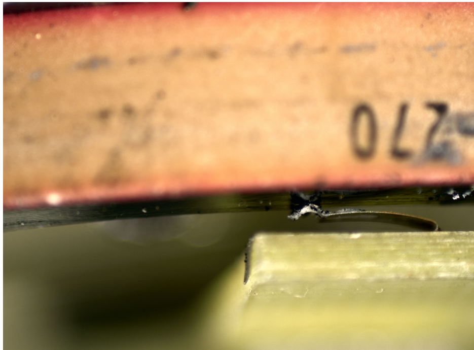
Figure 14 Wiper 2 contact with Potentiometer Number 2
