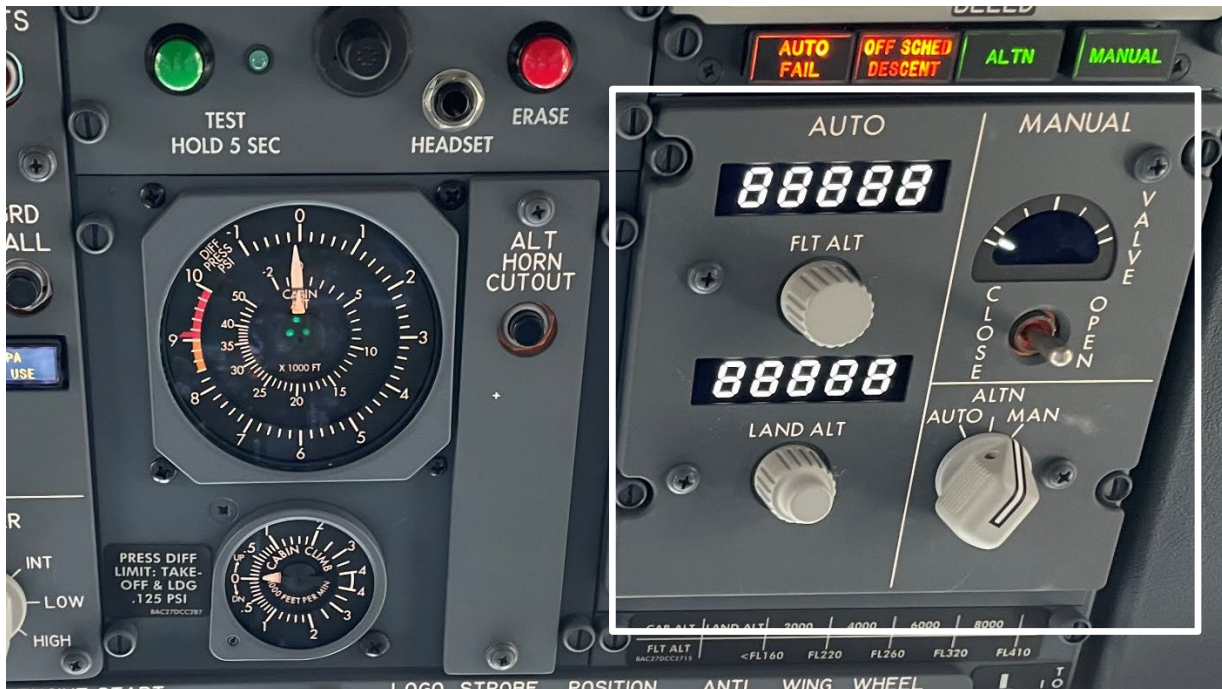
Figure 1. Cabin pressure control switches and indications on the P5 panel. The P5-6 selector panel is outlined by the white square.
